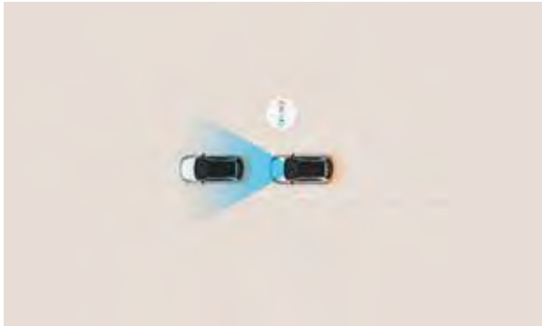
Forward Collision Avoidance (FCA): On detecting the risk of a collision ahead with a vehicle, pedestrian or cyclist, the driver is alerted to the danger, and if necessary, brakes are automatically applied to help prevent a frontal collision.
