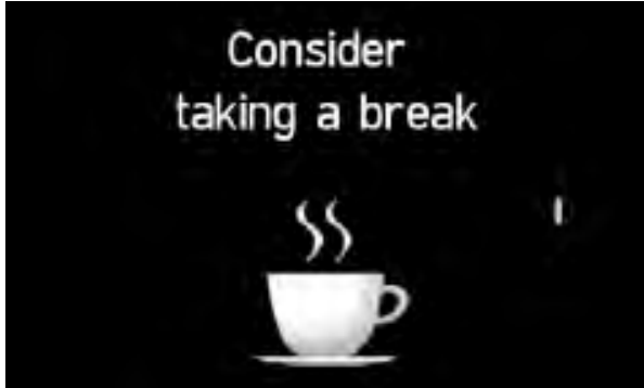
Driver Attention Warning (DAW): When a pattern of fatigue or distraction is identified, the system gets your attention with an alert and pop-up message suggesting a break.
