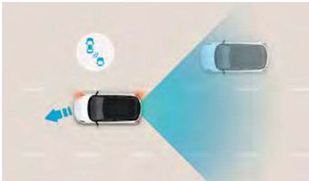
Blind Spot Collision Avoidance Assist (BCA): Radars detect traffic in the vehicle blind spot, warning drivers with an audible alarm when the indicator is used so you can be aware of the traffic around you. It will also take action itself, braking to help avoid a collision.
