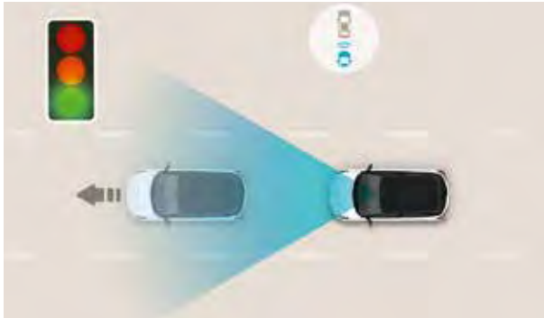
Leading Vehicle Departure Alert (LVDA): This clever feature for city driving alerts the driver when the vehicle in front departs from an idle state, like at a stoplight or in a traffic jam.
