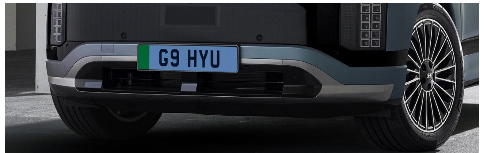
Dual-motion active air flap system for improved aerodynamics and a sleeker appearance. (optional on Calligraphy trim)
