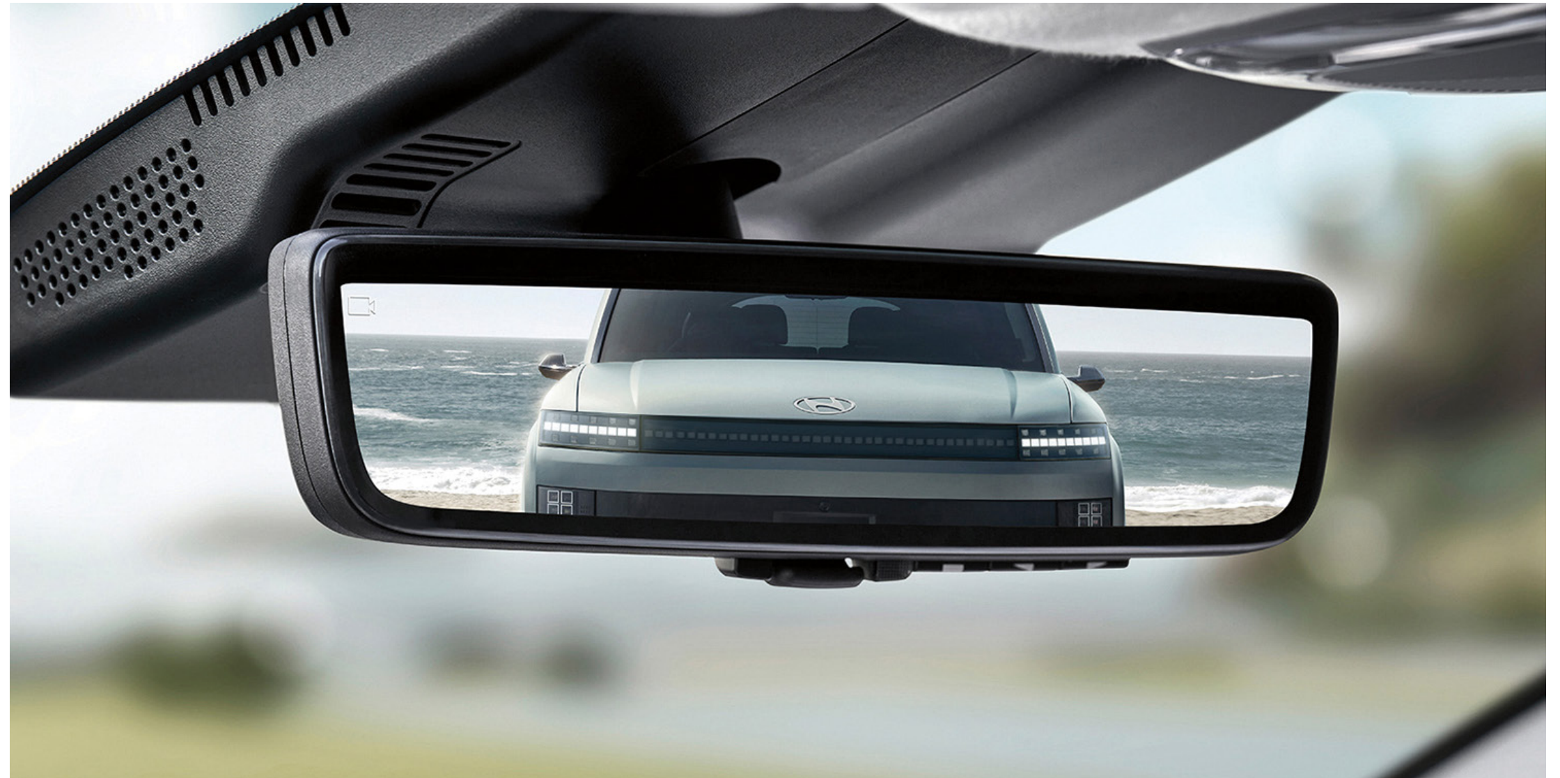
When activated, the Digital Centre Mirror uses a rear-mounted camera to project a real-time video feed onto the mirror for a much wider field of vision.
