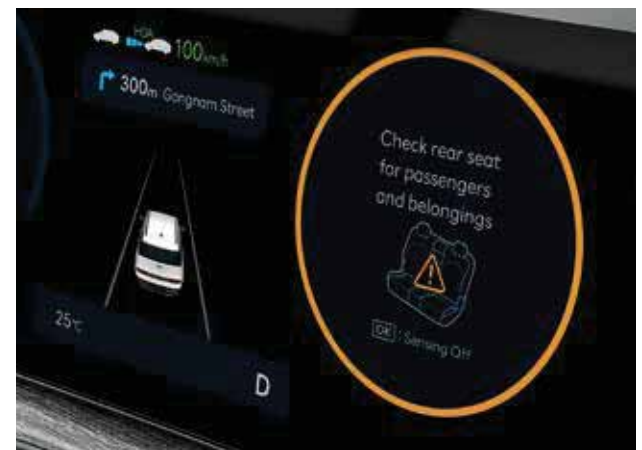
Blind-spot View Monitor (BVM). Rear Occupant Alert (ROA).
