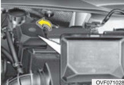
Engine compartment main fuse panel
