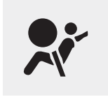
SRS warning light
