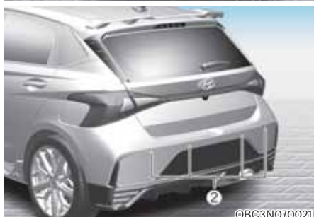
[1] : Front ultrasonic sensors, [2] : Rear ultrasonic sensors
