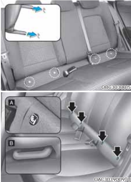
[A] : ISOFIX Anchorage Position Indicator, [B] : ISOFIX Anchorage
