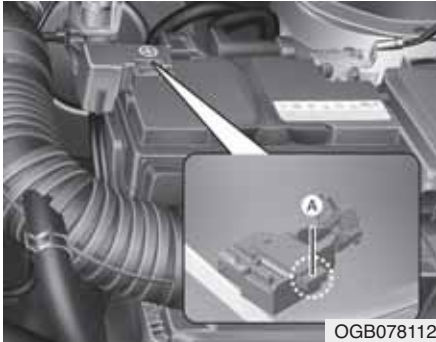
[A] : Battery sensor
