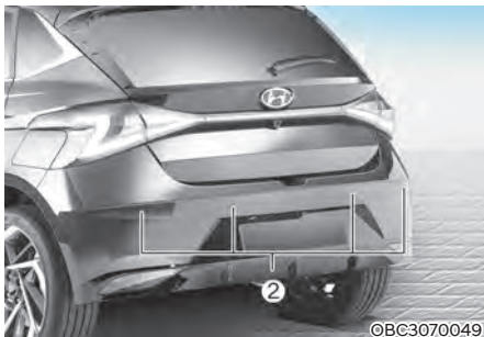
[1] : Front ultrasonic sensors, [2] : Rear ultrasonic sensors
