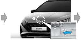
Raise the hood slightly, push the secondary latch up (1) inside of the hood center and lift the hood (2)
