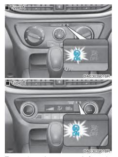
To reactivate the passenger's front airbag:
