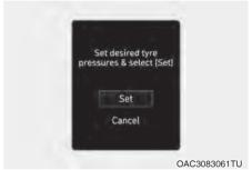
5. Check whether the "Standard tyre pressures saved" message appears on the cluster and the (!) warning light blinks for about 4 seconds.
