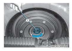
If it is hard to loosen the tyre hold-down wing bolt by hand, you can loosen it easily using the jack handle.
