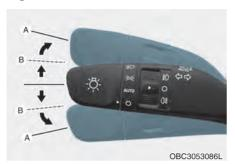
To signal a turn, push down on the lever for a left turn or up for a right turn in position (A). To signal a lane change, move the turn signal lever slightly and hold it in position (B).
