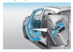
In case of an emergency (battery discharge, etc.) you can manually lock the door using the emergency key.
