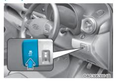
The Electronic Stability Control (ESC) system helps to stabilize the vehicle during cornering manoeuvres.
