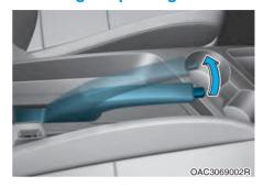
Check the stroke of the parking brake by counting the number of "clicks" heard whilst fully applying it from the released position.
