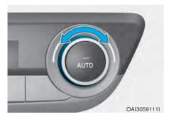
Turn the temperature control knob to set the desired temperature. If the temperature is set to the lowest setting (Lo), the air conditioning system will operate continuously.
