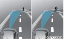
Forward Collision-Avoidance Assist may not detect other vehicle, a pedestrian or a cyclist in front of you whilst driving uphill or downhill adversely affecting the performance of the sensors.
