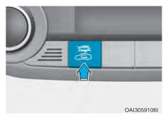
This is used to select the outside (fresh) air position or recirculated air position. To change the air intake control position, push the control button.
