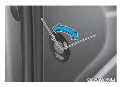
Passenger's front airbag ON/OFF switch (if equipped)
