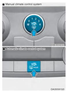
The defroster heats the window to remove frost, fog and thin ice from the interior and exterior of the rear window, whilst engine is running.
