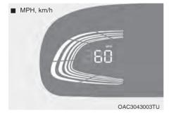
The speedometer indicates the speed of the vehicle and is calibrated in miles per hour (MPH).
