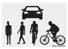
The illustration above shows the image the front view camera will detect as a vehicle, a pedestrian or a cyclist.
