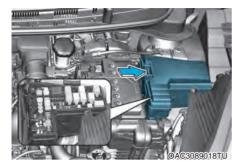
Inside the fuse/relay box covers, you can find the fuse/relay label describing fuse/relay names and ratings.
