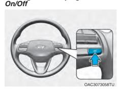
Whenever the vehicle is turned off and on, Lane Keeping Assist will always turn on and the gray (A) indicator light will appear on the cluster.
