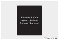
When the front windscreen where the front view camera is located or the sensor is covered with foreign material, such as snow or rain, it can reduce the detecting performance and temporarily limit or disable Forward Collision-Avoidance Assist.
