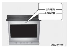
If your vehicle is equipped with a battery marked with LOWER (MIN) and UPPER (MAX) on the side, you should check the electrolyte level. The electrolyte level should be between LOWER (MIN) and UPPER (MAX). When the electrolyte level is low, add distilled (or de-mineralized) water. (Never add sulfuric acids or other electrolyte).
