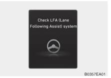
When Lane Following Assist is not working properly, the 'Check LFA (Lane Following Assist) system' warning message will appear on the instrument cluster, for several seconds, and the master warning light will illuminate on the instrument cluster. If this occurs, we recommend that the vehicle be inspected by a HYUNDAI authorised repairer.
