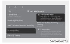
With the engine on, select or deselect User settings > Driver assistance > Diving safety from the settings menu in the instrument cluster or Settings > Vehicle > Driver assistance > Driving safety settings menu in the infotainment system to set whether or not to use each function.
