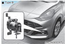
The front fog light can be aimed as the same manner of the head lights aiming. With the front fog lights and battery normal condition, aim the front fog lights. To aim the front fog light up or down, turn the driver clockwise or counterclockwise.
