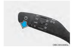
To flash the high beam headlight, pull the lever towards you, then release the lever. The high beams will remain ON as long as you hold the lever towards you.
