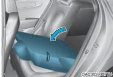
Pull up the seatback lever and fold the seatback toward the front of the vehicle
