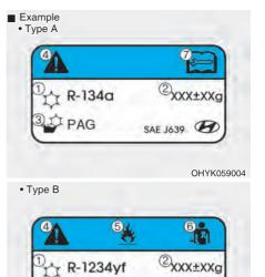
Each symbols and specification on the air conditioning refrigerant label is represented as below:
