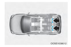
ISOFIX anchorages have been provided in the left and right outboard rear seating positions. Their locations are shown in the illustration. There are no ISOFIX anchorages provided for the centre rear seating position.
