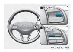
To change the trip mode, toggle the "\land \times \" switch on the steering wheel.
