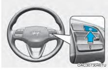
1. Press and hold Driving Assist ((Co)) button at the desired speed. The Speed Limit ((S) LIMIT) indicator will illuminate on the instrument cluster.
