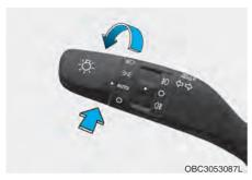
Hight Beam Assist will automatically switch between high beam and low beam depending on the detected brightness from the lamps of oncoming vehicles or vehicles in front.
