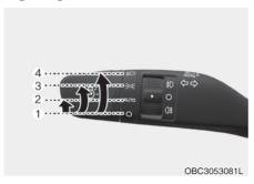
To operate the lights, turn the knob at the end of the control lever to one of the following positions:
