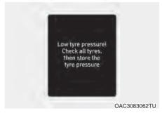
When the Low Tyre Pressure warning light ((!)) illuminates and a warning message appears on the instrument cluster for 10 seconds, one or more of your tyres is significantly under-inflated. If the warning light illuminates, reduce your speed, and also avoid hard cornering and sudden braking. We recommend that your vehicle be inspected by
