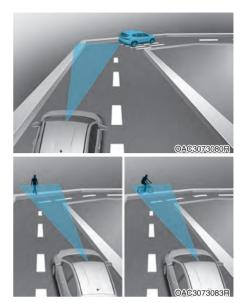
Forward Collision-Avoidance Assist may detect a vehicle, a pedestrian or a cyclist in the next lane or outside the lane when driving on a curved road.
