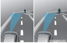
Forward Collision-Avoidance Assist may not detect other vehicle, a pedestrian or a cyclist in front of you on curved roads adversely affecting the performance of the sensors. This may result in no warning or braking assist when necessary.
