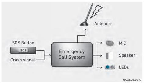
Overview of the 112-based eCall in-vehicle system, its operation and functionalities: refer to this section. The 112-based eCall service is a public service of general interest and is accessible free of charge.
