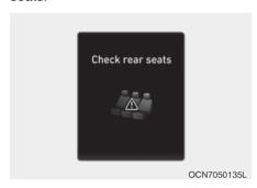
When the driver turns off the engine and opens the driver's door after opening and closing a rear door, a warning message "Check rear seats" appears on the cluster display.
