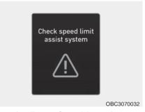
When Intelligent Speed Limit Assist is not working properly, the 'Check Speed Limit system' warning message will appear on the cluster for several seconds, and the master ((A)) warning light and ((C)) warning light will illuminate on the instrument cluster. If this occurs, we recommend that you have the vehicle inspected by a HYUNDAI authorised repairer.
