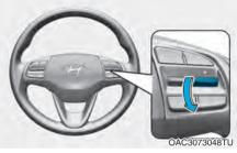
Push the + switch up or - switch down, and release it at the desired speed.
