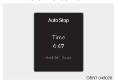
AUTO STOP display shows the elapsed time of engine stop by Idle Stop and Go system.
