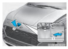
Go to the front of the vehicle, raise the bonnet slightly, push up the secondary hood release lever (1) inside of the bonnet centre and lift the bonnet (2).
