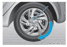
13. Use the wheel lug nut wrench to tighten the lug nuts in the order shown. Double-check each lug nut until they are tight. After changing tyres, we recommend that a HYUN-DAI authorised repairer tighten the lug nuts to their proper torque as soon as possible. The wheel lug nut should be tightened to 11-13 kgf.m (79-94 lbf.ft).
