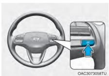
With the engine on, short press the Lane Driving Assist button located on the steering wheel to turn on Lane Following Assist.
