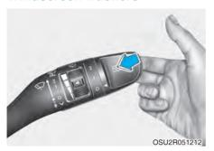
In the OFF (O) position, pull the lever gently toward you to spray washer fluid on the windscreen and to run the wipers 1-3 cycles. The spray and wiper operation will continue until you release the lever. If the washer does not work. vou may need to add washer fluid to the washer fluid reservoir.
