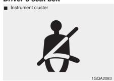
Regardless of the driver's seat belt fastening, the warning light will illuminate for about 6 seconds each time you turn the ignition switch ON. If the driver's seat belt is not fastened, the warning chime will sound for about 6 seconds and the waning light will stay ON until the driver's seat belt is fastened.
