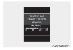
Press and hold the ESC OFF button continuously for more than 3 seconds. The ESC OFF indicator light and/or message "Traction control and ESC disabled" illuminates and a warning chime sounds twice. In this state, both the traction control function of ESC (engine management) and the brake control function of ESC (braking management) are disabled.
