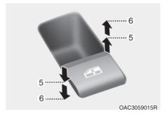
Pressing or pulling up the power window switch momentarily to the second detent position (6) completely lowers orlifts the window even when the switch is released. To stop the window at the desired position while the window is in operation, pull up or press down and release the switch
