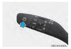
To turn on the high beam headlight, push the lever away from you.
