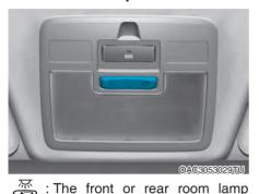
come on when the front or rear doors are opened if the engine is running or not. When doors are unlocked by the remote key or smart key, the front and rear lights come on for about 30 seconds as long as any door is not opened. The front and rear room lamps go out gradually after about 30 seconds if the door is closed. However, if the ignition switch is in the ON position or all doors are locked, the
