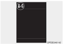
This indicator informs which gear is desired whilst driving to save fuel.
