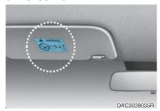
Airbag warning labels are attached to alert the driver and passengers of potential risks of the airbag system. Be sure to read all of the information about the airbags that are installed on your vehicle in this Owner's Manual.
