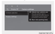
You can change Rear View Monitor Content selection by touching the setup icon (③) on the screen whilst Rear View Monitor is operating, or selecting Settings > Vehicle > Driver assistance > Parking safety > Camera settings from the Settings menu whilst the engine is on.
