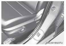
All specifications (sizes and pressures) can be found on a label attached to the left side centre pillar.
