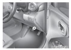
Foot lamp (A): The light turns on when a door is opened and turns off when the door is closed.
