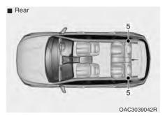
(5) Rear retractor pre-tensioner assembly (if equipped)
