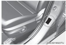
The vehicle certification label attached on the driver's (or front passenger's) side centre pillar gives the vehicle identification number (VIN).
