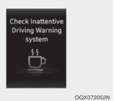
When Driver Attention Warning is not working properly, the 'Check Inattentive Driving Warning system' warning message will appear on the instrument cluster for several seconds, and the master warning light and Driver Attention Warning light ( ) will illuminate on the instrument cluster. If this occurs, we recommend that the vehicle be inspected by a HYUNDAI authorised repairer.
