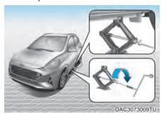
Insert the jack handle into the jack and turn it clockwise, raising the vehicle until the tyre clears the ground. Make sure the vehicle is stable on the jack.
