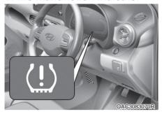
The TPMS malfunction indicator ((!)) illuminates for about 70 seconds when there is a problem with the Tyre Pressure Monitoring System.
