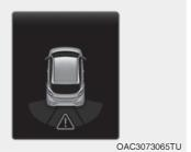
When the Parking Distance Warning is operating, if the function is not working normally or the ultrasonic sensor is blocked, the master warning light (△) appears in the direction of the corresponding sensor. You can check the warning in the Utility view on the cluster.
