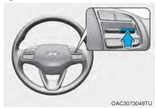
Press the **IID** switch to temporarily pause the set speed limit. The set speed limit will turn off but the Speed Limit (**S**I\_IMIT) indicator will stay on.
