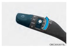
Vehicle with front fog light To turn on the rear fog light:
