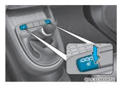
Whilst the engine is running, push either of the switches to warm the driver's seat or front passenger's seat.
