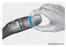
The rear window wiper and washer switch is located at the end of the wiper and washer switch lever.
