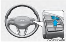
Press the Driving Assist (Co) button to turn Cruise Control off. The Cruise ( CRUISE) indicator will go off.
