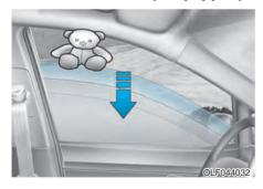
If a window senses any obstacle whilst it is closing automatically, it will stop and lower about 12 in. (30 cm) to allow the object to be cleared. If the window detects the resistance whilst the power window switch is pulled up continuously, the window will stop upward movement then lower about 1 in. (2.5 cm).
