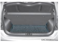
To keep items from shifting in the cargo area, you can use the four holders located in the cargo area to attach the luggage net.
