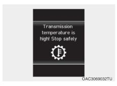
Transmission(clutch) High temperature (first & second warning)
