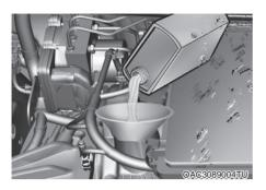
7. If the oil level is near or below the L, add enough oil to bring the level to F. Use a funnel to help prevent oil from being spilled on engine components. Use only the specified engine oil. (Refer to "Recommended lubricants and capacities" in chapter 2.)
