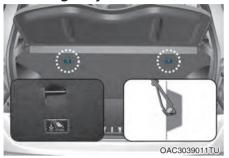
Top-tether anchorages for Child Restraint Systems are located on the rear of the seatback.
