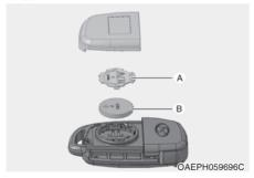
Battery type: CR2032 To replace the battery:
