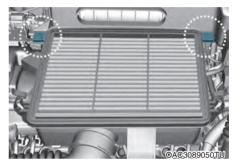
5. The protrusions in the filter should be mounted either on the left or right side of the air cleaner upper side. If incorrectly installed to the bottom side, it may be difficult to assemble.
