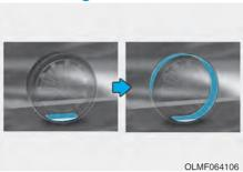
Immediately drive about 4-6 miles (7-10 km or, about 10min) to evenly distribute the sealant in the tyre.
