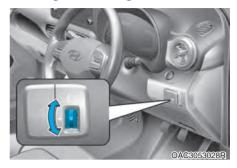
To adjust the headlight beam level according to the number of the passengers and loading weight in the luggage area, turn the beam levelling switch.
