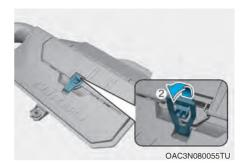
Open the air cleaner filter cover by lifting the lock(2) in the direction of the arrow.
