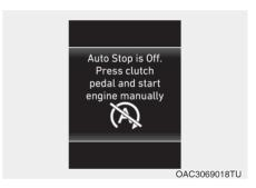
The message, "Auto Stop is Off. Press clutch pedal and start engine manually", appears on the cluster display with a beep sound.
