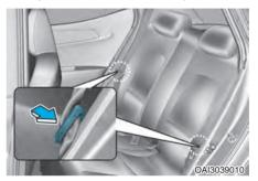
Insert the rear lap/shoulder belt plate into the holder on the side trim. It will prevent the lap/shoulder belt from interfering with the seatback when folding.
