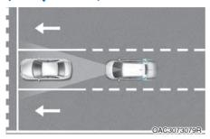
Forward Collision-Avoidance Assist is designed to help detect and monitor the vehicle ahead or help detect a pedestrian or a cyclist in the roadway and warn the driver that a collision is imminent with a warning message and an audible warning, and if necessary, apply emergency braking.
