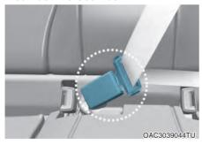
When using the rear centre seat belt, the buckle with the "CENTER" mark must be used
