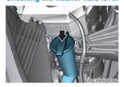
Check the fluid level in the washer fluid reservoir and add fluid if necessary.
