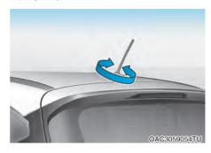
The roof antenna receives DAB (if equipped) and both AM and FM broadcast signals. Rotate the roof antenna in a counterclockwise direction to remove it. Rotate it in a clockwise direction to reinstall it.
