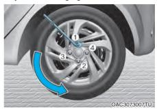
6. Loosen the wheel lug nuts counterclockwise one turn each in the order shown above, but do not remove any lug nuts until the tyre has been raised off of the ground.
