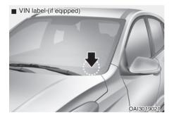
The VIN is also on a plate attached to the top of the dashboard. The number on the plate can easily be seen through the windscreen from outside.
