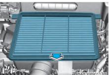
Remove the cleaner cover by opening the clips.
