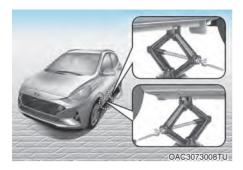
7. Place the jack at the designated jacking position under the frame closest to the tyre you are changing. The jacking positions are plates welded to the frame with two notches. Never jack any other position or part of the vehicle. Doing so may damage the side seal molding or other parts of the vehicle.
