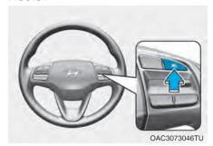
Press the Driving Assist ( $\bigcirc$ n) button to turn Manual Speed Limit Assist off. The Speed Limit ( $\bigcirc$ 1 indicator will go off.
