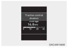
Press the ESC OFF button briefly. The ESC OFF indicator light and/or message "Traction control disabled" will illuminate and a warning chime sounds once. In this state, the traction control function of ESC (engine management) is disabled, but the brake control function of ESC (braking management) still operates.
