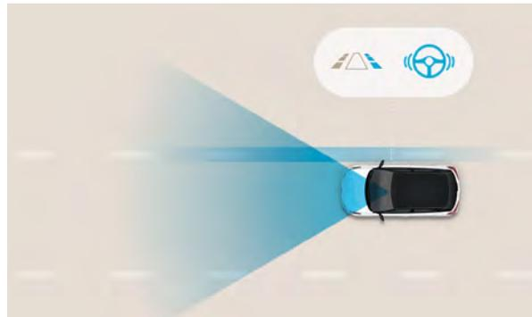
**Highway Driving Assist (HDA):** For additional safety, Highway Driving Assist keeps your vehicle at your pre-set speed and maintains road position in your lane. HDA monitors the distance to the vehicles ahead, reducing speed automatically when the gap closes. When the safe distance is restored, HDA resumes the pre-set cruising speed.
