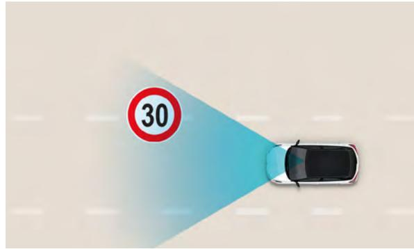
**Intelligent Speed Limit Warning (ISLW):** External cameras and the onboard navigation system combine to monitor road speed limits, keeping you informed via the navigation screen to keep your pace at a safe speed. Available on Premium and Ultimate trims only.
