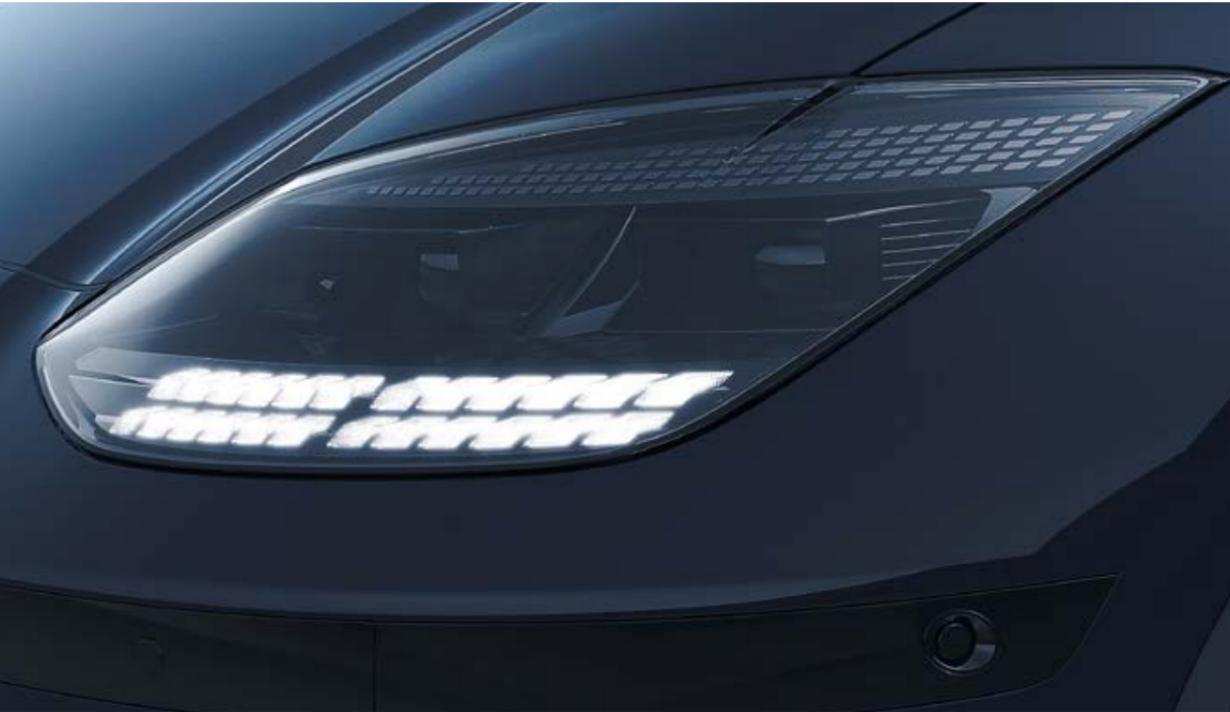
Featuring Matrix beam LED technology and Parametric Pixel Daytime Running Lights, the Intelligent Front-lighting System automatically adapts to road situations, maximizing high beam usage without the risk of dazzling oncoming drivers.
