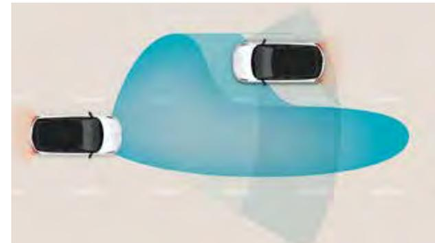
**High Beam Assist (HBA):** Less stress and maximum visibility. HBA not only detects oncoming vehicles but also vehicles in the same lane ahead and switches to low-beam as appropriate.
