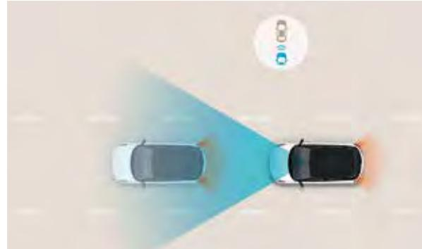
**Forward Collision Avoidance (FCA):** The front view camera and radar sensors warn drivers of imminent collisions with vehicles and objects, applying the brakes when necessary to avoid collisions. The system includes Junction Assist (Turning) across the range.
