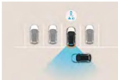
**Rear Cross-traffic Collision Warning (RCCW):** Sensors detect vehicles approaching from both sides when the i30 is in reverse, avoiding collisions in congested or reduced visibility environments such as car parks. Standard on Premium models.
