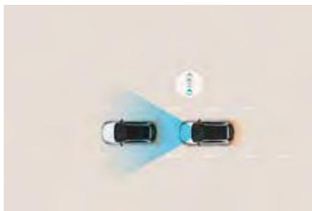
**Front Collision Avoidance (FCA):** The front view camera and radar sensors warn drivers of imminent collisions with vehicles and pedestrians, applying the brakes when necessary to avoid collisions.
