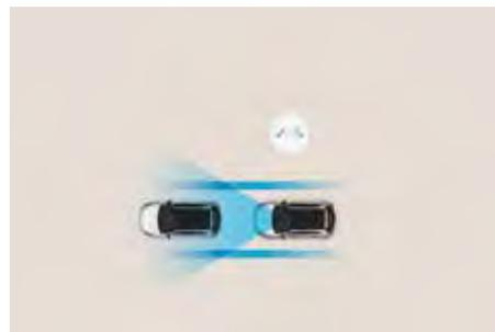
**Lane Follow Assist (LFA):** Smart sensors and the forward-facing camera detect when the car drifts from the centre of the lane, applying steering torque to hold road positioning for safety. The car also estimates the trajectory of the vehicle ahead and adjusts its position accordingly. Standard on Premium models.
