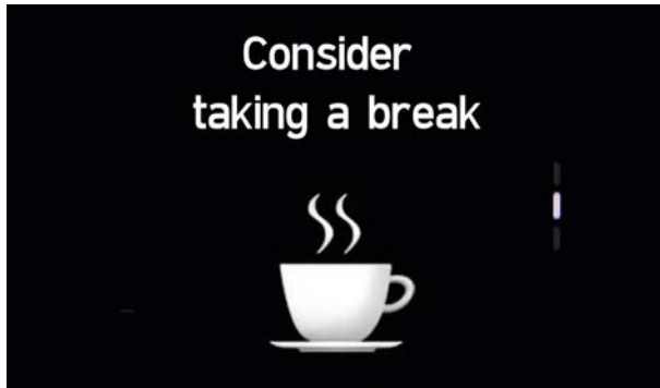
Driver Attention Warning (DAW): When a pattern of fatigue or distraction is identified, the system gets your attention with an alert and pop-up message suggesting a break.
