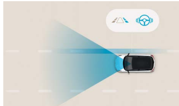
Lane Keeping Assist (LKA): The Lane Keeping Assist (LKA) uses the front multi-function camera to monitor the lines of the road. In case of an unintended lane departure, it warns you and can apply counter steering torque to guide the car back to the lane.
