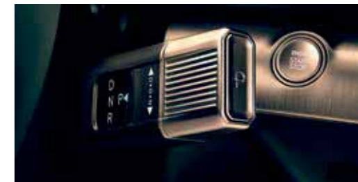
Shift-by-wire via la colonne de direction.
