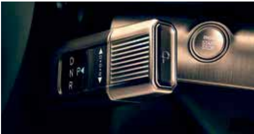
Shift-by-wire via la colonne de direction.
