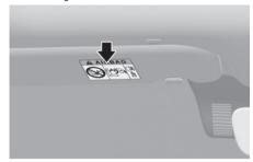
Air bag warning labels are attached to alert the passengers of potential risks of the air bag system.
