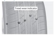
If the tyre is worn evenly, a tread wear indicator will appear as a solid band across the tread. This shows there is less than 1/16 in (1.6 mm.) of tread left on the tyre. Replace the tyre when this happens.
