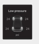
This warning message is displayed if the tyre pressure is low. The corresponding tyre on the vehicle will be illuminated.
