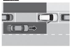
Whilst your vehicle is stopped, and if Safe Exit Warning detects a vehicle approaching the rear corner of your vehicle and a passenger opens a door, Safe Exit Warning may warn you with a warning message and a warning sound to help avoid a collision.
