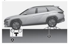
[A] Roll tester (Speedometer)[B] Temporary free roller
