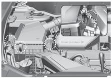
Loosen the air cleaner cover attaching clips and open the cover.
