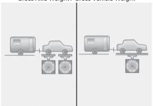
The tongue load is an important weight to measure because it affects the total Gross Vehicle Weight (GVW) of your vehicle. The trailer tongue should weigh a maximum of 10% of the total loaded trailer weight, within the limits of the maximum trailer tongue load permissible.
