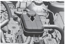
Check the condition and connections of all cooling system hoses and heater hoses. Replace any swollen or deteriorated hoses.
