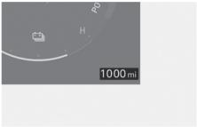
The odometer indicates the total distance that the vehicle has been driven and is used to determine when periodic maintenance is required.
