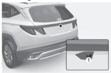
(1) Wide-rear view camera Refer to the picture above for the detailed location of the detecting sensor.
