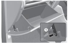
1. Open the glove box and remove the support rod (1).
