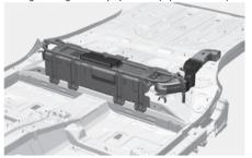
High voltage battery system \*2 (Plug-in hybrid vehicle)
