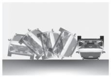
Front air bags may not inflate in rollover accidents because front air bag deployment would not provide additional occupant protection.
