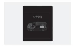
The engine charges the high voltage battery according to the vehicle and surrounding conditions.
