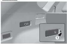
Pull the rear seatback folding switch (1) located on both sides of the cargo area.
