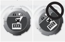
1. Check if the coolant cap label is straight In front.
