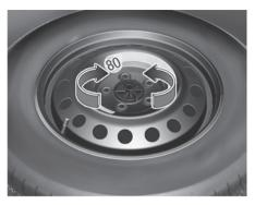
Turn the winged hold down bolt counterclockwise to remove the spare tyre.
