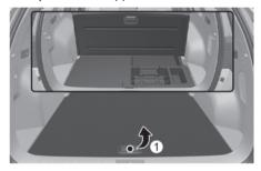
3. Open the emergency cable cover located in the cargo tray with a small blade tool (e.g. screwdriver or similar) (2) and pull the emergency cable.
