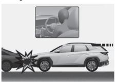
In certain low-speed collisions the air bags may not deploy. The air bags are designed not to deploy in such cases because they may not provide benefits beyond the protection of the seat belts.
