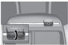
Press the DRIVE/TERRAIN button to change from normal driving mode to multi terrain mode. You can select SNOW, MUD, and SAND modes with the MODE switch within 4 seconds. If you press the DRIVE/TERRAIN button again, it changes to drive mode.
