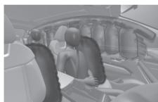
Your vehicle is equipped with a side air bag in each front row seat. Additionally, a front centre side air bag is provided in the inboard side of the driver seatback. The purpose of the air bag is to provide the vehicle's additional protection than that offered by the seat belt alone.
