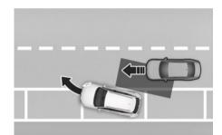
When you are driving forward out of a parking space, if Blind-Spot Collision-Avoidance Assist judges that there is a collision risk with an approaching vehicle in the blind spot, it can help avoid collision by applying the brake.
