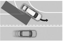
Blind-Spot Collision-Avoidance Assist may not operate properly when driving on a slope. The function may not detect the vehicle in the next lane or may incorrectly detect the ground or structure. Always pay attention to road and driving conditions whilst driving.
