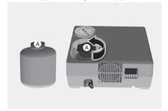
3. Connect the sealant bottle (2) and compressor (6).
