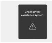
When Forward Collision-Avoidance Assist is not working properly, the 'Check driver assistance system' warning message will appear, and the (△) and (♣) warning lights will illuminate on the cluster. We recommend that your vehicle be inspected by a HYUNDAI authorised repairer.
