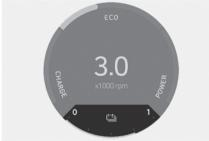
The SOC gauge indicates the remaining hybrid battery power.
