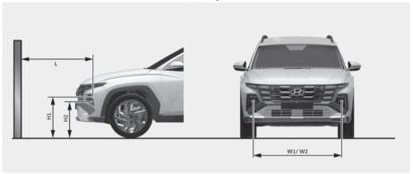
H1: Height between the head light bulb centre and ground (Low beam)
