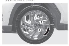
13.Use the wheel lug nut wrench to tighten the lug nuts in the order shown. Double-check each lug nut until they are tight. After changing tyres, we recommend that a HYUNDAI authorised repairer tighten the lug nuts to their proper torque as soon as possible. The wheel lug nut should be tightened to 79~94 lbf·ft (11~13 kgf·m).
