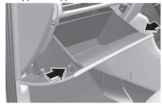
Push in both sides of the glove box as shown. This will ensure that the glove box stopper pins will get released from its holding location allowing the glove box to hang.
