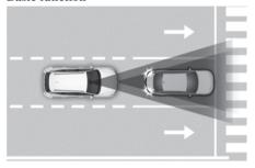
Forward Collision-Avoidance Assist is designed to help detect and monitor the vehicle ahead or help detect a powered two-wheeler, pedestrian or cyclist in the roadway and warn the driver that a collision is imminent with a warning message and warning and apply emergency braking.
