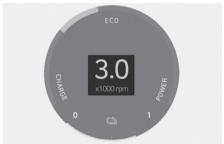
The tachometer indicates the approximate number of engine revolutions per minute (RPM).
