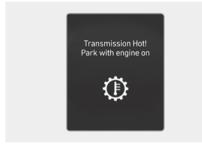
Repeated sudden acceleration and quick start may overheat the transmission. If the transmission is overheated, the self protection mode alarms the driver with an audible sound warning message.
