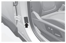
All specifications (sizes and pressures) can be found on a label attached to the driver's side centre pillar.
