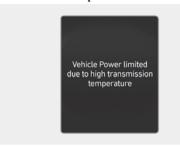
If you continue to drive with overheated transmission, the above warning message appears and self-protection mode restricts the power output of the vehicle
