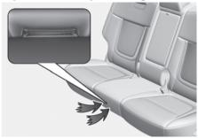
The hybrid battery cooling duct is located in the middle of the rear seats. The cooling duct cools down the hybrid battery. When the hybrid battery cooling duct is blocked, the hybrid battery may be overheated.
