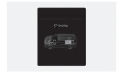
The engine is simultaneously used to drive the vehicle and to charge up the high voltage battery.
