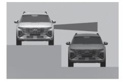
Blind-Spot Collision-Avoidance Assist may not operate properly when driving where the heights of the lanes are different. The function may not detect the vehicle on a road with different lane heights (underpass joining section, grade separated intersections, etc.). Always pay attention to road and
