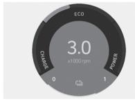
The power gauge indicates whether the current driving condition is fuel efficient or not.
