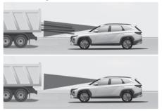
If the vehicle in front of you has cargo that extends rearward from the cab, or when the vehicle in front of you has higher ground clearance, additional special attention is required. Forward Collision-Avoidance Assist may not be able to detect the cargo extending from the vehicle. In these instances, you must maintain a safe braking distance from the rearmost object, and if necessary, steer the vehicle and depress the brake pedal to reduce your driving speed in order to maintain distance.
