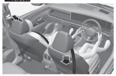
Your vehicle is equipped with driver's and front passenger's and rear passengers Pre-tensioner Seat Belts (Retractor Pre-tensioner). The purpose of the pre-tensioner is to make sure the seat belts fit tightly against the occupant's body in certain frontal or side collision(s). The pre-tensioner seat belts may be activated in crashes where the frontal or side collision(s) is severe enough, together with the air bags.
