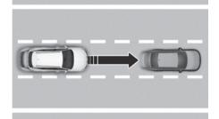
Highway Driving Assist is helps maintain a set distance and speed from the vehicle ahead whilst driving on a highway main section and helps centre the vehicle in the lane.
