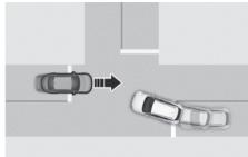
Junction Turning function can help avoid a collision with an oncoming vehicle in an adjacent lane when turning right (right-hand drive) at a crossroad with the turn signal on by applying emergency braking.
