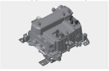
High voltage battery system \*2 (Hybrid vehicle)
