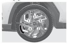
6. Loosen the wheel lug nuts counterclockwise one turn each in the order shown above, but do not remove any wheel lug nuts until the tyre has been raised off of the ground.
