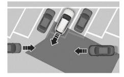
Rear Cross-Traffic Collision-Avoidance Assist may be limited when backing up diagonally, and may not detect the vehicle approaching from the left or right. If this occurs, the function may not warn the driver or control the brakes when necessary.
