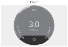
This gauge indicates the remaining hybrid battery power. If the SOC is near the L (Low) level, the vehicle automatically operates the engine to charge the battery.
