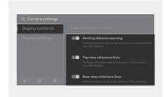
You can change Surround View Monitor Display contents by touching the setup icon (\*) on the screen whilst Surround View Monitor is operating, or selecting Driver assistance > Parking safety > Camera settings from the Settings menu in the infotainment system whilst the engine is on.
