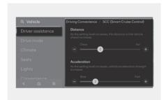
With the vehicle on, select Settings > Vehicle > Driver assistance > Driving convenience > SCC (Smart Cruise Control) from the settings menu in the infotainment system to change Distance, Acceleration, Response speed manually.
