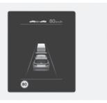
Manual Speed Limit Assist or Smart Cruise Control assists the vehicle to adjust its speed according to the speed limit. When the cruising speed is set as same as the speed limit, the vehicle automatically adjusts its speed if the speed limit changes. The function operates on the road which has a speed limit of 44 mph (70 km/h) or higher. When the function is active, the cruising speed on the instrument cluster appears in green.
