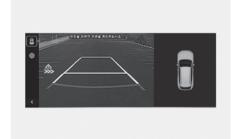
To warn the driver of an approaching vehicle from the rear left/right side of your vehicle, the warning light on the outside rearview mirror blinks and a warning message appears on the instrument cluster. At the same time, an audible warning sounds. A warning also appears on the infotainment system.
