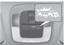
Insert the key or a similar rigid device into the passenger's front air bag ON/OFF switch and turn it to the OFF position. The passenger air bag OFF indicator (巻) will illuminate and stay on until the passenger's front air bag is reactivated.
