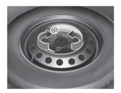
Turn the winged hold down bolt counterclockwise to remove the spare tyre.
