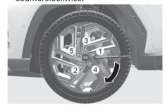
13. Use the wheel lug nut wrench to tighten the lug nuts in the order shown. Double-check each lug nut until they are tight. After changing tyres, we recommend that a HYUNDAI authorised repairer tighten the lug nuts to their proper torque as soon as possible. The wheel lug nut should be tightened to 11-13 kgf·m (79-94 lbf·ft).
