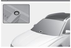
This vehicle is equipped with a solar radiation sensor located on the upper portion of the dashboard. With the air conditioning set to AUTO, the sensor will detect the solar radiation and adjust the indoor temperature automatically. Avoid placing any object on the solar radiation sensor for indoor temperature control.
