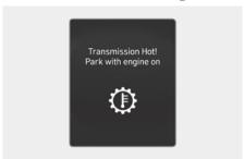
If you continue to drive with an overheated transmission, the above warning message appears, and the self-protection mode disables the clutch.
