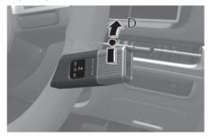
This is the normal forward driving position. The transmission automatically shifts to the optimal gear ratio, providing better fuel efficiency and a smoother ride.
