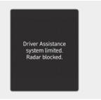
When the rear bumper around the rear corner radar or sensor is covered with foreign material, such as snow or rain, or installing a trailer or carrier, it can reduce the detecting performance and temporarily limit or disable Safe Exit Warning.
