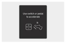
In traffic, your vehicle will stop if the vehicle ahead of you stops. Also, if the vehicle ahead of you starts moving, your vehicle will start as well. In addition, after the vehicle has stopped and a certain time have passed, the 'Use switch or pedal to accelerate' message will appear on the instrument cluster. Depress the accelerator pedal or operate the + switch, - switch or II'2 switch to start driving.
