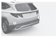
(1) Rear corner radar Refer to the picture above for the detailed location of the detecting sensors.
