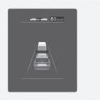
If you want to speed up temporarily without altering the set speed whilst Smart Cruise Control is operating, depress the accelerator pedal. whilst the accelerator pedal is depressed, the set speed, distance level and target distance will blink on the cluster.
