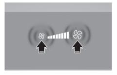
The fan speed can be set as desired by pressing the fan speed control button. More air is delivered with higher fan speeds.
