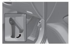
Go to the front of the vehicle, raise the bonnet slightly, push up the secondary bonnet release lever (1) inside of the bonnet centre and lift the bonnet (2).
