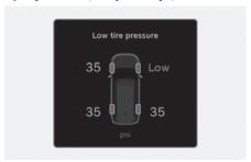
The tyre pressure of each tyre appears. For more information, refer to "Tyre pressure monitoring system (TPMS)" section in chapter 8.
