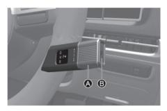
[A] Rotary gear shift dial[B] P button
