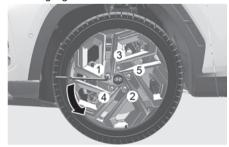
6. Loosen the wheel lug nuts counterclockwise one turn each in the order shown above, but do not remove any wheel lug nuts until the tyre has been raised off of the ground.
