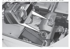
2. Pull down the lever to the UNLOCK (2) position.
