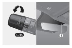
The position light and headlight are turned ON or OFF automatically depending on the amount of daylight as measured by the ambient light sensor (1) in front of the instrument panel.
