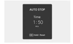
AUTO STOP display shows the elapsed time of engine stop by Idle Stop and Go system.
