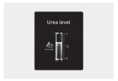
This mode displays the approximate amount of remaining urea solution inside the urea solution tank.
