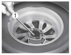
If it is hard to loosen the tyre hold down wing bolt by hand, you can loosen it easily using the jack handle.
