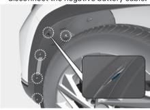
2. Remove wheel guard clips (under the front bumper: 6 pieces).
