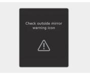
When the outside rearview mirror warning light is not working properly, the **Check outside mirror warning icon** warning message will appear on the instrument cluster for several seconds, and the master (A) warning light will appear on the instrument cluster. If this occurs, we recommend that your vehicle be inspected by a HYUNDAI authorised repairer.
