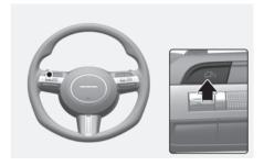
To turn Smart Cruise Control off, press the Driving Assist ( $\bigcap$ ) button.
