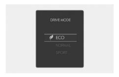
The mode changes, as the following, whenever the DRIVE MODE button is pressed up or down.
