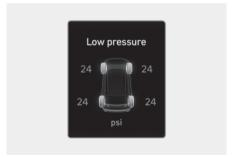
This warning message is displayed if the tyre pressure is low. The corresponding tyre on the vehicle will be illuminated.
