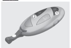
Press and hold the door lock button (1) for more than 3 seconds and the front windows move up after the doors are locked. Window movement stops when you release the door lock button.  Press and hold the door unlock button (2) for more than 3 seconds and the front windows move down after the doors are unlocked. Window movement stops when you release the door unlock button.
