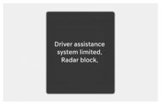
When the front windscreen where the front view camera is located, front radar cover, bumper or sensor is covered with foreign material, such as snow or rain, it can reduce the detecting performance and temporarily limit or disable Forward Collision-Avoidance Assist.
