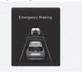
To warn the driver that emergency braking will be assisted, the 'Emergency Braking' warning message will appear on the cluster, an audible warning will sound and the steering wheel will vibrate (if equipped).
