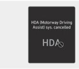
If the driver still does not have their hands on the steering wheel after the hands-off warning, "HDA(Motorway Driving Assist) sys. cancelled" warning message will appear and Highway Driving Assist and Lane Change Assist will be automatically cancelled.
