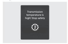
Repeated stop-and-go launches on steep grades, sudden take off or acceleration, or other harsh driving conditions may increase the clutch and transmission temperature.
