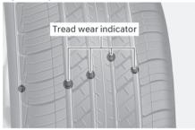
If the tyre is worn evenly, a tread wear indicator will appear as a solid band across the tread. This shows there is less than 1/16 in. (1.6 mm) of tread left on the tyre. Replace the tyre when this happens.
