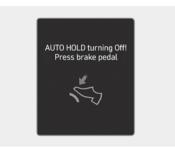
When the conversion from Auto Hold to EPB is not working properly a warning will sound and a message will appear.
