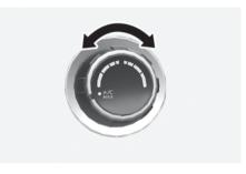
The temperature increases by turning the knob to the right. The temperature decreases by turning the knob to the left.
