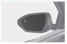
Your vehicle is equipped with both left-hand and right-hand outside rearview mirrors. The mirrors can be adjusted with the mirror adjustment control switch. Adjust the outside rearview mirrors to your desired position before driving. The outside rearview mirrors can be folded to help prevent damage when going through an automatic car wash or when passing through a narrow street.
