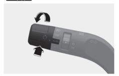
High Beam Assist will automatically adjust the headlamp range (switches between high beam and low beam) depending on the brightness of detected vehicles and certain road conditions.
