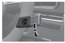
To shift the gear R (Reverse), rotate the rotary gear shift dial to R (Reverse) whilst depressing the brake pedal.
