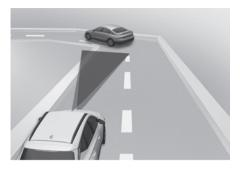
Your vehicle speed can be reduced due to a vehicle in the adjacent lane.
