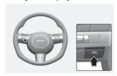
Whenever the vehicle is turned on, Lane Keeping Assist always turn on, and the grey (/♠\) indicator light illuminates on the cluster. When Lane Keeping Assist is on, press and hold the Lane Driving Assist (/⊕\) button to turn off the function.
