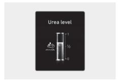
DEF (Diesel Exhaust Fluid) level gauge display shows the approximate amount of remaining urea solution inside the urea solution tank.
