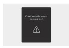
When the outside rearview mirror warning light is not working properly, the 'Check outside rearview mirror warning icon' warning message appears on the instrument cluster for several seconds, and the master (A) warning light illuminates on the cluster. If this occur, we recommend that your vehicle be inspected by a HYUNDAI authorised repairer.
