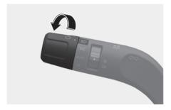
The headlight, position light, license plate light and instrument panel light are turned ON.
