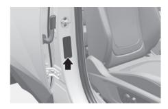
The vehicle certification label attached on the driver's (or front passenger's) side centre pillar gives the vehicle identification number (VIN).
