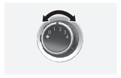
Turn the knob to the right to increase the fan speed and airflow. Turn the knob to the left to decrease fan speed and airflow. Setting the fan speed control knob to the "O" position turns off the fan.
