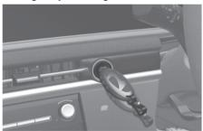
If the smart key battery is weak or the smart key does not work correctly, you can start the vehicle by pressing the Engine Start/Stop button with the smart key in the direction of the picture above.
