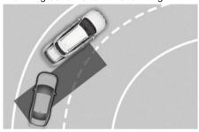
Blind-Spot Collision-Avoidance Assist may not operate properly when driving on a curved road. The function may recognise a vehicle in the same lane.
