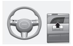
Press the Driving Assist button to turn Cruise Control off. The Cruise (MCRUISE) indicator will go off.
