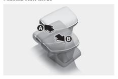
[A] Push the lever forwards once to shift up one gear.[B] Pull the lever backward once to shift down one gear.
