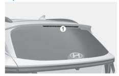
If the LED lamp (1) does not operate, we recommend that the system be inspected by a HYUNDAI authorised repairer.
