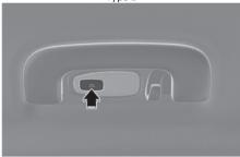
모:Press the button to turn on and off the rear lamp.
