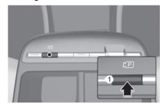
Press the Parking/View button (1) whilst the gear is in P (Park), D (Drive) or N (Neutral) to turn on the Rear View Monitor.
