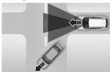
When a vehicle in front of you merges out of the lane, Smart Cruise Control may not immediately detect the new vehicle that is now in front of you. Always pay attention to road and driving conditions whilst driving.
