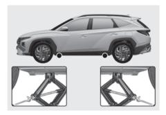
7. Place the jack at the designated jacking position under the frame closest to the tyre you are changing. The jacking positions are plates welded to the frame with two notches. Never jack at any other position or part of the vehicle. Doing so may damage the side seal molding or other parts of the vehicle.
