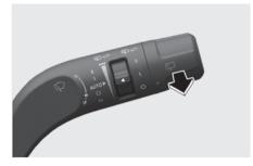
In the OFF (O) position, pull the lever gently toward you to spray washer fluid on the windscreen and to run the wipers 1-3 cycles. The spray and wiper operation continues until you release the lever. If the washer does not work, you may need to add washer fluid to the washer fluid reservoir.
