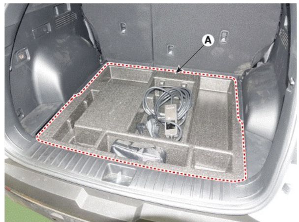
4-2. Remove the 12V battery service cover (A).
