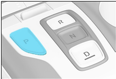
Step on brake pedal to park the vehicle, then select the shift lever in park (P)
