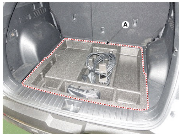
3-2. Remove the 12V battery service cover (A).
