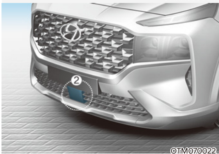
[1] : Front view camera, [2] : Front radar
