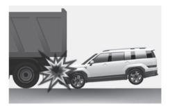
Just before impact, drivers often brake heavily. Such heavy braking lowers the front portion of the vehicle causing it to 'nosedive'. This is particularly important when the vehicle in front has a higher ground clearance. Airbags may not inflate if your vehicle is in a 'nosedive' condition because the collision forces detected by the sensors may have been significantly reduced.
