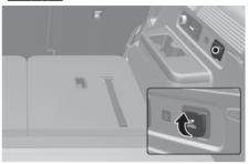
The AC inverter supplies 220 volts/200 watts electric power to operate electric accessories or equipment.
