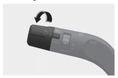
The position light, license plate light, and instrument panel light are turned ON.
