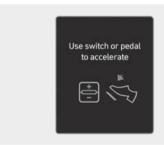
When Highway Driving Assist is operating, your vehicle will stop if the vehicle ahead of you stops. Also, if the vehicle ahead of you starts moving within 30 seconds after the stop, your vehicle will start as well. In addition, after the vehicle has stopped and 30 seconds have passed, the "Use switch or pedal to accelerate" message will appear on the instrument cluster. Depress the accelerator pedal or operate the + switch, - switch or IIO switch to start driving.
