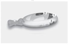
If you press any button on the Smart key during the Detect and Alert stage, the smart tailgate is deactivated.
