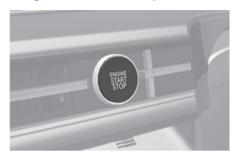
Whenever the front door is opened, the Engine Start/Stop button illuminates and goes off a few seconds after the door is closed.
