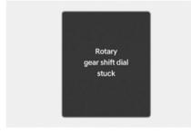
This message appears when the rotary gear shift dial does not return back to it's normal position after rotating it.
