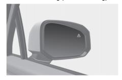
To warn the driver a vehicle is detected, the warning light on the outside rearview mirror and head-up display will illuminate.
