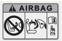
Never install a Child Restraint System in the front passenger seat, unless the airbag is deactived.
