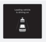
When a detected vehicle in front departs from a stop, Leading Vehicle Departure Alert will inform the driver by displaying the 'Leading vehicle is driving on' message on the instrument cluster and an audible warning will sound.
