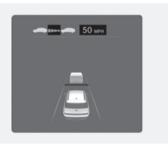
If you want to speed up temporarily without altering the set speed whilst Smart Cruise Control is operating, depress the accelerator pedal. Whilst the accelerator pedal is depressed, the set speed, distance level and target distance will blink on the cluster.
