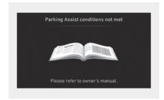
The 'Parking Assist Conditions not met' message appears when Parking/View (E) button has been pressed and held whilst Remote Smart Parking Assist is in standby. After a whilst, press and hold the Parking/View (E) button again to see if Remote Smart Parking Assist works.
