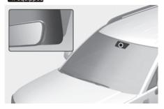
The Auto defogging reduces the possibility of fogging up the inside of the windscreen by automatically sensing the moisture on inside the windscreen.
