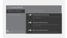
You can change Surround View Monitor Display contents by touching the setup icon (\*) on the screen whilst Surround View Monitor is operating, or selecting Driver assistance > Parking safety > Camera settings from the Settings menu in the infotainment system whilst the vehicle is on.
