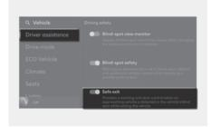
With the vehicle on, select **Settings** > **Vehicle** > **Driver assistance** > **Driving safety** > **Safe exit** from the Settings menu to turn on Safe Exit Warning and deselect to turn off the function.
