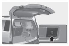
Press the power tailgate lock button whilst carrying the smart key. The power tailgate closes and locks automatically. Additionally, all doors will lock.
