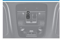
The sunshade opens automatically when the sunroof glass is opened by pushing the sunroof switch (A) rearward, but the sunshade does not close automatically when the sunroof glass is closed. Also, only the sunshade cannot be closed when the sunroof glass is opened.
