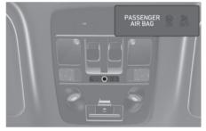
Insert the key or a similar rigid device into the passenger's front airbag ON/OFF switch and turn it to the OFF position [B]. The passenger airbag OFF indicator (%) illuminates and stays on until the passenger's front airbag is reactivated.
