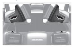
The paddle shifter is available when the gear is in the D (Drive) position in SPORT and TERRAIN (if equipped) mode.
