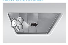
If the power sunshade or sunroof glass senses any obstacle whilst it is closing automatically, it will reverse direction then stop at a certain position.
