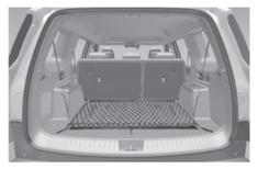
To keep items from shifting in the cargo area, use the 4 holders located in the cargo area side trim to attach the cargo net.
