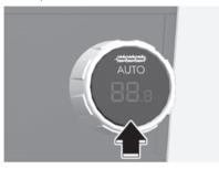
In automatic mode, press the AUTO button to select the fan speed from level 1 to 3.
