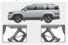
Insert the wheel lug wrench into the jack and turn it clockwise, raising the vehicle until the tyre clears the ground. Make sure the vehicle is stable on the jack.
