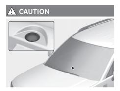
This vehicle is equipped with a solar radiation sensor located on the upper portion of the dashboard. With the air conditioning set to AUTO, the sensor will detect the solar radiation and adjust the indoor temperature automatically. Avoid placing any object on the solar radiation sensor for indoor temperature control.
