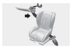
4. Push and pull on the Child Restraint System to confirm that the seat belt is holding it firmly in place.
