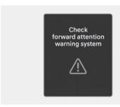
When Forward Attention Warning is not working properly, the 'Check forward attention warning system' warning message appears on the instrument cluster for several seconds, the (③) warning light illuminates on the instrument cluster, and an audible warning sounds until the Forward Attention Warning is working properly. If this occur, we recommend that your vehicle be inspected by a HYUNDAI authorised repairer.
