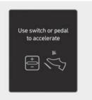
In traffic, your vehicle will stop if the vehicle ahead of you stops. Also, if the vehicle ahead of you starts moving, your vehicle will start as well. In addition, after the vehicle has stopped and a certain time have passed, the "Use switch or pedal to accelerate" message will appear on the instrument cluster. Depress the accelerator pedal or operate the + switch, - switch or II'O switch to start driving.
