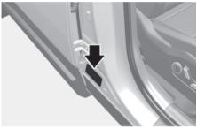
The vehicle certification label attached on the right front seat side centre pillar gives the vehicle identification number (VIN).
