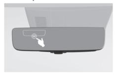
If the symbol shown in the illustration is displayed when using the Digital Centre Mirror in digital mirror mode, the system may be malfunctioning. The symbol will disappear in a few seconds.
