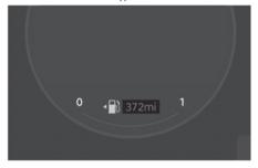
The distance to empty is the estimated distance the vehicle can be driven with the remaining fuel.
