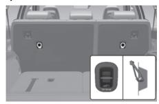
Top-tether anchorages for Child Restraint Systems are located on the rear of the seatbacks and on the rear of the front passenger seatback (if equipped).
