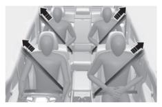
Your vehicle is equipped with driver's, front passenger's and rear passenger's (if equipped) pretensioner seat belts (retractor pretensioner). The pretensioner makes sure the seat belts fit tightly against your body in certain frontal or side collision(s). The pretensioner seat belts may be activated in some crashes where the frontal or side collision(s) is severe enough, together with the airbags.
