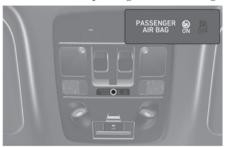
Insert the key or a similar rigid device into the passenger's front airbag ON/OFF switch and turn it to the ON position [A]. The passenger airbag ON indicator (®) illuminates.
