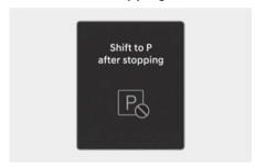
This message appears when the gear is shifted to P (Park) whilst the vehicle is moving.
