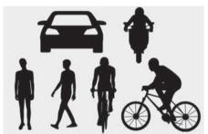
The illustration above shows the image the front view camera and front radar are capable of detecting as a vehicle, powered two-wheeler, pedestrian and cyclist.
