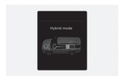
Both the motor and the engine power are used to drive the vehicle. (Battery & Engine → Wheel)
