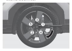
12.Use the wheel lug wrench to tighten the wheel bolts in the order shown. Double-check each wheel bolts until they are tight. After changing tyres, we recommend that a HYUNDAI authorised repairer tighten the wheel bolts to their proper torque as soon as possible. The wheel bolt should be tightened to 79~94 lbf. ft (11~13 kgf.m).
