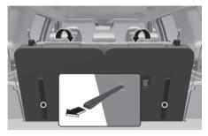
Pull the seatback angle adjustment strap to completely fold the seatback forward. Make sure the seatback is securely locked in place.
