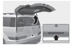
When the tailgate is closed, press the power tailgate open button to open the tailgate.
