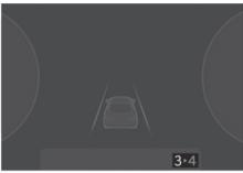
In the manual shift mode, this indicator informs which gear is recommended whilst driving, to save fuel.
