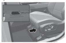
The hybrid battery cooling duct is located below the front passenger's seat. The cooling duct cools down the hybrid battery. When the hybrid battery cooling duct is blocked, the hybrid battery may be overheated.
