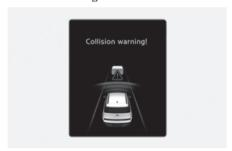
To warn the driver of a collision, Forward Safety warning light (ﷺ) blinks, the "Collision warning!" warning message will appear on the cluster, an audible warning will sound and the steering wheel will vibrate (if equipped).
