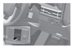
When the tailgate is closed, press the power tailgate open/close button for 1 second. The tailgate will open with a warning sound.
