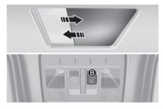
Push the power sunshade open switch (B), the power sunshade automatically slides open.
