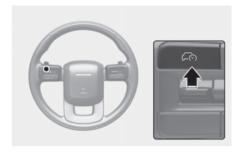
Press the Driving Assist button to turn Cruise Control off. The Cruise (ত্বেলেডাছ) indicator will go off.
