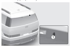
If the camera lens (1) is dirty, the displayed image may not be clear. In this case, clean it with a soft cloth dampened with water or a swab.
