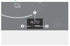
When the smart regeneration system is ON, the regenerative braking level appears as "AUTO" (1) on the instrument cluster. The "AUTO" appears in grey in the ready state. The system automatically controls the regenerative braking level (2) according to the smart regeneration system operating conditions. If the front radar detects a vehicle in front, the indicator light (3) appears in green.
