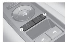
When pressing the  $(\triangle)$  portion (1) on the switch, all vehicle doors are locked.
