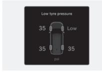
This warning message appears if the tyre pressure is low. The corresponding tyre on the vehicle is illuminated.
