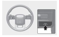
Whenever the vehicle is turned on, Lane Keeping Assist always turn on, and the grey (/♠\) indicator light illuminates on the instrument cluster. When Lane Keeping Assist is on, press and hold the Lane Driving Assist (/♠\) button to turn off the function.
