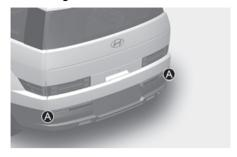
[A] Rear corner radar See the illustration above for the detailed location of the detecting sensors.
