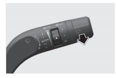
In the O (OFF) position, pull the lever gently toward you to spray washer fluid on the windscreen and to run the wipers 1-3 cycles. The spray and wiper operation continues until you release the lever. If the washer does not work, you may need to add washer fluid to the washer fluid reservoir.
