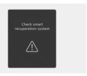
If the front radar is covered by any foreign material, such as snow, rain, or dirt, the detecting performance may decrease and disable the smart regeneration system.
