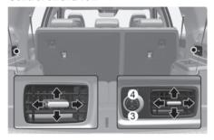
Press the air conditioning button (3) on the 3rd seat to start the system. (indicator light ON)
