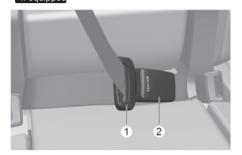
Insert the tongue plate (1) into the buckle (2) until an audible 'click' is heard, indicating the latch is locked. Pull the shoulder portion of the belt to snug the belt across your hips and remove slack. Make sure the seat belt is not twisted. When using the rear centre seat belt, use
