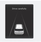
When the vehicle is stopped due to emergency braking, the "Drive carefully" warning message will appear on the cluster.
