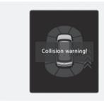
When an approaching vehicle from the rear is detected at the moment a door is opened, the "Collision warning!" warning message will appear on the cluster, and an audible warning will sound.  Safe Exit Warning will warn the driver when your vehicle speed is below 2 mph (3 km/h), and the speed of the approaching vehicle from the rear is above 4 mph (6 km/h).
