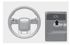
To turn Smart Cruise Control off, press the Driving Assist ( $\triangle$ ) button.
