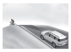
Forward Collision-Avoidance Assist may not detect other vehicles, powered two-wheelers, pedestrians or cyclists in front of you whilst driving uphill or downhill, adversely affecting the performance of the sensors.
