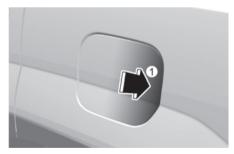
6. Pull the fuel filler door out to fully open.
