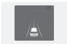
If the vehicle ahead and/or both lane markings are detected and your vehicle speed is below 112 mph (180 km/h), the green (②) indicator light appears on the cluster, and Lane Following Assist helps centre the vehicle in the lane by assisting the steering wheel.
