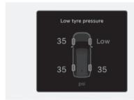
When the tyre pressure monitoring system warning indicator ((!)) is illuminated and a warning message appears on the cluster display, one or more of your tyres is significantly under-inflated. The Low Tyre Pressure Position Telltale will indicate which tyre is significantly under inflated by illuminating the corresponding position light.
