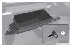
Remove the stoppers on both sides to allow the glove box to hang freely on the hinges.
