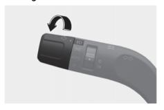
The headlight, position light, license plate light and instrument panel light are turned ON.
