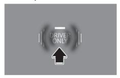
If you press the **DRIVER ONLY** button (indicator light ON), most of the air flow is directed toward the driver's seat.
