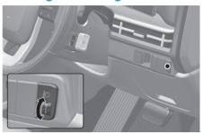
To adjust the headlight beam level according to the number of the passengers and loading weight in the luggage area, turn the beam leveling switch.
