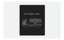
Only the engine power is used to drive the vehicle. (Engine → Wheel)
