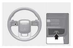
With the vehicle on, shortly press the Lane Driving Assist (/⊕\) button located on the steering wheel to turn on Lane Following Assist. The grey or green (⊖) indicator light will appear on the cluster. Press the button again to turn off the function.
