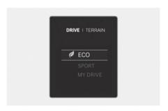
The mode changes, as the following, whenever the DRIVE/TERRAIN button is pushed up or down.
