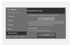
To delete all the registered digital key (smartphone), select **Settings** > **Vehicle** > **Digital key** > **Smartphone key** > **Delete all** in the infotainment system.
