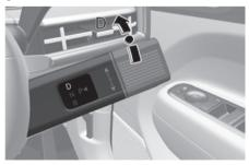
To shift the gear D (Drive), rotate the rotary gear shift dial to D (Drive) whilst depressing the brake pedal.
