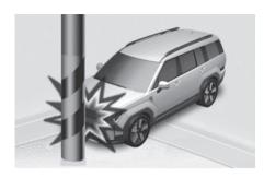
Airbags may not inflate if the vehicle collides with objects such as utility poles or trees, where the point of impact is concentrated and the collision energy is absorbed by the vehicle structure.
