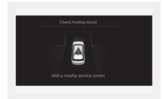
When Remote Smart Parking Assist is not working properly, the 'Check Parking Assist' warning message will appear on the infotainment system. If the message appears, stop using Remote Smart Parking Assist, and we recommend that your vehicle be inspected by a HYUNDAI authorised repairer.
