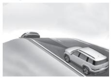
During uphill or downhill coasting, the smart regeneration system may not detect a moving vehicle in your lane, and cause your vehicle to accelerate. Also, your vehicle speed decelerates when a vehicle ahead is detected suddenly. Apply the brake pedal or accelerator pedal depending on the road and driving conditions.
