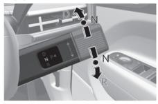
To shift the gear to N (Neutral), rotate the rotary gear shift dial to N (Neutral) from R (Reverse) or D (Drive) whilst depressing the brake pedal.
