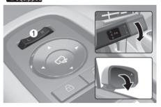
When the gear is shifted to the R (Reverse) position, the outside rearview mirrors rotate downwards to aid with driving in reverse.
