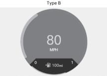
The fuel gauge indicates the approximate amount of fuel remaining in the fuel tank.
