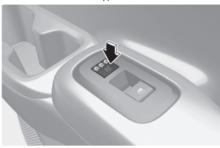
Whilst the engine is running, press the seat warmer switch to warm the rear seat.
