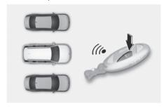
Press and hold the Remote Start button ( ) within 4 seconds until the engine starts.
