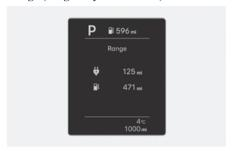
The range is the estimated distance the vehicle can be driven with the remaining fuel in the fuel tank (Petrol) and high-voltage (hybrid) battery (Electric).
