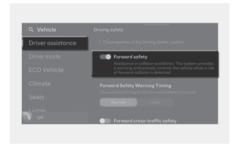
With the vehicle on, select **Settings** > **Vehicle** > **Driver assistance** > **Driving safety** from the settings menu in the infotainment system to set whether to use each function.
