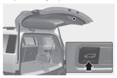
When the tailgate is opened, press and hold the tailgate open/close button to close the power tailgate. If you release the button whilst the tailgate is closing, power tailgate operation will stop.
