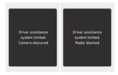
When the front windscreen where the front view camera is located, front radar cover, bumper or sensor is covered with foreign material, such as snow or rain, it can reduce the detecting performance and temporarily limit or disable Forward Collision-Avoidance Assist.
