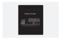
The engine braking is used to decelerate the vehicle. (Wheel → Engine)
