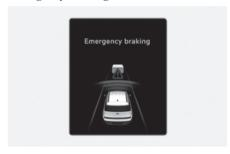
To warn the driver that emergency braking will be assisted, Forward Safety warning light (♣) blinks, the "Emergency braking" warning message will appear on the cluster, an audible warning will sound and the steering wheel will vibrate (if equipped).
