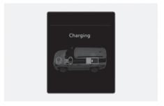
The engine and regenerative brake system charges up the high voltage battery. (Engine and Wheel  $\rightarrow$  Battery)
