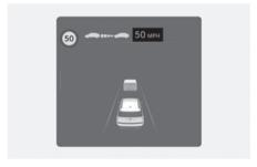
Manual Speed Limit Assist or Smart Cruise Control assists the vehicle to adjust its speed according to the speed limit. When the cruising speed is set as same as the speed limit, the vehicle automatically adjusts its speed if the speed limit changes. The function operates on the road which has a speed limit of 44 mph (70 km/h) or higher. When the function is active, the cruising speed on the instrument cluster appears in green.
