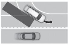
Blind-Spot Collision-Avoidance Assist may not operate properly when driving on a slope. The function may not detect the vehicle in the next lane or may incorrectly detect the ground or structure. Always pay attention to road and driving conditions whilst driving.
