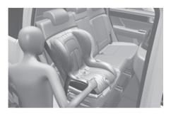
If your Child Restraint System manufacturer instructs or recommends you to use a top tether anchorage with the lap/shoulder belt, refer to "Installing a Child Restraint System" section for more information.
