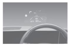
The Head-up display is an optional feature that allows the driver to view information projected onto a transparent screen whilst still keeping your eyes on the road ahead whilst driving.
