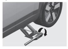
9. Loosen a wheel bolt with the wheel lug wrench and remove it with your fingers. Slide the wheel off the studs and lay it flat so it cannot roll away. To put the wheel on the hub, pick up the spare tyre, line up the holes with the studs and slide the wheel onto them. If this is difficult, tip the wheel slightly and get the top hole in the wheel lined up with the top stud. Then jiggle the wheel back and forth until the wheel can be slid over the other studs.
