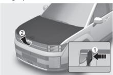
3. Go to the front of the vehicle, raise the bonnet slightly, push up the secondary bonnet release lever (1) inside of the bonnet centre and lift the bonnet (2).
