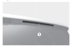
If the LED light (1) does not operate, we recommend that the system be inspected by a HYUNDAI authorised repairer.
