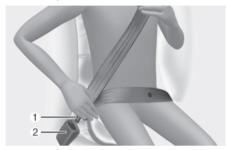
Pull the belt out of the retractor and insert the metal tab (1) into the buckle (2). There An audible 'click' sounds when the tab locks into the buckle. Make sure the seat belt is not twisted.
