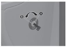
[A] Passenger airbag ON[B] Passenger airbag OFF
