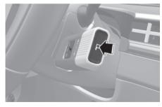
To shift the gear to P (Park), press the P button whilst depressing the brake pedal. If you turn the vehicle off in R (Reverse), N (Neutral) or D (Drive), the gear automatically shifts to P (Park).
