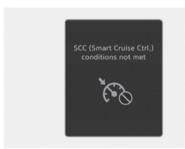
If the Driving Assist button, + switch, - switch or IIO switch is operated when Smart Cruise Control operating conditions are not satisfied, the "SCC (Smart Cruise Ctrl.) conditions not metmessage will appear on the cluster, and an audible warning will sound.
