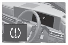
The TPMS Malfunction Indicator ((!)) illuminates after it blinks for about one minute when there is a problem with the Tyre Pressure Monitoring System.
