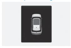
If the driver turns off the engine when the sunroof is not fully closed, the warning chime sounds for several seconds and the sunroof open warning appears on the cluster display.
