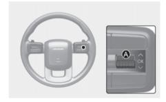
If you do not want to use Rear Occupant Alert, press the **OK** button on the steering wheel when the first alert is displayed on the cluster. Doing so will deactivate the second alert one time.
