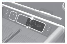
Press the USB port selection button whilst the engine is running. Press the upper portion of the button (1) to charge an electronic device. Press the lower portion of the button (2) to charge and listen to music with a media storage device. The USB port can be used after either indicator light turns on.
