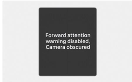
When there is an object right in front of the in-cabin camera or between the driver and the camera for a certain period of time Forward Attention Warning does not operate properly. If this occurs, the '**Forward attention warning disabled. Camera obscured**' warning message appears on the instrument cluster for several seconds, the (👁️) warning light illuminates on the instrument cluster, and an audible warning sounds until the Forward Attention Warning is working properly.
