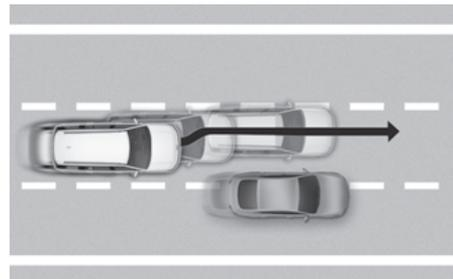
When vehicle speed is above 40 mph (60 km/h), if a detected vehicle around you is driving at a close distance, your vehicle will control steering in the opposite direction of the vehicle to assist in safe driving. If there a detected vehicle in both sides of the lane that are driving close to you, the function will not veer to the opposite side of the lane.
