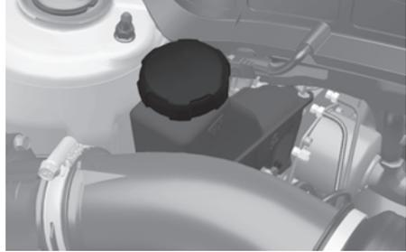
Check the fluid level in the reservoir periodically. The fluid level should be between MAX and MIN marks on the side of the reservoir.
