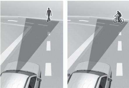
On curves, the smart regeneration system may not detect a vehicle in the same lane, and may accelerate the vehicle by lowering the regenerative braking intensity automatically. Your vehicle speed may decelerate by increasing regenerative braking intensity automatically if a vehicle is detected in an adjacent lane or when a vehicle ahead is detected suddenly. Apply the brake pedal or accelerator pedal depending on the road and driving conditions.
