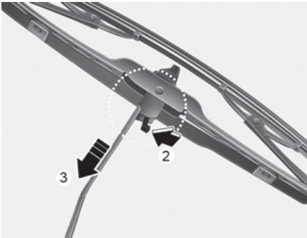
4. Install a new wiper blade assembly in the reverse order of removal.
