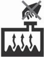
Never remove the engine coolant and/or battery system coolant cap or the drain plug whilst the engine and radiator are hot.
