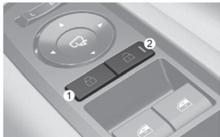
When pressing the (🔒) portion (1) on the switch, all vehicle doors are locked.
