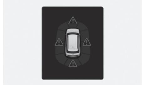
When the Parking Distance Warning is operating, if the function is not working normally or the ultrasonic sensor is blocked, the master warning light (△) appears in the direction of the corresponding sensor. You can check the warning in the Utility view on the cluster.
