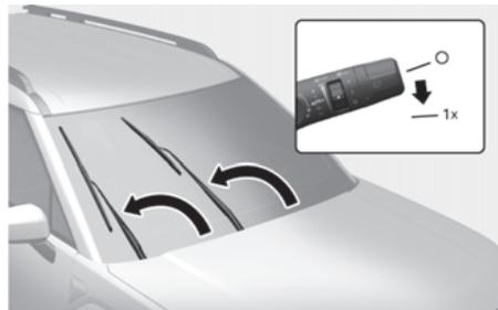
This vehicle has a "hidden" wiper design that cannot be lifted when in their bottom resting position.
