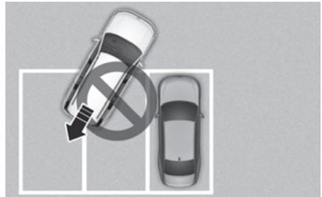
If Remote Smart Parking Assist is used, when parking in a parking space with a vehicle only on one side, your vehicle may cross the parking line to avoid the parked vehicle.
