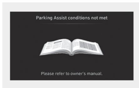
The '**Parking Assist Conditions not met**' message appears when Parking/View (ⓁⓅ) button has been pressed and held whilst Remote Smart Parking Assist is in standby. After a whilst, press and hold the Parking/View (ⓁⓅ) button again to see if Remote Smart Parking Assist works.
