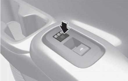
Whilst the engine is running, press the seat warmer switch to warm the rear seat.
