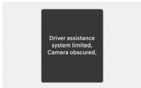
When the front windshield where the front view camera is located is covered with foreign material, such as snow or rain, it can reduce the detecting performance and temporarily limit or disable Intelligent Speed Limit Assist. If this occurs, the "**Driver assistance**
