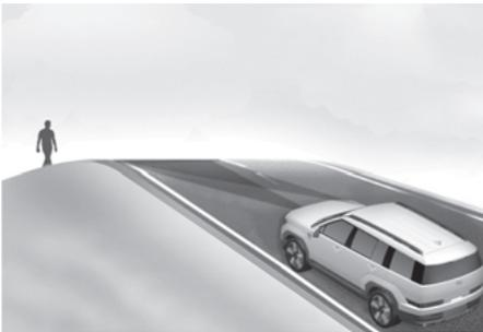
Forward Collision-Avoidance Assist may not detect other vehicles, powered two-wheelers, pedestrians or cyclists in front of you whilst driving uphill or downhill, adversely affecting the performance of the sensors.
