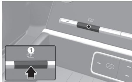
Press the Parking/View button (1) whilst the gear is in P (Park), D (Drive) or N (Neutral) to turn on the Rear View Monitor.
