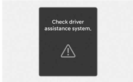
When Intelligent Speed Limit Assist is not working properly, the "**Check driver assistance system**" warning message will appear on the instrument cluster for several seconds, and the master (⚠) warning light and speed limit (⊖) warning light will appear on the instrument cluster. If this occurs, we recommend that your vehicle be inspected by a HYUNDAI authorised repairer.
