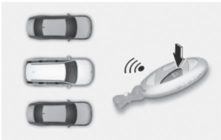
2. Press and hold the Remote Start button (🔑) within 4 seconds until the engine starts.
