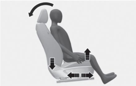
Relaxation comfort seats help distribute body pressure and concentrated weight on specific body parts that occur whilst sitting in the same position for a long period of time. The seat helps relieve fatigue and discomfort by providing the optimal sit position.
