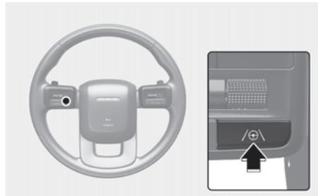
Whenever the vehicle is turned on, Lane Keeping Assist always turn on, and the grey (LKA) indicator light illuminates on the instrument cluster. When Lane Keeping Assist is on, press and hold the Lane Driving Assist (LKA) button to turn off the function.
