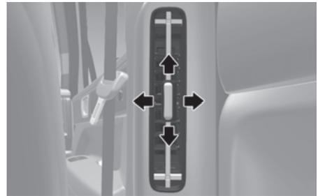
The instrument panel vent air flow can be directed up/down or left/right using the vent adjustment lever.
