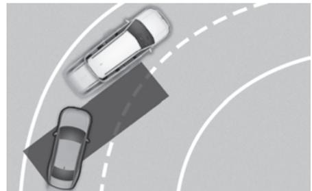
Blind-Spot Collision-Avoidance Assist may not operate properly when driving on a curved road. The function may recognise a vehicle in the same lane.
