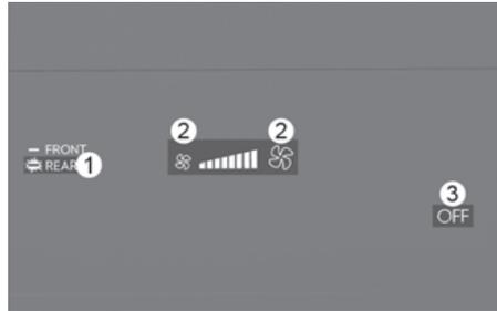
1. Press the 3rd row air conditioning FRONT/REAR button located on the front climate control panel and set the fan speed to the desired speed with the 3rd row fan speed button (2). (indicator light on the REAR button will illuminate).
