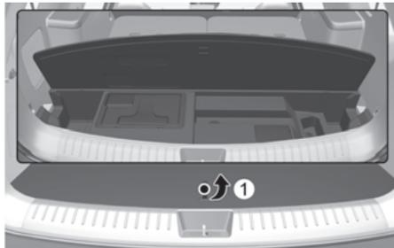
3. Open the emergency cable cover located in the cargo tray with a small blade tool (e.g. screwdriver or similar) (2) and pull the emergency cable.
