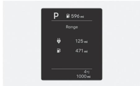
The range is the estimated distance the vehicle can be driven with the remaining fuel in the fuel tank (Petrol) and high-voltage (hybrid) battery (Electric). If the estimated distance is below 1 mi. (1 km), the trip computer will display "---" as the range.
