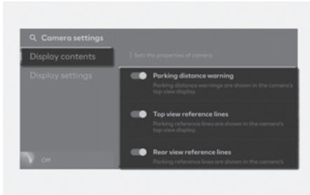
You can change Surround View Monitor **Display contents** by touching the setup icon (⚙️) on the screen whilst Surround View Monitor is operating, or selecting **Driver assistance > Parking safety > Camera settings** from the **Settings** menu in the infotainment system whilst the vehicle is on.
