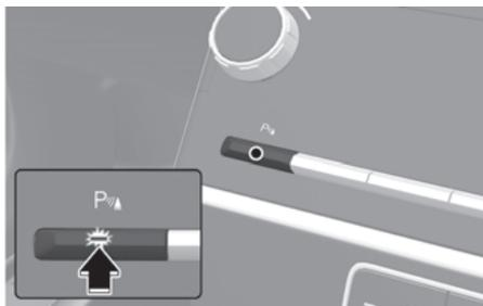
Press the Parking Safety (P<sub>SA</sub>) button to turn on Forward/Reverse Parking Distance Warning. Press the button again to turn off the function.
