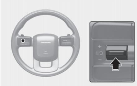
Press the **||** switch to temporarily pause the set speed limit. The set speed limit will turn off but the Speed Limit (LIMIT) indicator will stay on.
