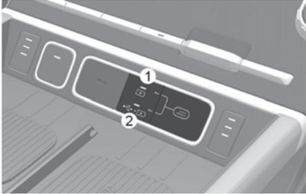
Press the USB port selection button whilst the engine is running. Press the upper portion of the button (1) to charge an electronic device. Press the lower portion of the button (2) to charge and listen to music with a media storage device. The USB port can be used after either indicator light turns on.
