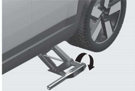
9. Loosen a wheel bolt with the wheel lug wrench and remove it with your fingers. Slide the wheel off the studs and lay it flat so it cannot roll away. To put the wheel on the hub, pick up the spare tyre, line up the holes with the studs and slide the wheel onto them. If this is difficult, tip the wheel slightly and get the top hole in the wheel lined up with the top stud. Then jiggle the wheel back and forth until the wheel can be slid over the other studs.
