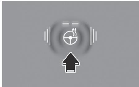
When the Engine Start/Stop button is in the ON position or when the engine is running, press the steering wheel heater button to warm the steering wheel. The indicator on the button illuminates. To turn the steering wheel heater off, press the button again. The indicator on the button turns off.
