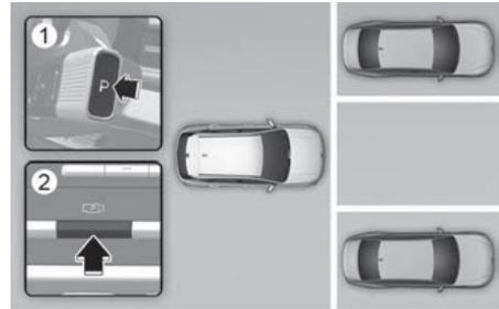
Method (2) Using the function with engine on
