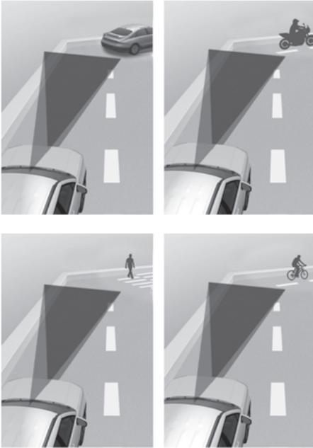
Forward Collision-Avoidance Assist may not detect other vehicles, powered two-wheelers, pedestrians or cyclists in front of you when driving on curved roads adversely affecting the performance of the sensors. This may result in no warning, braking assist or steering assist (if equipped) when necessary.
