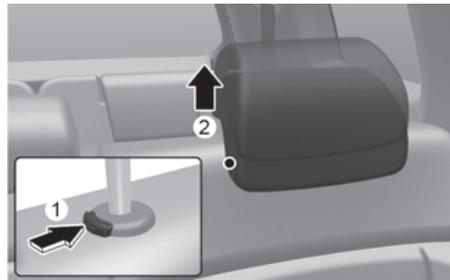
To remove the head restraint:
