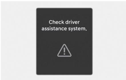
When High Beam Assist is not working properly, the "**Check driver assistance system**" warning message may appear, and the (⚠) warning light may illuminate on the instrument cluster. We recommend that the system be inspected by a HYUNDAI authorised repairer.
