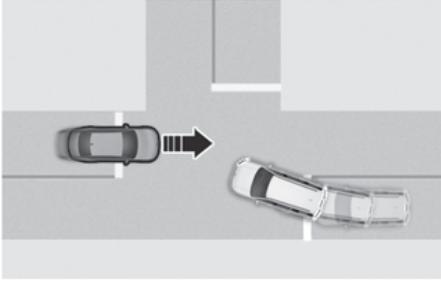
Junction Turning function can help avoid a collision with an oncoming vehicle or powered two-wheeler in an adjacent lane when turning right at a crossroad with the turn signal on by applying emergency braking.
