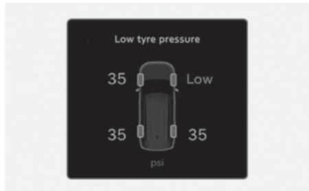
The tyre pressure of each tyre appears. For more information, refer to "Tyre pressure monitoring system (TPMS)" section in chapter 8.
