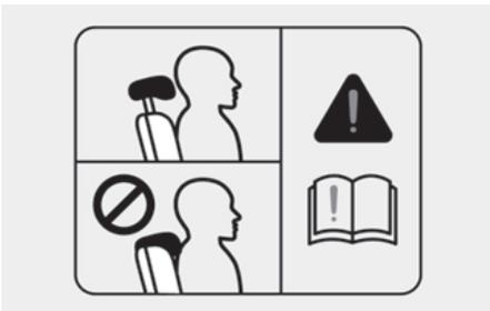
When sitting on the rear seat, do not adjust the height of the head restraint to the lowest position.
