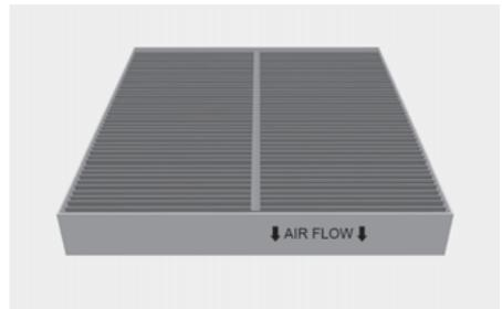
Install a new cabin air filter in the correct direction with the arrow symbol (↓) facing downwards, to prevent noise and reduce effectiveness.
