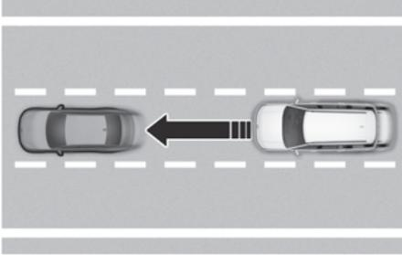
Highway Driving Assist helps maintain a set distance and speed from the vehicle ahead whilst driving on a highway main section and helps centre the vehicle in the lane.
