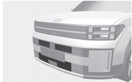
Active air flap system controls the air flap below the front bumper to cool the vehicle parts and improve energy efficiency.
