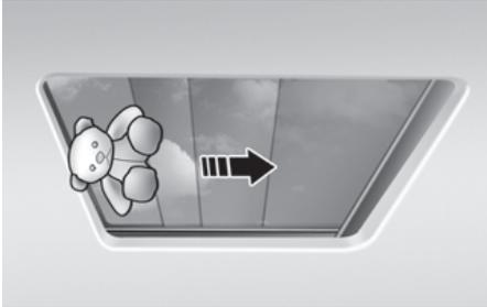
If the power sunshade or sunroof glass senses any obstacle whilst it is closing automatically, it will reverse direction then stop at a certain position.
