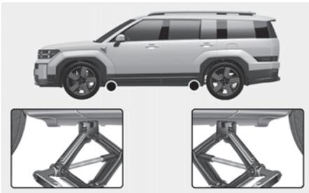
8. Insert the wheel lug wrench into the jack and turn it clockwise, raising the vehicle until the tyre clears the ground. Make sure the vehicle is stable on the jack.
