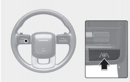
With the vehicle on, shortly press the Lane Driving Assist (/⊕) button located on the steering wheel to turn on Lane Following Assist. The grey or green (⊕) indicator light will appear on the cluster. Press the button again to turn off the function.
