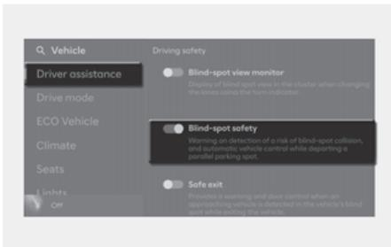
With the vehicle on, select **Settings > Vehicle > Driver assistance > Driving safety > Blind-spot safety** from the settings menu to set whether to use each function.
