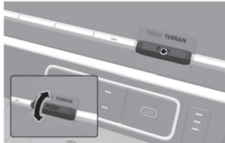
Press the DRIVE/TERRAIN button to change from normal driving mode to multi terrain mode. Press the button up or down to select SNOW, MUD, or SAND.
