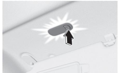
Push the switch to turn the lamp on or off.
