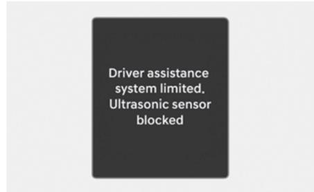
If this occurs the '**Driver assistance system limited. Ultrasonic sensor blocked**' warning message appears on the instrument cluster. Parking Distance Warning operates properly when snow, rain or foreign material is removed.
