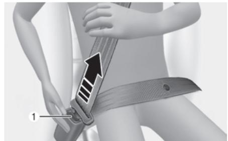
Once released, the belt should automatically draw back into the retractor. If this does not happen, check the belt to be sure it is not twisted, then try again.
