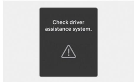
When Safe Exit Warning is not working properly, the "**Check driver assistance system**" warning message will appear on the cluster for several seconds, and the master warning light (
