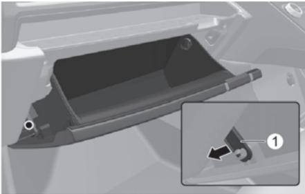
2. Remove the stoppers on both sides to allow the glove box to hang freely on the hinges.
