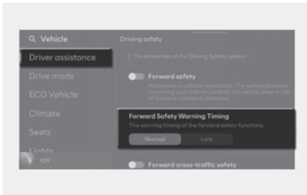
With the vehicle on, select **Settings** > **Vehicle** > **Driver assistance** > **Driving safety** > **Forward Safety Warning Timing** settings menu in the infotainment system to change the initial warning activation time for Forward Collision-Avoidance Assist. The warning time can be set to either **Normal** or **Late**.
