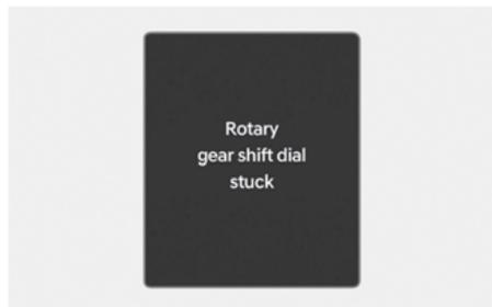
This message appears when the rotary gear shift dial does not return back to its normal position after rotating it. We recommend that your vehicle be inspected by a HYUNDAI authorised repairer.
