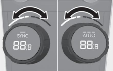
3. We recommend that you use the AUTO (automatic control) button to keep indoor air pleasant, regardless of the season. Normally, set the temperature to 22 °C. The AUTO (automatic control) button will not illuminate once you select the following functions. The selected function of the following will be activated whilst AUTO system remains operating.
