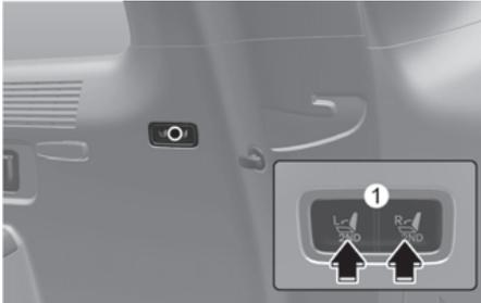
This feature can make it easier for you to fold the 2nd row seatback forward when the tailgate is open.
