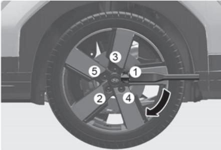
12. Use the wheel lug wrench to tighten the wheel bolts in the order shown. Double-check each wheel bolts until they are tight. After changing tyres, we recommend that a HYUNDAI authorised repairer tighten the wheel bolts to their proper torque as soon as possible. The wheel bolt should be tightened to 79~94 lbf. ft (11~13 kgf.m).
