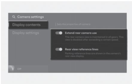
You can change Rear View Monitor **Display contents** by touching the setup icon (⚙️) on the screen whilst Rear View Monitor is operating, or selecting **Driver assistance > Parking safety > Camera settings** from the **Settings** menu in the infotainment system whilst the vehicle is on.
