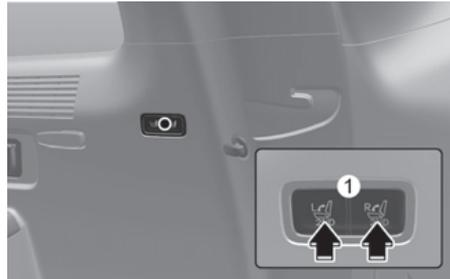
This feature can make it easier for you to fold or unfold the 2nd row seatback forward or rearward when the tailgate is open.
