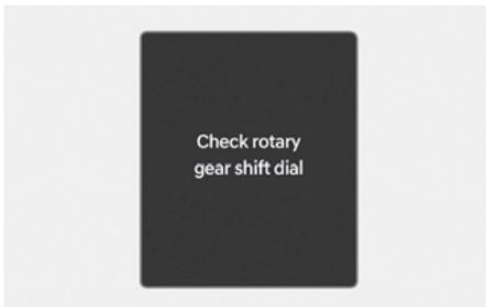
This message appears when there is a malfunction with the rotary gear shift dial. We recommend that your vehicle be inspected by a HYUNDAI authorised repairer.
