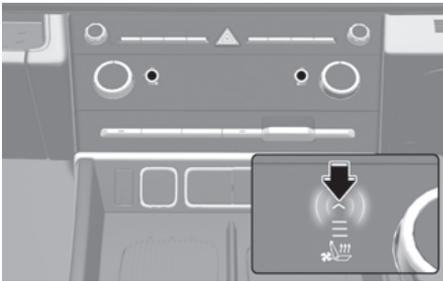
Whilst the engine is running, touch the icon to warm the driver's seat or front passenger's seat.
