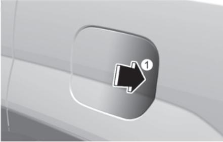
4. Pull the fuel filler door outward to access the fuel tank cap.
