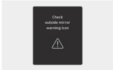
When the outside rearview mirror warning light is not working properly, the "**Check outside mirror warning icon**" warning message appears on the instrument cluster for several seconds, and the master (⚠) warning light illuminates on the cluster. If this occur, we recommend that your vehicle be inspected by a HYUNDAI authorised repairer.
