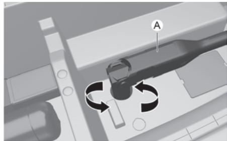
5. After the spare tyre reaches the ground, continue to turn the wrench counterclockwise, and draw the spare tyre outside. Never rotate the wrench excessively, otherwise the spare tyre carrier may be damaged.
