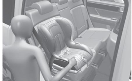
If your Child Restraint System manufacturer instructs or recommends you to use a top tether anchorage with the lap/shoulder belt, refer to "Installing a Child Restraint System" section for more information.
