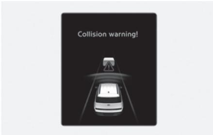
Whilst Smart Cruise Control is operating, when the collision risk with the vehicle ahead is high, the **"Collision warning!"** warning message will appear on the instrument cluster, an audible warning will sound, and the steering wheel vibrates (if equipped) to warn the driver. Always have your eyes on the road whilst driving, and if necessary, depress the brake pedal to reduce your driving speed in order to maintain a safe distance.
