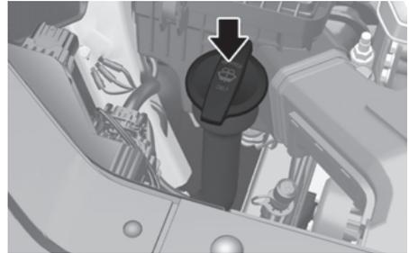
Check the fluid level in the washer fluid reservoir and add fluid if necessary. Plain water may be used if washer fluid is not available. However, use washer solvent with antifreeze characteristics in cold climates to prevent freezing.
