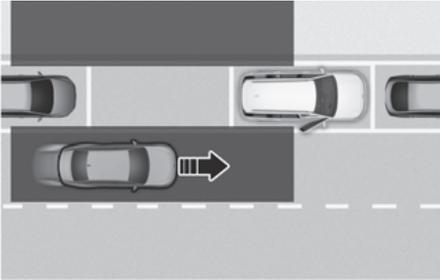
whilst your vehicle is stopped, and if Safe Exit Warning detects a vehicle approaching the rear corner of your vehicle and a passenger opens a door, Safe Exit Warning may warn you with a warning message and a warning sound to help avoid a collision.
