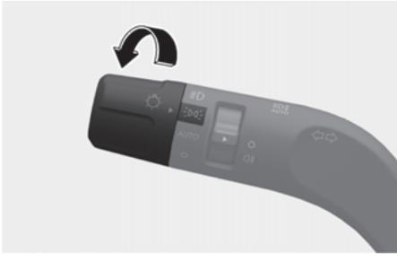
The position light, license plate light, and instrument panel light are turned ON.
