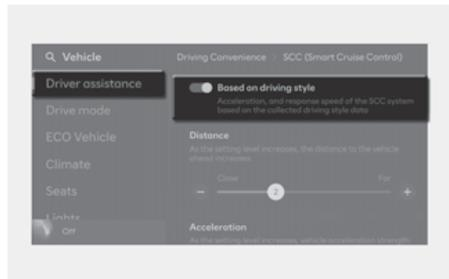
With the vehicle on, if **Settings > Vehicle > Driver assistance > Driving convenience > SCC (Smart Cruise Control) > Based on driving style** is selected from the Settings menu, Smart Cruise Control will operate based on the driver's driving style, such as vehicle distance, acceleration, reaction speed.
