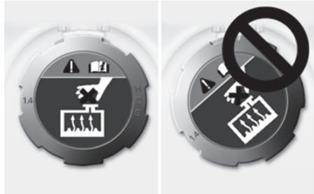
2. Make sure that the tiny protrusions inside the coolant cap is securely interlocked.
