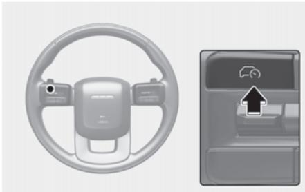
2. Push the + switch up or - switch down, and release it at the desired speed.
