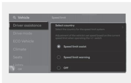
With the vehicle on, select or deselect **Settings > Vehicle > Driver assistance > Speed limit** from the Settings menu to set whether to use each function.
