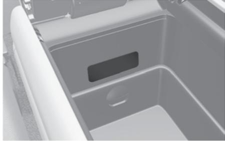
The two-way multi console lamp turns on when you turn on the interior button lights with the lighting control lever whilst the Engine Start/Stop button is in the ON position.
