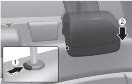
To reinstall the head restraint:
