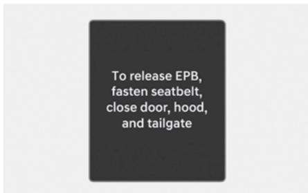
If the driver's seat belt is unfastened, or the bonnet, tailgate, doors are open, and you try to drive with EPB applied, a warning sounds and a message appears.
