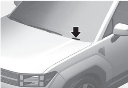
The VIN is also on a plate attached to the top of the left side dashboard. The number on the plate can easily be seen through the windscreen from outside.
