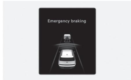
To warn the driver that emergency braking will be assisted, Forward Safety warning light (⚠️) blinks, the "**Emergency braking**" warning message will appear on the cluster, an audible warning will sound and the steering wheel will vibrate (if equipped).
