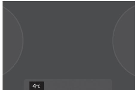
The outside ambient temperature appears in the lower portion of the cluster display. The temperature reads in Fahrenheit or Celsius depending on the units selected from the Settings menu in the instrument cluster or infotainment system.
