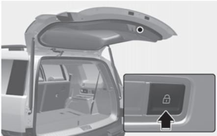
Press the power tailgate lock button whilst carrying the smart key. The power tailgate closes and locks automatically. Additionally, all doors will lock.
