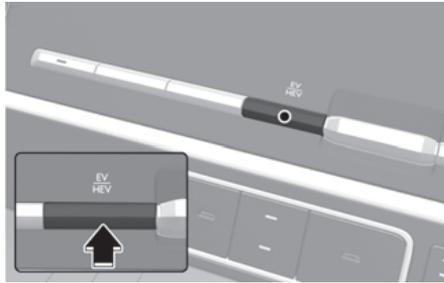
Pressing the EV/HEV button changes the plug-in hybrid system modes, between Electric (CD) mode and Hybrid (CS) mode.
