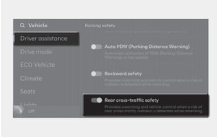
With the vehicle on, select **Settings > Driver assistance > Parking safety > Rear cross-traffic safety** from the settings menu in the infotainment system to turn on Rear Cross-Traffic Collision-Avoidance Assist and deselect to turn off the function.
