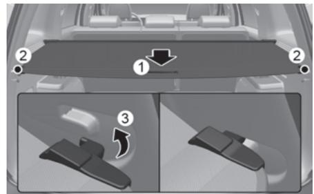
1. Pull the cargo security screen towards the rear of the vehicle by the handle (1).
