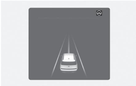
If the vehicle ahead and/or both lane markings are detected and your vehicle speed is below 112 mph (180 km/h), the green (⊕) indicator light appears on the cluster, and Lane Following Assist helps centre the vehicle in the lane by assisting the steering wheel.
