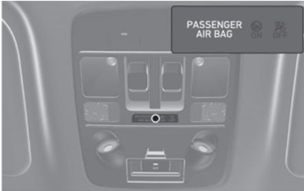
Insert the key or a similar rigid device into the passenger's front airbag ON/OFF switch and turn it to the OFF position [B]. The passenger airbag OFF indicator (
