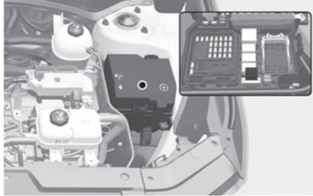
High voltage cut-off switch is a device located inside the engine compartment to block the battery's high voltage when your vehicle is inspected at a HYUNDAI authorised repairer.
