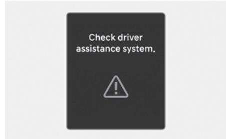
When Smart Cruise Control is not working properly, the "**Check driver assistance system**" warning message and the master ( $\triangle$ ) warning light will appear on the instrument cluster. We recommend that your vehicle be inspected by a HYUNDAI authorised repairer.
