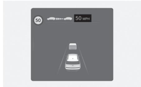
Manual Speed Limit Assist or Smart Cruise Control assists the vehicle to adjust its speed according to the speed limit. When the cruising speed is set as same as the speed limit, the vehicle automatically adjusts its speed if the speed limit changes. The function operates on the road which has a speed limit of 44 mph (70 km/h) or higher. When the function is active, the cruising speed on the instrument cluster appears in green.
