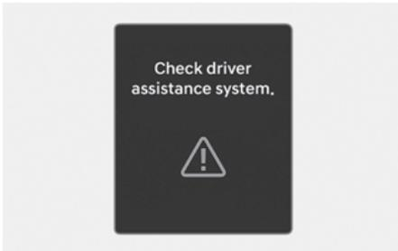
When Blind-Spot Collision Warning is not working properly, the "**Check driver assistance system**" warning message will appear on the instrument cluster for several seconds, and the master (⚠) warning light will appear on the instrument cluster. If this occurs, we recommend that your vehicle be inspected by a HYUNDAI authorised repairer.
