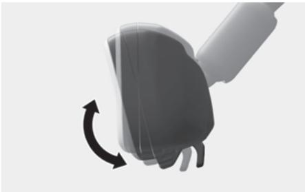
The height of the rearview mirror can be adjusted to suit your driving posture. Change to optical mirror mode, adjusting the rearview mirror angle by moving it up and down.
