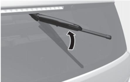
1. Within 20 seconds after the vehicle is turned off, push down the wiper switch to the MIST position for about 2 seconds until the wipers move to the lowest position.
