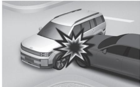
Front airbags may not inflate in side impact collisions, because occupants move in the direction of the collision. Side and curtain airbags may inflate depending on the severity of impact.
