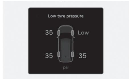
This warning message appears if the tyre pressure is low. The corresponding tyre on the vehicle is illuminated.
