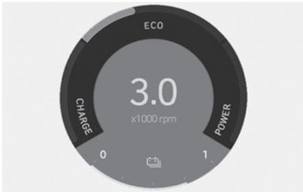
The power gauge indicates whether the current driving condition is fuel efficient or not.
