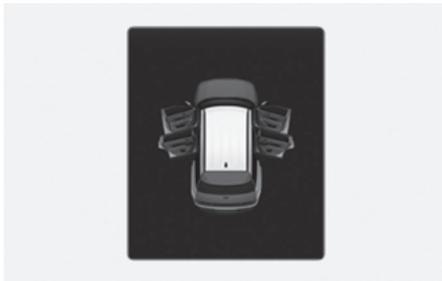
This warning appears if any door or bonnet or tailgate is left open. The warning indicates which door is open on the cluster display.
