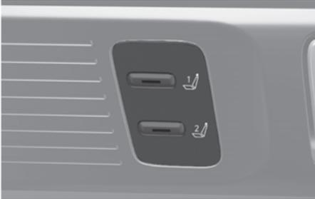
The Integrated Memory System for the driver's seat is equipped on some models and allows the driver to store and recall the following memory settings with a simple button operation.
