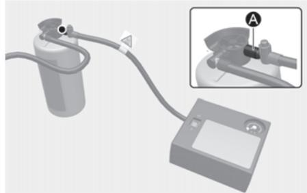
3. Unscrew the valve cap from the valve of the defective wheel and screw the filling hose (3) of the sealant bottle onto the tyre valve.
