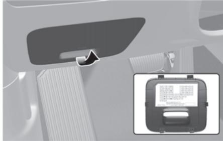
Inside the fuse panel cover, you can find the fuse/relay label describing fuse/relay names and ratings.
