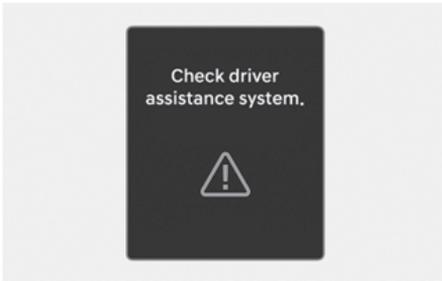
When Rear Cross-Traffic Collision-Avoidance Assist is not working properly, the "**Check driver assistance system**" warning message appears on the instrument cluster for several seconds, and the master (⚠) warning light illuminates on the instrument cluster. If this occur, we recommend that your vehicle be inspected by a HYUNDAI authorised repairer.
