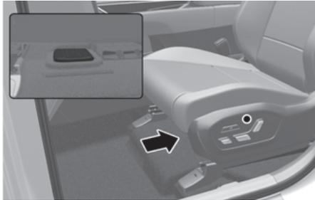
The hybrid battery cooling duct is located below the front passenger's seat. The cooling duct cools down the hybrid battery. When the hybrid battery cooling duct is blocked, the hybrid battery may be overheated.
