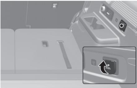
The AC inverter supplies 220 volts/200 watts electric power to operate electric accessories or equipment.
