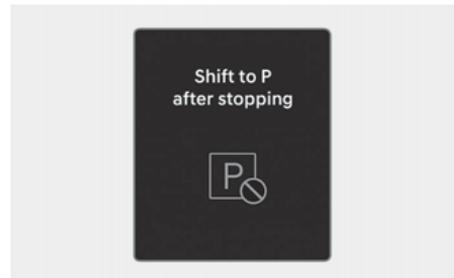
This message appears when the gear is shifted to P (Park) whilst the vehicle is moving.
