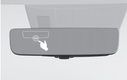
If the symbol shown in the illustration is displayed when using the Digital Centre Mirror in digital mirror mode, the system may be malfunctioning. The symbol will disappear in a few seconds.
