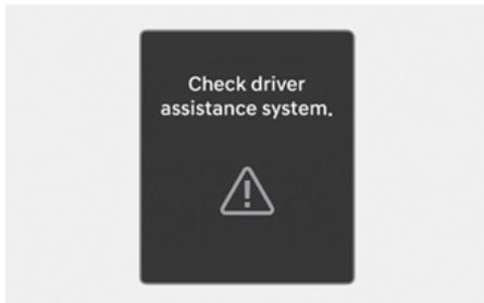
When Lane Keeping Assist is not working properly, the '**Check Driver assistance system.**' warning message, the master (⚠) warning light, and yellow Lane Keeping Assist (LKA) warning light appears on the cluster. If this occurs, we recommend that your vehicle be inspected by a HYUNDAI authorised repairer.
