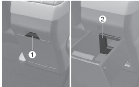
To open the storage compartment, pull the lever (1). This tray is designed to store long items.
