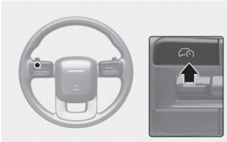
2. Press the Driving Assist button at the desired speed. The set speed and Cruise (
