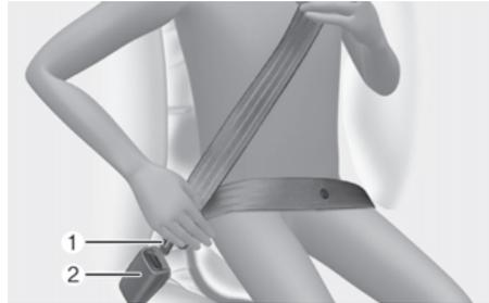
Pull the belt out of the retractor and insert the metal tab (1) into the buckle (2). There An audible 'click' sounds when the tab locks into the buckle. Make sure the seat belt is not twisted.
