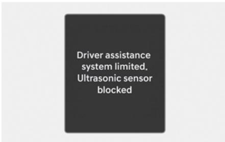
The "**Driver assistance system limited. Camera obscured.**" or "**Driver assistance system limited. Ultrasonic sensor blocked.**" warning message appears on the cluster if the following situations occur:
