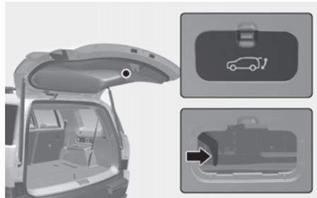
To unlock and open the tailgate manually from inside the cargo area, perform the following:
