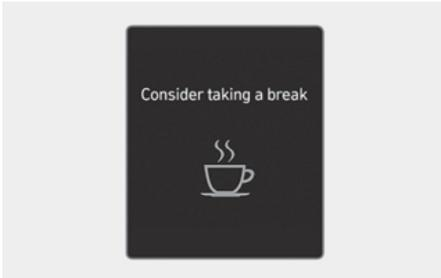
The Driver Drowsiness Attention Warning monitors your eyes whilst driving. When the driver's eyes are constantly closed or not facing forward frequently, the Driver Drowsiness Attention Warning recommends a break to help with safe driving. The '**Consider taking a break**' warning message and the (☕) warning light appears on the cluster, and an audible warning sounds until the off conditions are met.
