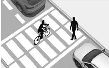
If there is a pedestrian(s) or bicycle(s) in between you and the vehicle in front, Leading Vehicle Departure Alert may not operate properly.
