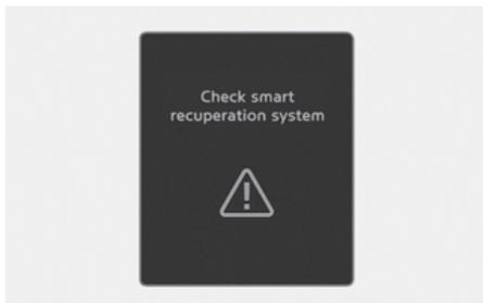
If the front radar is covered by any foreign material, such as snow, rain, or dirt, the detecting performance may decrease and disable the smart regeneration system.
