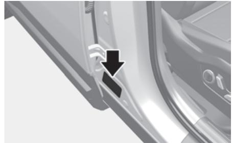
The vehicle certification label attached on the right front seat side centre pillar gives the vehicle identification number (VIN).
