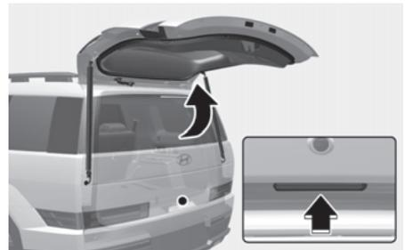
When the tailgate is closed, press the power tailgate open button to open the tailgate.
