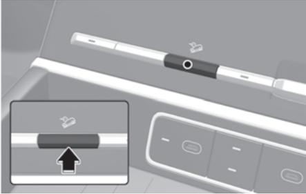
Downhill Brake Control assists when descending down a steep hill without having to depress the brake pedal.
