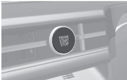
Whenever the front door is opened, the Engine Start/Stop button illuminates and goes off a few seconds after the door is closed.
