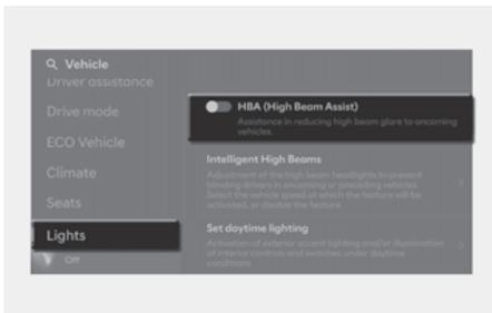
With the Engine Start/Stop button in the ON position, select **Settings > Vehicle > Lights > HBA (High Beam Assist)** from the Settings menu to turn on High Beam Assist and deselect to turn off the function.
