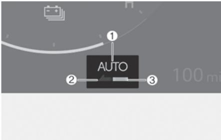
When the smart regeneration system is ON, the regenerative braking level appears as **"AUTO"** (1) on the instrument cluster. The **"AUTO"** appears in grey in the ready state. The system automatically controls the regenerative braking level (2) according to the smart regeneration system operating conditions. If the front radar detects a vehicle in front, the indicator light (3) appears in green.
