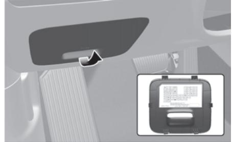
4. Refer to the label on the inside of the fuse panel cover to locate the suspected fuse location.
