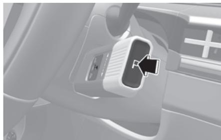
To shift the gear to P (Park), press the P button whilst depressing the brake pedal.
