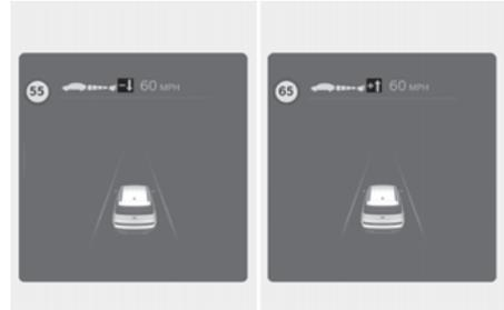
If the speed limit of the road changes during the operation of Manual Speed Limit Assist or Smart Cruise Control, an arrow in the direction of up or down is displayed to inform the driver that the set speed needs to be changed. At this time, the driver can change the set speed according to the speed limit by using the + or - switch on the steering wheel.
