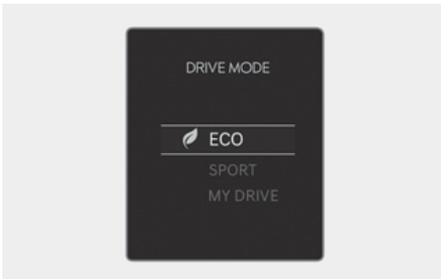
The mode changes, as the following, whenever the DRIVE MODE button is pushed up or down.
