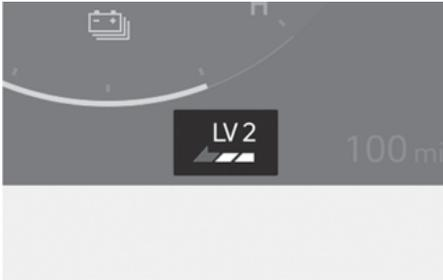
The selected regenerative braking level appears on the instrument cluster.
