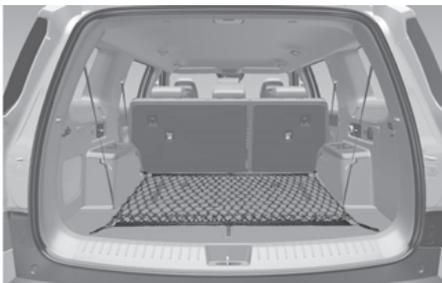
To keep items from shifting in the cargo area, use the 4 holders located in the cargo area side trim to attach the cargo net.
