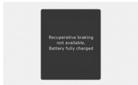
Regenerative braking is temporarily limited to protect the battery because the high voltage battery is fully charged.
