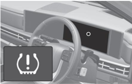
The TPMS Malfunction Indicator (
