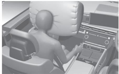
After complete inflation, the airbag immediately starts deflating, enabling the driver to maintain forward visibility and steer or operate other controls.
