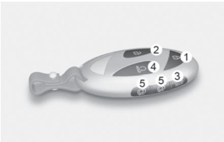
Your HYUNDAI uses a smart key that is used to lock or unlock the driver's and passenger's doors and the rear tailgate, and start the engine.
