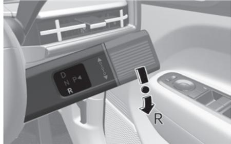
To shift the gear R (Reverse), rotate the rotary gear shift dial to R (Reverse) whilst depressing the brake pedal.
