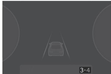
In the manual shift mode, this indicator informs which gear is recommended whilst driving, to save fuel.
