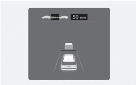
If you want to speed up temporarily without altering the set speed whilst Smart Cruise Control is operating, depress the accelerator pedal. Whilst the accelerator pedal is depressed, the set speed, distance level and target distance will blink on the cluster.
