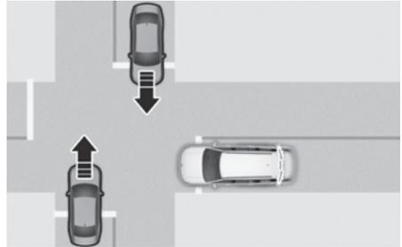
Junction Crossing function can help avoid a collision with oncoming vehicles on the left or right side when crossing an intersection by applying emergency braking.
