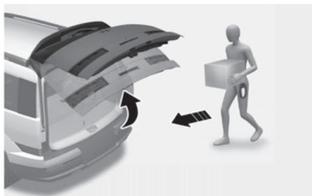
On a vehicle equipped with a smart key, the tailgate can be opened with hands-free activation using the smart tailgate system.
