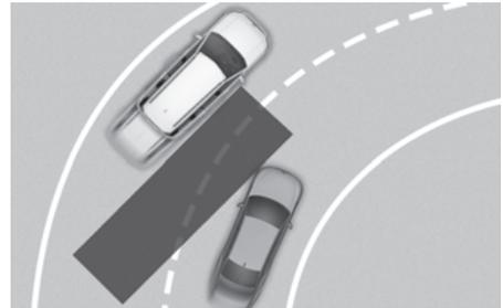
Blind-Spot Collision-Avoidance Assist may not operate properly when driving on a curved road. The function may not detect the vehicle in the next lane.
