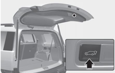
When the tailgate is opened, press and hold the tailgate open/close button to close the power tailgate. If you release the button whilst the tailgate is closing, power tailgate operation will stop.
