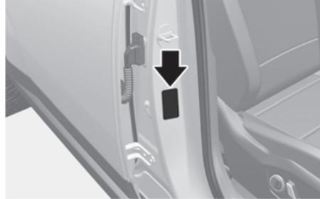
All specifications (sizes and pressures) can be found on a label attached to the driver's side centre pillar.
