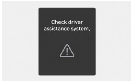
When Reverse Parking Collision-Avoidance Assist or other related functions are not working properly, the "**Check driver assistance system.**" warning message appears on the instrument cluster, and Reverse Parking Collision-Avoidance Assist turns off automatically. We recommend that your vehicle be inspected by a HYUNDAI authorised repairer.
