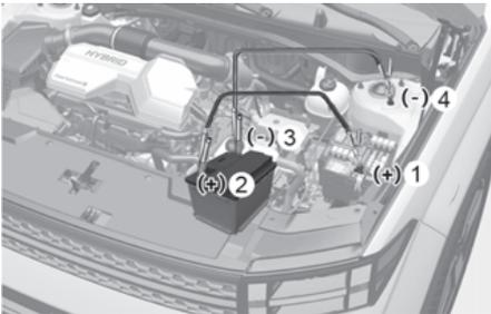
6. Connect the jumper cables in the exact sequence shown in the illustration. First connect one jumper cable to the red, positive (+) jumper terminal of your vehicle (1).
