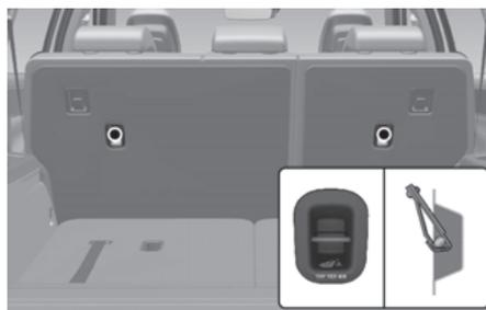
Top-tether anchorages for Child Restraint Systems are located on the rear of the seatbacks and on the rear of the front passenger seatback (if equipped).
