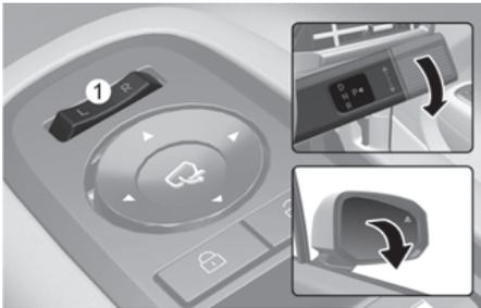
When the gear is shifted to the R (Reverse) position, the outside rearview mirrors rotate downwards to aid with driving in reverse.
