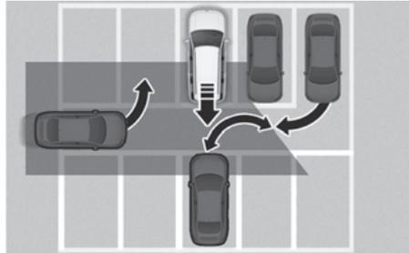
Rear Cross-Traffic Collision-Avoidance Assist may detect vehicles which are parking or pulling out near your vehicle (for example, a vehicle leaving beside your vehicle, a vehicle parking or pulling out in the rear area, a vehicle approaching your vehicle making a turn, etc.). If this occurs, the function may unnecessarily warn the driver and control the brake.
