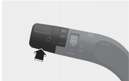
To turn on the high beam headlight, push the lever away from you. The lever returns to its original position.
