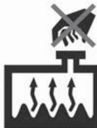
Never remove the engine coolant and/or battery system coolant cap or the drain plug whilst the engine and radiator are hot. Hot coolant and steam may blow out under pressure, causing serious injury.
