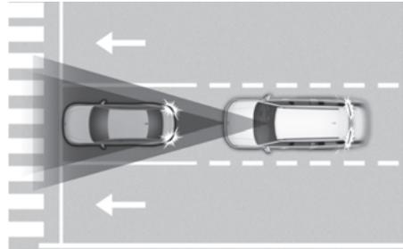
Forward Collision-Avoidance Assist is designed to help detect and monitor the vehicle ahead or help detect a powered two-wheeler, pedestrian or cyclist in the roadway and warn the driver that a collision is imminent with a warning message and warning and apply emergency braking.
