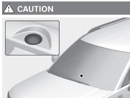
This vehicle is equipped with a solar radiation sensor located on the upper portion of the dashboard. With the air conditioning set to AUTO, the sensor will detect the solar radiation and adjust the indoor temperature automatically. Avoid placing any object on the solar radiation sensor for indoor temperature control.
