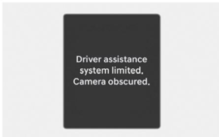
When the front windscreen where the front view camera is located, or sensor is covered with foreign material, such as snow or rain, it can reduce the detecting performance and temporarily limit or disable Lane Keeping Assist.
