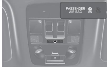
Insert the key or a similar rigid device into the passenger's front airbag ON/OFF switch and turn it to the ON position [A]. The passenger airbag ON indicator (
