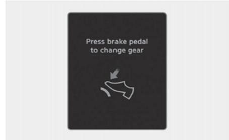
This message appears when the brake pedal is not depressed whilst shifting the gear.
