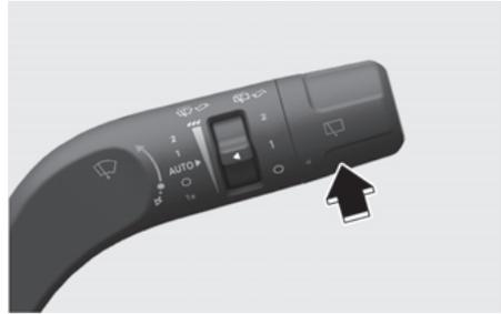
Push the lever away from you to spray rear washer fluid and to run the rear wipers 1-3 cycles. The spray and wiper operation continues until you release the lever.
