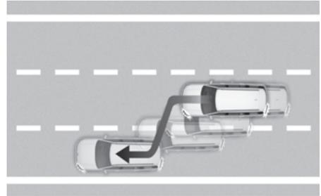
Highway Lane Change Assist function helps change lanes to the direction you operate the turn signal switch if the function judges that lane change is possible.
