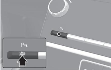
Press and hold the Parking Safety (PVA) button more than 2 seconds, to turn the Parking Collision-Avoidance Assist on or off.
