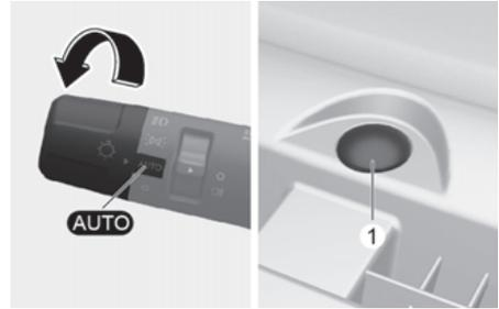
The position light and headlight are turned ON or OFF automatically depending on the amount of daylight as measured by the ambient light sensor (1) in front of the instrument panel.
