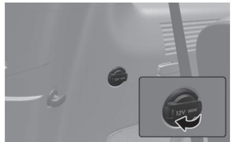
The power outlet is designed to provide power for mobile phones or other devices designed to operate with vehicle electrical systems.
