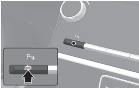
Press the Parking Safety (P<sub>WA</sub>) button to turn on Forward/Reverse Parking Distance Warning. Press the button again to turn off the function.
