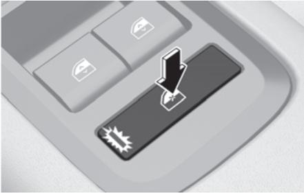
The driver can disable the power window switches on the rear passenger doors by pressing the power window lock button.
