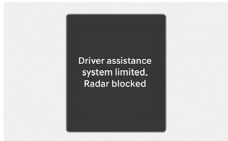
When the rear bumper around the rear-side radar or sensor is covered with foreign material, such as snow or rain, or installing a trailer or carrier, it can reduce the detecting performance and temporarily limit or disable Rear Cross-Traffic Collision-Avoidance Assist. If this occurs, the "**Driver assistance system limited. Radar blocked.**" warning message appears on the instrument cluster.
