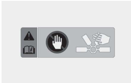
Do not put your hand near the cooling fan in the motor compartment whilst charging. It may operate automatically to control the battery temperature, even if the vehicle is turned off.
