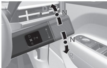
To shift the gear to N (Neutral), rotate the rotary gear shift dial to N (Neutral) from R (Reverse) or D (Drive) whilst depressing the brake pedal.
