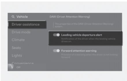
If **Leading vehicle departure alert** is enabled, the function informs the driver when a detected vehicle in front departs from a stop.
