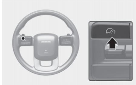
Press the Driving Assist button to turn Cruise Control off. The Cruise (
