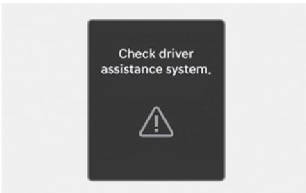
When Lane Following Assist is not working properly, the "**Check driver assistance system**" warning message will appear on the instrument cluster for several seconds, and the master (⚠) warning light appears on the instrument cluster. If this occur, we recommend that your vehicle be inspected by a HYUNDAI authorised repairer.
