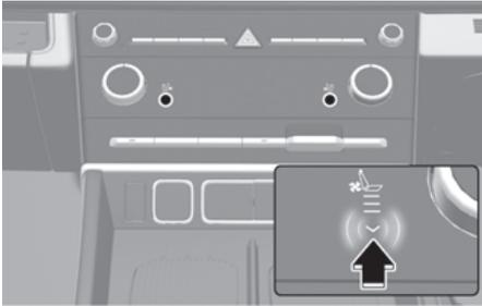
Whilst the engine is running, touch the icon to cool the driver's seat or front passenger's seat.
