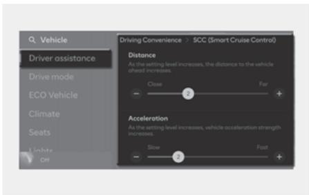
With the vehicle on, select **Settings > Vehicle > Driver assistance > Driving convenience > SCC (Smart Cruise Control)** from the settings menu in the infotainment system to change Distance, Acceleration, Response speed manually.
