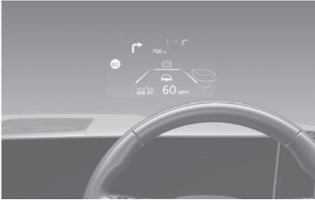
The Head-up display is an optional feature that allows the driver to view information projected onto a transparent screen whilst still keeping your eyes on the road ahead whilst driving.
