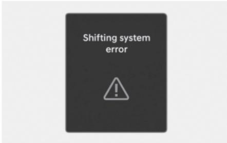
This message appears when the transmission or the shift dial does not properly operate in the P (Park) position. We recommend that your vehicle be inspected by a HYUNDAI authorised repairer.
