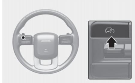
Press the Driving Assist (DRIVE ASSIST) button to turn Manual Speed Limit Assist off. The Speed Limit (LIMIT) indicator will go off. Always press the Driving Assist (DRIVE ASSIST) button to turn Manual Speed Limit Assist off when not in use.
