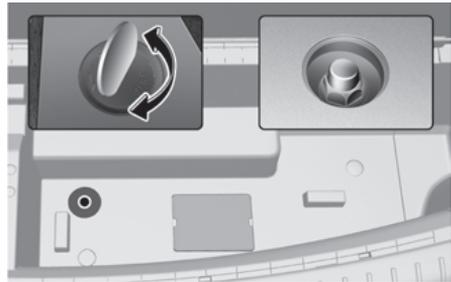
3. Connect the wheel lug nut wrench (A) to the bolt.
