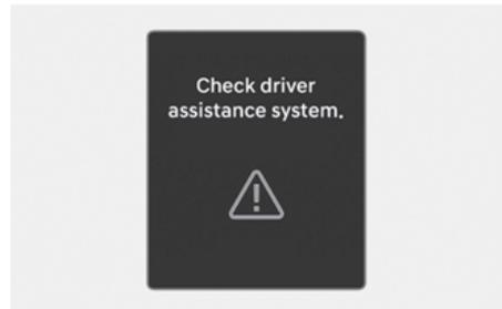
When Highway Driving Assist is not working properly, the "**Check driver assistance system**" warning message and yellow Lane Keeping Assist (
