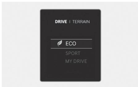
The mode changes, as the following, whenever the DRIVE/TERRAIN button is pushed up or down.
