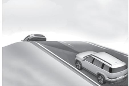
During uphill or downhill coasting, the smart regeneration system may not detect a moving vehicle in your lane, and cause your vehicle to accelerate. Also, your vehicle speed decelerates when a vehicle ahead is detected suddenly. Apply the brake pedal or accelerator pedal depending on the road and driving conditions.
