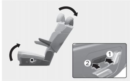
Press the rear portion of the Relaxation mode switch (1) for more than 0.5 seconds.
