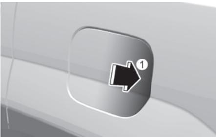
6. Pull the fuel filler door out to fully open.
