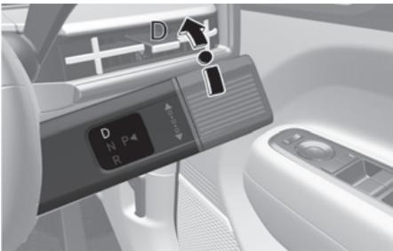
To shift the gear D (Drive), rotate the rotary gear shift dial to D (Drive) whilst depressing the brake pedal.
