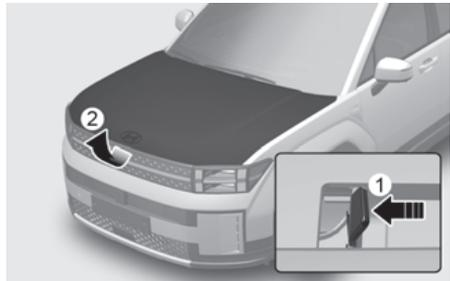
3. Go to the front of the vehicle, raise the bonnet slightly, push up the secondary bonnet release lever (1) inside of the bonnet centre and lift the bonnet (2). After the bonnet has been lifted halfway, it will raise completely by itself.
