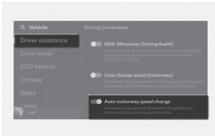
With the vehicle on, select **Settings > Vehicle > Driver assistance > Driving Convenience > Auto motorway speed change** from the Settings menu to turn on Navigation-based Smart Cruise Control and deselect to turn off the function.
