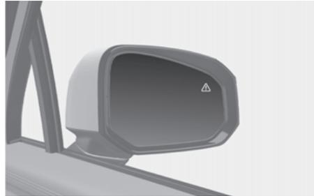
To warn the driver a vehicle is detected, the warning light on the outside rearview mirror and head-up display will illuminate.
