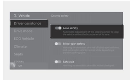
With the vehicle on, select **Settings** > **Vehicle** > **Driver assistance** > **Driving safety** > **Lane safety** from the settings menu in the infotainment system to set whether to use each function.
