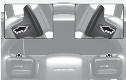
The paddle shifter is available when the gear is in the D (Drive) position in SPORT and TERRAIN (if equipped) mode.
