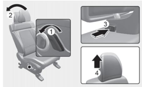
To remove the head restraint:
