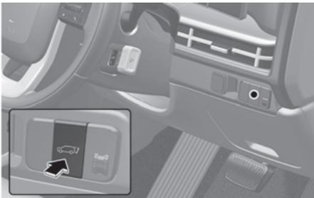
When the tailgate is closed, press the power tailgate open/close button for 1 second. The tailgate will open with a warning sound.
