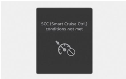
If the Driving Assist button, + switch, - switch or
