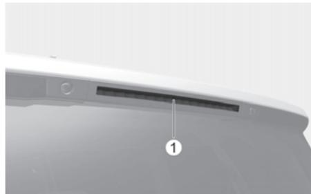
If the LED light (1) does not operate, we recommend that the system be inspected by a HYUNDAI authorised repairer.
