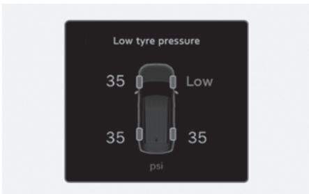
When the tyre pressure monitoring system warning indicator (⚠) is illuminated and a warning message appears on the cluster display, one or more of your tyres is significantly under-inflated. The Low Tyre Pressure Position Telltale will indicate which tyre is significantly under inflated by illuminating the corresponding position light.
