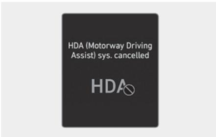
If the driver still does not have their hands on the steering wheel after the hands-off warning, **"HDA(Motorway Driving Assist) system cancelled"** warning message will appear and Highway Driving Assist and Lane Change Assist will be automatically cancelled.
