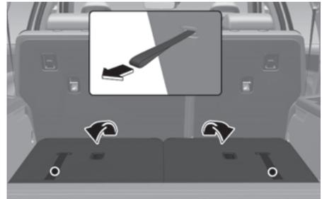
When using it as a seat, pull the seatback angle adjustment strap to fully raise the seatback. Adjust the seatback to the desired angle, and release the upper angle adjustment strap to lock in place. Make sure the seatback is locked in place.
