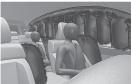
Side, curtain airbags and the front centre side airbag are designed to inflate when an impact is detected by side collision sensors depending on the severity of impact resulting from a side impact collision.
