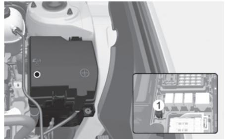
5. Pull the suspected fuse straight out. Use the removal tool (1) provided in the engine compartment fuses panel cover.
