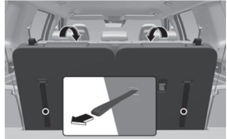
Pull the seatback angle adjustment strap to completely fold the seatback forward. Make sure the seatback is securely locked in place.
