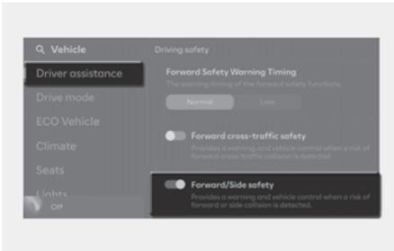
With the vehicle on, select or deselect **Settings > Vehicle > Driver assistance > Driving safety > Forward/Side safety** from the Settings menu to turn on or off Lane-Change Oncoming function, Lane-Change Side function, and Evasive Steering Assist function.
