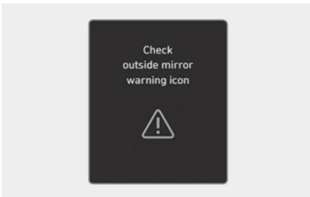
When the outside rearview mirror warning light is not working properly, the "**Check outside mirror warning icon**" warning message will appear on the instrument cluster for several seconds, and the master (⚠) warning light will appear on the instrument cluster. If this occurs, we recommend that your vehicle
