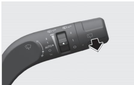
In the O (OFF) position, pull the lever gently toward you to spray washer fluid on the windscreen and to run the wipers 1-3 cycles. The spray and wiper operation continues until you release the lever. If the washer does not work, you may need to add washer fluid to the washer fluid reservoir.
