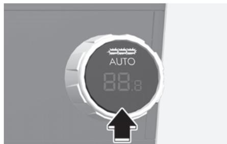
In automatic mode, press the AUTO button to select the fan speed from level 1 to 3.
