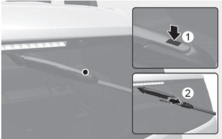
3. Lift off the wiper arm by pressing the blade home (1).
