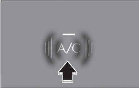
Press the A/C button to manually turn on the system on (indicator light ON) and off.
