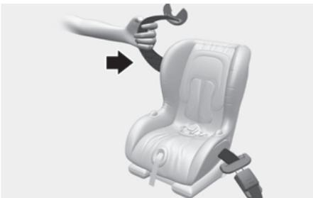
4. Push and pull on the Child Restraint System to confirm that the seat belt is holding it firmly in place.
