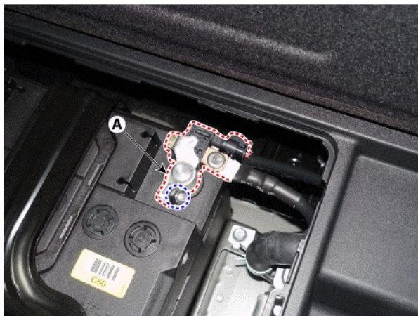
3-3. Turn the ignition switch OFF and disconnect the auxiliary 12V battery negative (-) terminal (A).
