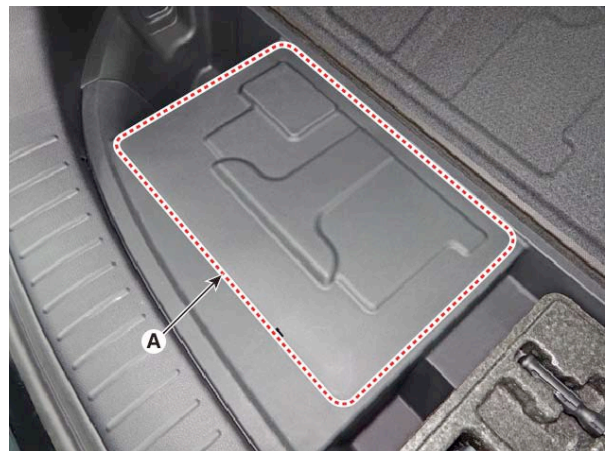
3-2. Remove the 12V battery service cover (A).
