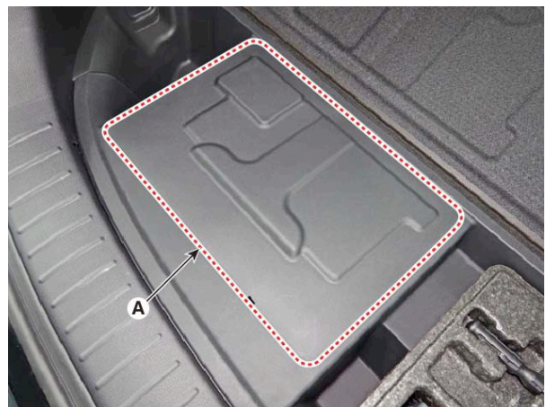
4-2. Remove the 12V battery service cover (A).
