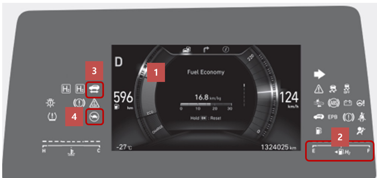
4 : Power Down Warning Light indicates that there may be a malfunction with the fuel cell stack. It comes on during driving the vehicle power should be limited due to a malfunction with fuel cell stack.
