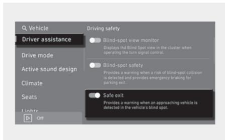
With the vehicle on, press the **SETUP** button, and then select **Driver assistance** > **Driving safety** > **Safe exit** in the infotainment system to turn on Safe Exit Warning and deselect to turn off the function.
