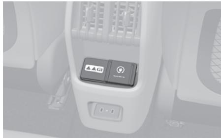
V2L(Vehicle to Load) is installed at the central rear seat. V2L is a convenient feature which provides enough electricity to use diverse household electrical appliances in the vehicle.
