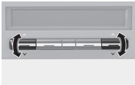
Push up the switch to increase the temperature. Push down to decrease the temperature.
