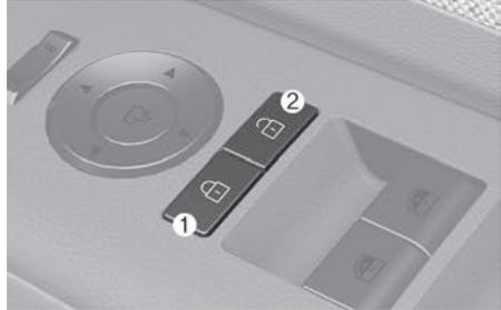
When pressing the
