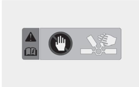
When using the V2L, the cooling fan in the vehicle motor compartment can operate automatically even if the vehicle is turned off. Do not put your hand near the cooling fan in the V2L operating state.
