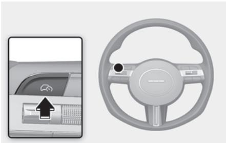
1. Press the Driving Assist (
