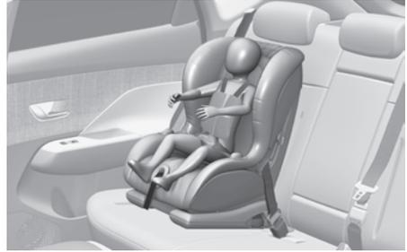
A forward-facing Child Restraint System provides restraint for the child's body with a harness. Keep children in a forward-facing Child Restraint System with a harness until they reach the top height or weight limit allowed by your Child Restraint System's manufacturer. Once your child outgrows the forward-facing Child Restraint System, your child is ready for a booster seat.
