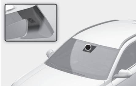
The Auto defogging reduces the likelihood of fogging up the inside of the windshield by automatically sensing moisture on inside of the windshield. The Auto defogging system operates when the heater or air conditioning is on.
