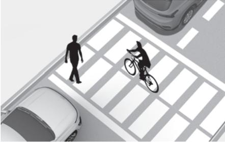
If there is a pedestrian(s) or bicycle(s) in between you and the vehicle in front, Leading Vehicle Departure Alert may not operate properly.
