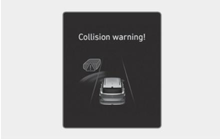
Whilst Smart Cruise Control is operating, when the collision risk with the vehicle ahead is high, the 'Collision Warning' warning message will appear on the instrument cluster, and an audible warning will sound to warn the driver. Always have your eyes on the road whilst driving, and if necessary, depress the brake pedal to reduce your driving speed in order to maintain a safe distance.
