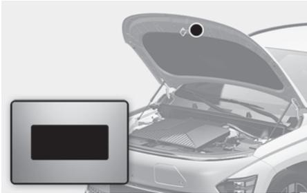
You can find out which air conditioning refrigerant is applied to your vehicle on the label located inside of the bonnet.
