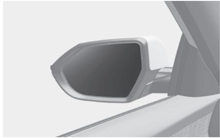
Your vehicle is equipped with both left-hand and right-hand rearview mirrors. The mirrors can be adjusted with the mirror adjustment control switch. Adjust the rearview mirrors to your desired position before driving. The rearview mirrors can be folded to help prevent damage when going through an automatic car wash or when passing through a narrow street.
