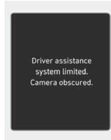
When the front windscreen where the front view camera is located, front radar cover, bumper (if equipped) or sensor is covered with foreign material, such as snow or rain, it can reduce the detecting performance and temporarily limit or disable Forward Collision-Avoidance Assist.
