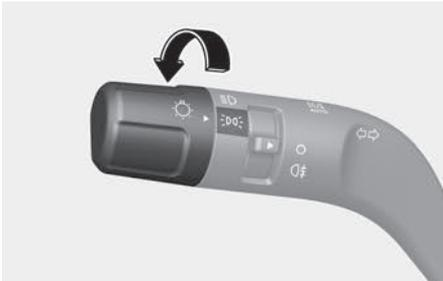
The position light, number plate light, and instrument panel lamp are turned ON.
