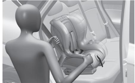
If your Child Restraint System manufacturer instructs or recommends you to use a top tether anchorage with the lap/shoulder belt, refer to "Securing a Child Restraint System seat with Top Tether Anchorage system" section for more information.
