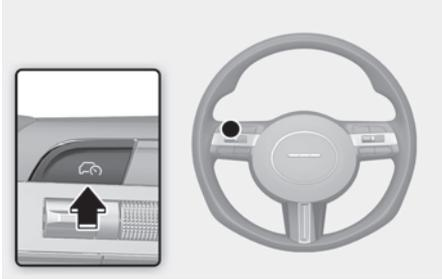
To turn Smart Cruise Control off, press the Driving Assist (DRIVE ASSIST) button.
