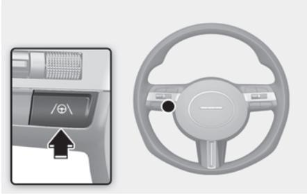
With the vehicle on, shortly press the Lane Driving Assist button located on the steering wheel to turn on Lane Following Assist. The grey or green (⊕) indicator light will appear on the cluster.
