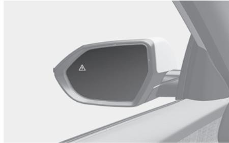
To warn the driver a vehicle is detected, the warning light on the side view mirror illuminates. Vehicle detection operates under following conditions.
