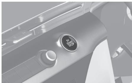
Whenever the front door is opened, the Start/Stop button illuminates and goes off for a few seconds after the door is closed.
