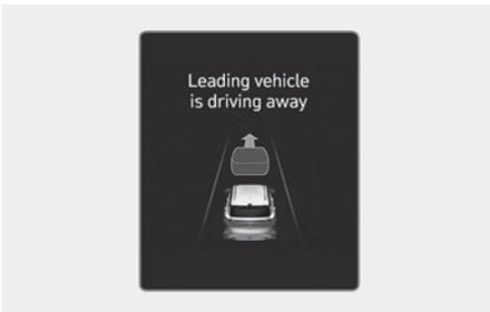
When a detected vehicle in front departs from a stop, Leading Vehicle Departure Alert will inform the driver by displaying the "**Leading vehicle is driving on**" message on the instrument cluster and an audible warning will sound.
