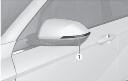
If the side repeater light (1) does not operate, we recommend that the system be inspected by a HYUNDAI authorised repairer.
