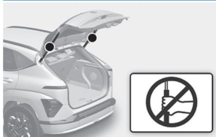
Always close the tailgate before driving. Do not grab or hold on to the tailgate support struts or they may be damaged. Deformation of the tailgate support struts may result in vehicle damage and personal injury.
