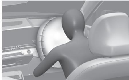
Upon deployment, tear seam in the pad cover separates from the expansion of the airbags.
