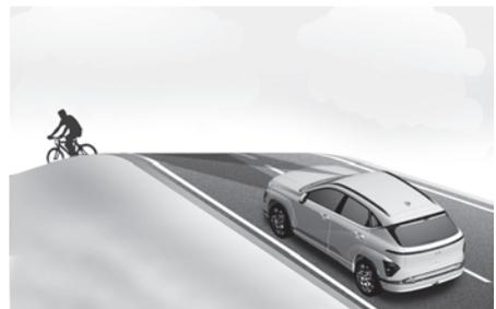
Forward Collision-Avoidance Assist may not detect other vehicles, powered two-wheelers, pedestrians or cyclists in front of you whilst driving uphill or downhill, adversely affecting the performance of the sensors.
