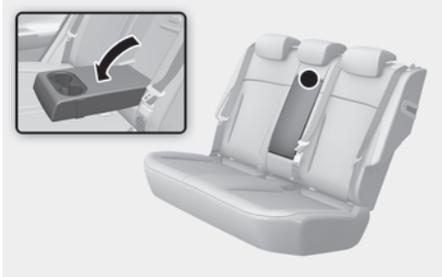
The armrest is located in the centre of the rear seat. Pull the armrest down from the seatback to use it.
