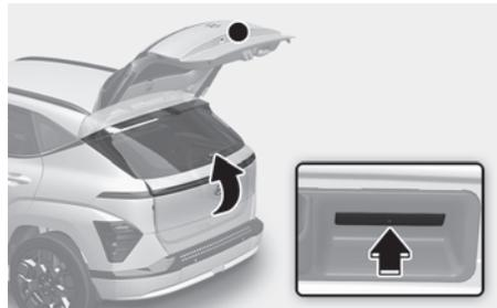
When the tailgate is closed, press the power tailgate open/close button to open the tailgate.
