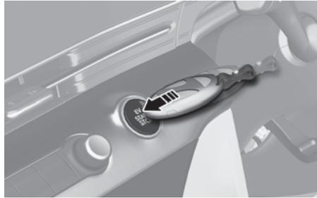
If the smart key battery is weak or the smart key does not work correctly, you can start the vehicle by pressing the Start/Stop button with the smart key in the direction of the picture above.
