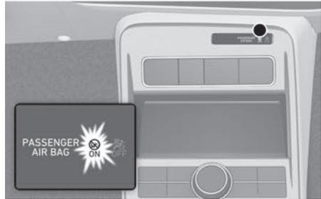
Insert the key or a similar rigid device into the passenger's front airbag ON/OFF switch and turn it to the ON position [A]. The passenger airbag ON indicator (⊗) illuminates.
