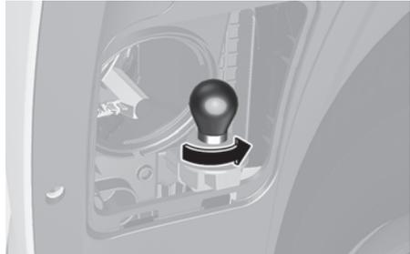
6. Install a new bulb and reinstall in the reverse order.
