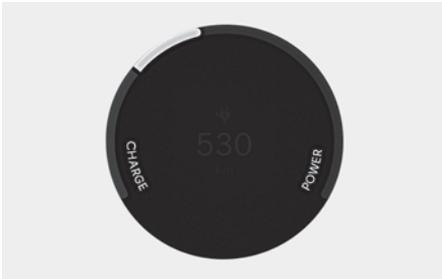
The Power/Charge Gauge shows the energy consumption rate of the vehicle and the charge/discharge status of the regenerative brakes.
