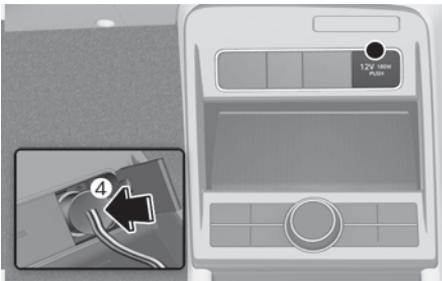
5. Make sure the compressor is turned off and plug the compressor power cord (4) into the vehicle power outlet.
