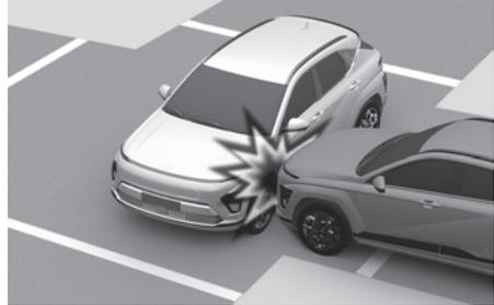
Front airbags may not inflate in side impact collisions, because occupants move in the direction of the collision. Side and curtain airbags may inflate depending on the severity of impact.
