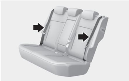
4. Pull up the seatback folding lever, then fold the each seat toward the front of the vehicle.
