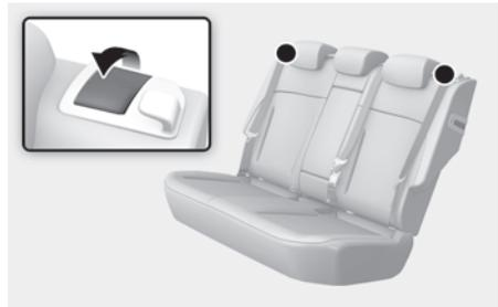
5. Pull up and hold the lever located behind the seatback and fold it forward.
