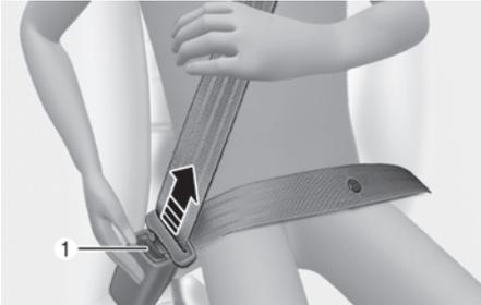
Once released, the belt should automatically draw back into the retractor. If this does not happen, check the belt to be sure it is not twisted, then try again.
