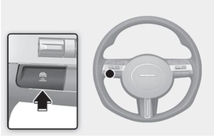
Press the button repeatedly to cycle through the headway settings from **Distance 4** → **Distance 3** → **Distance 2** → **Distance 1** → **Distance 4**.
