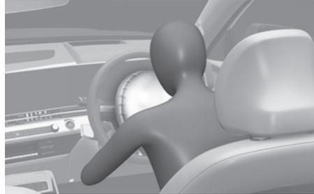
When the SRSCM detects a sufficiently severe impact to the front of the vehicle, it automatically deploys the front airbags.
