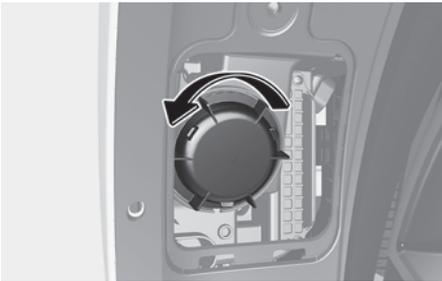
5. Remove the bulb from the socket by pushing it in and rotating it counterclockwise.
