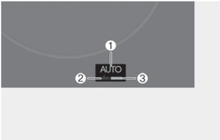
The instrument cluster displays 'AUTO' (1) when the smart regeneration system is ON. Depending on the conditions, the system adjusts the regenerative braking level (2). The sky blue indicator light (3) illuminates when the vehicle recognises a vehicle.
