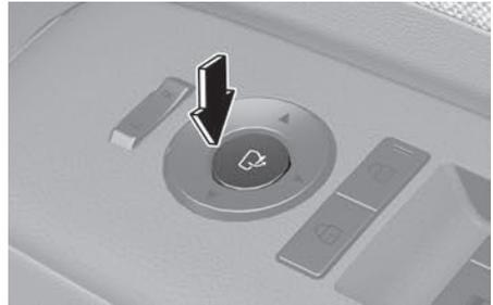
The rearview mirrors can be folded or unfolded by pressing the button.
