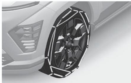
Since the sidewalls of radial tyres are thinner than other types of tyres, they may be damaged by mounting some types of tyre chains on them. Therefore, the use of snow tyres is recommended instead of tyre chains. If tyre chains must be used, use genuine HYUNDAI Parts and install the tyre chains after reviewing the instructions provided with the tyre chains. Damage to your vehicle caused by improper tyre chain use is not covered by your vehicle manufacturer's warranty.
