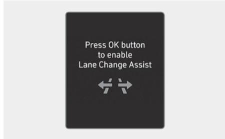
Whilst Highway Lane Change Assist function is on, the function will be ready to operate when all the following conditions are satisfied:
