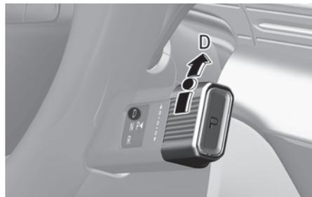
To shift the gear to D (Drive), rotate the rotary gear shift dial to D (Drive) whilst depressing the brake pedal.
