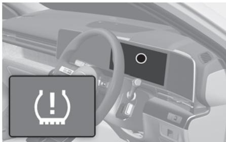
The TPMS malfunction indicator (⚠) illuminates after blinking for about 70 seconds when there is a problem with the Tyre Pressure Monitoring System.
