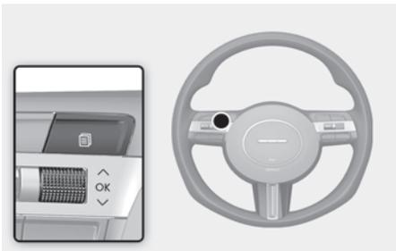
3. Select **Tyre Pressure** on the cluster by using the **^**, **v** (UP, DOWN) switch.
