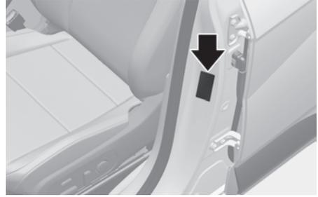
The vehicle certification label attached on the driver's (or front passenger's) side centre pillar gives the vehicle identification number (VIN).
