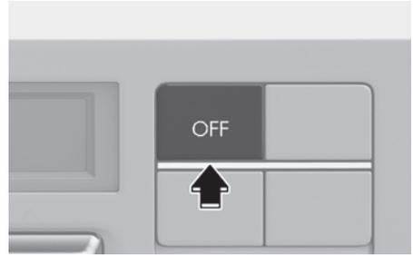
Press the **OFF** button to turn the climate control system off. You can still operate the mode and air intake buttons as long as the Start/Stop button is in the ON position.
