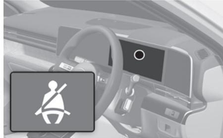
As a reminder to the driver, the driver's seat belt warning lights illuminates for about 6 seconds each time the Start/Stop button is in the ON position regardless of seatbelt fastening.
