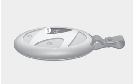
You can start the vehicle using the Remote Start button of the smart key.
