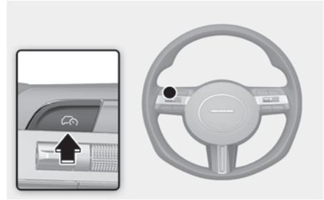
Press the Driving Assist (
