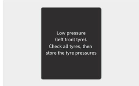
When the Low Tyre Pressure warning light (⚠) illuminates and a warning message appears on the cluster for 10 seconds, one or more of your tyres is significantly under-inflated.
