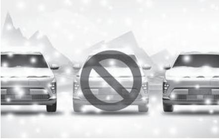
Snow may interfere with sensor operation, or Remote Smart Parking Assist may cancel if the road is slippery whilst parking.
