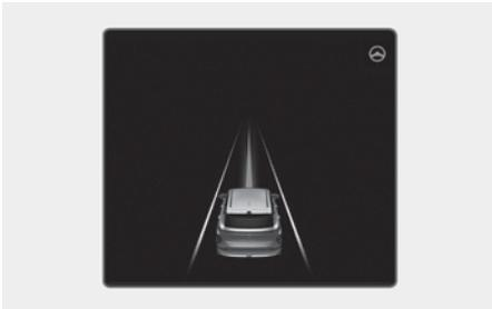
If the vehicle ahead and/or both lane markings are detected and your vehicle speed is below 120 mph (200 km/h), the green (⊕) indicator light appears on the cluster, and Lane Following Assist helps centre the vehicle in the lane by assisting the steering wheel.
