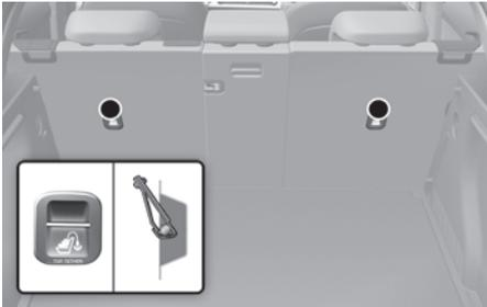
First secure the child restraint with the ISOFIX anchorages or the seat belt. If the child restraint manufacturer recommends that the top tether strap be attached, attach and tighten the top tether strap to the top tether strap anchorage.
