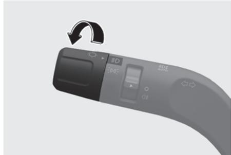
The headlight, position light, number plate light and instrument panel lamp are turned ON.
