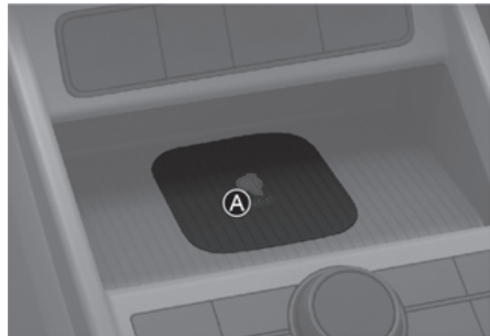
[A] Vehicle authentication pad (Wireless charging pad)
