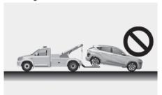
Do not tow vehicles with sling-type equipment. Only use wheel lift or flatbed equipment.
