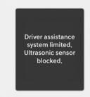
If this occurs the "Driver assistance system limited. Ultrasonic sensor blocked." warning message appears on the instrument cluster. Parking Distance Warning operates properly when snow, rain or foreign material is removed.
