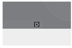
The automatic transmission shift indicator in the lower portion of the cluster display indicates the current gear or P (Park).
