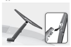
4. If the replacement is complete, put down the wiper arm onto the rear windscreen, and turn the vehicle ON and operate the wipers to check the blade is installed correctly.
