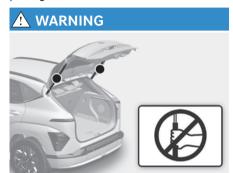
Always close the tailgate before driving. Do not grab or hold on to the tailgate support struts or they may be damaged. Deformation of the tailgate support struts may result in vehicle damage and personal injury.
