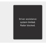
When the rear bumper around the rear corner radar or sensor is covered with foreign material, such as snow or rain, or installing a trailer or carrier, it can reduce the detecting performance and temporarily limit or disable Blind-Spot Collision-Avoidance Assist.
