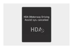
If the driver still does not have their hands on the steering wheel after the hands-off warning, "HDA (Motorway Driving Assist) sys. cancelled" warning message will appear and Highway Driving Assist and Lane Change Assist will be automatically cancelled.
