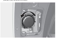
Remove the bulb from the socket by pushing it in and rotating it counterclockwise.
