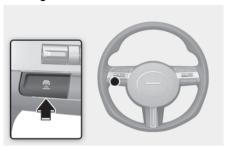
Press the button repeatedly to cycle through the headway settings from Distance  $4 \rightarrow$  Distance  $3 \rightarrow$  Distance  $2 \rightarrow$  Distance  $1 \rightarrow$  Distance  $4 \rightarrow$
