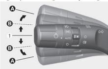
Highway Lane Change Assist function will operate, when you push the turn signal lever up or down to the A or B position whilst the function is in the ready state (indicator is green), and all of the following conditions are satisfied:
