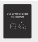
In traffic, your vehicle will stop if the vehicle ahead of you stops. Also, if the vehicle ahead of you starts moving, your vehicle will start as well. In addition, after the vehicle has stopped and a certain time have passed, the 'Use switch or pedal to accelerate' message will appear on the instrument cluster. Depress the accelerator pedal or operate the +, — or II'2 switch to start driving.
