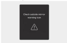
When the outside rearview mirror warning light is not working properly, the "Check outside mirror warning icon" warning message appears on the instrument cluster for several seconds, and the master (A) warning light illuminates on the cluster. If this occur, we recommend that your vehicle be inspected by a HYUNDAI authorised repairer.
