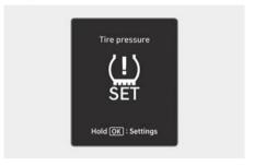
The tire pressure screen appears to reset the TPMS system.
