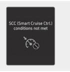
If the Driving Assist button, +, — or II'D switch is operated when Smart Cruise Control operating conditions are not satisfied, the "SCC (Smart Cruise Ctrl.) conditions not met" will appear on the cluster, and an audible warning will sound.
