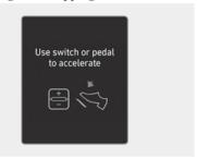
When Highway Driving Assist is operating, your vehicle will stop if the vehicle ahead of you stops. Also, if the vehicle ahead of you starts moving within 30 seconds after the stop, your vehicle will start as well. In addition, after the vehicle has stopped and 30 seconds have passed, the "Use switch or pedal to accelerate" message will appear on the instrument cluster. Depress the accelerator pedal or operate the + switch, — switch or II'D switch to start driving.
