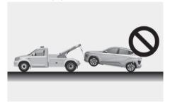
Do not lift using the trailer hitch or body and chassis part.
