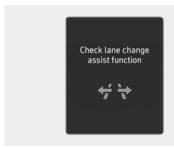
When Highway Driving Assist is not working properly, the "Check driver assistance system" and "Check lane change assist function" warning message and the master (△) warning light appears on the instrument cluster. If this occurs, we recommend that your vehicle be inspected by a HYUNDAI authorised repairer.
