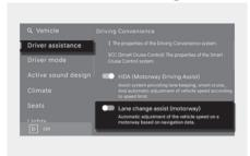
With the vehicle on, press the SETUP button, and then select Vehicle > Driver assistance > Driving Convenience > ALane change assist (motorway) in the infotainment system to turn on Navigation-based Smart Cruise Control and deselect to turn off the function.
