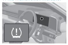
The TPMS malfunction indicator ((!)) illuminates after blinking for about 70 seconds when there is a problem with the Tyre Pressure Monitoring System.
