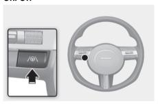
With the vehicle on, shortly press the Lane Driving Assist button located on the steering wheel to turn on Lane Following Assist. The grey or green (⊖) indicator light will appear on the cluster.
