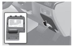
Refer to the label on the inside of the fuse panel cover to locate the suspected fuse location. 5. Pull the suspected fuse straight out. Use the removal tool provided in the motor compartment fuses panel cover.
