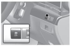
The Electronic Stability Control (ESC) system helps stabilize the vehicle during cornering manoeuvres.
