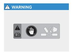
Keep hands, clothing, and tools away from the rotating fan blades of the cooling fan. The electric motor for the cooling fan may continue to operate or start up when the vehicle is off and can cause serious injury.
