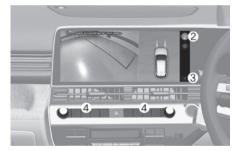
The front view appears on the screen when the gear is in N (Neutral) or D (Drive) to assist in parking.
