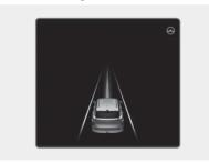
If the vehicle ahead and/or both lane markings are detected and your vehicle speed is below 120 mph (200 km/h), the green (②) indicator light appears on the cluster, and Lane Following Assist helps centre the vehicle in the lane by assisting the steering wheel.
