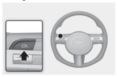
To turn Smart Cruise Control off, press the Driving Assist (←) button.
