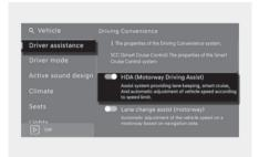
With the vehicle on, press the SETUP button and then select or deselect Vehicle > Driver assistance > Driving Convenience > HDA (Motorway Driving Assist) from the infotainment system to set whether to use each function.
