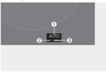
The instrument cluster displays 'AUTO' (1) when the smart regeneration system is ON. Depending on the conditions, the system adjusts the regenerative braking level (2). The sky blue indicator light (3) illuminates when the vehicle recognises a vehicle.
