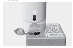
3. Make sure the compressor valve on the filling hose is locked.
