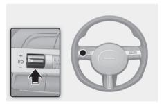
Press the **II 3** switch or depress the brake pedal to temporarily cancel Smart Cruise Control.
