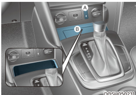
[A] : Indicator light, [B] : Charging pad
