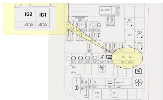
motor compartment fuse box
