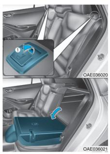
4.Pull on the seatback folding lever, then fold the seat toward the front of the vehicle.
