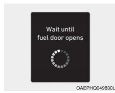
This message is displayed when you attempt to open the fuel filler door with the fuel tank pressurized. Wait until the fuel tank is depressurized.
