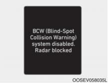
**BCW** (Blind-Spot Collision Warning) system disabled. Radar blocked
