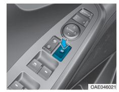
The driver can disable the power window switches on the rear passengers' doors by pressing the power window lock switch.
