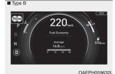
The cluster displays the speed limit information, overtaking restriction and conditional road sign.
