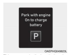
This message is displayed when the hybrid battery power (SOC) level is low.
