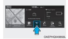
Press [PHEV] on the [Home] screen or the [All menus] screen and the menus related to plug-in hybrid ([ECO driving], [Energy information], [EV range], [Set charging times], [Charging stations], [Petrol stations]) are displayed.
