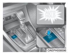
With the driver's door and engine hood closed, depress the brake pedal and then press the [AUTO HOLD] switch. The white AUTO HOLD indicator will come on and the system will be in the standby position.
