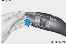
To turn on the high beam headlamp, push the lever away from you. The lever will return to its original position. The high beam indicator will light when the headlamp high beams are switched on.
