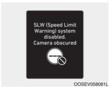
SLW (Speed Limit Warning) system disabled. Camera obscured
