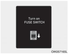
If the fuse switch is OFF, "Turn on FUSE SWITCH" message will appear.
