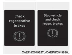
This warning message is displayed when the regenerative brake system does not work properly.
