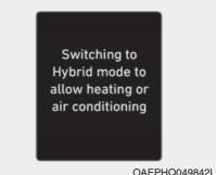
This message is displayed when the vehicle automatically switches to HEV mode to allow heating or air conditioning. It is when the coolant temperature is low (below -14°C) and the driver turns on the heating or cooling system.
