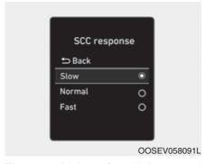
The sensitivity of vehicle speed when following the front vehicle to maintain the set distance can be adjusted.
