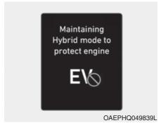
This message is displayed when the [HEV] button is pressed but it is impossible to switch from the HEV mode to EV mode due to engine lubrication.
