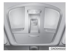
The sunroof can be opened, closed, or tilted when the ignition switch is in the ON position.
