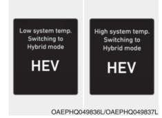
This message is displayed when the temperature of the high-voltage (hybrid) battery is too low or high. This warning message is to protect the battery and the hybrid system.
