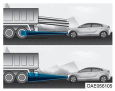
• Detecting the vehicle in front of you If the vehicle in front of you has cargo that extends rearward from the cab, or when the vehicle in front of you has higher ground clearance, additional special attention is required. The FCA system may not be able to detect the cargo extending from the vehicle. In these instances, you must maintain a safe braking distance from the rearmost object, and if necessary, depress the brake pedal to reduce your driving speed in order to maintain distance.
