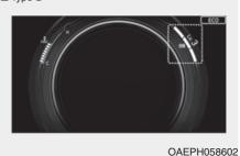
The selected regenerative braking level is displayed on the instrument cluster.
