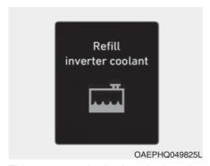
This message is displayed when the inverter coolant is nearly empty.
