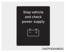
This message is displayed when a failure occurs in the power supply system.
