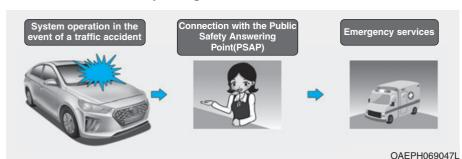
The Pan-European eCall device automatically makes an emergency call to the Public Safety Answering Point (PSAP) for proper rescuing operations in event of vehicle accident.
