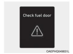
This message is displayed when there is a problem with the fuel filler door. Such as, when the fuel filler door does not open after 20 seconds at freezing temperature.
