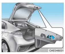
Lower the tailgate lid and press down until it locks. To be sure the tailgate lid is securely fastened, always check by trying to pull it up again.
