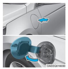
5. Press center edge of the charging door to open the charging door.
