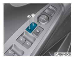
When pressing the  $(\mathbf{G})$  portion (1) of the switch, all vehicle doors will lock.
