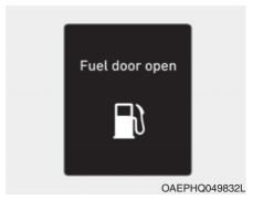
This message is displayed when the fuel filler door opens after the fuel tank is depressurized. If this message is displayed, you can refuel the fuel tank.
