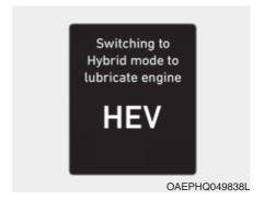
This message is displayed when the vehicle is automatically switched to the HEV mode to lubricate engine while the ignition switch is in the ON position.
