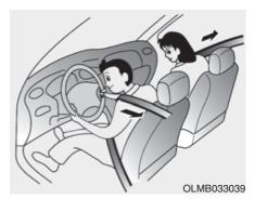
Your vehicle is equipped with driver's and front passenger's and rear passenger's (if equipped) Pre-tensioner Seat Belts (Retractor Pretensioner). The purpose of the pre-tensioner is to make sure the seat belts fit tightly against the occupant's body in certain frontal collisions. The pre-tensioner seat belts may be activated in crashes where the frontal collision is severe enough, together with the air bags.
