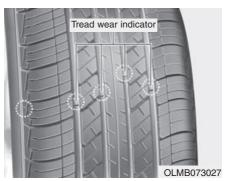
If the tire is worn evenly, a tread wear indicator will appear as a solid band across the tread. This shows there is less than 1.6 mm (1/16 in.) of tread left on the tire. Replace the tire when this happens.
