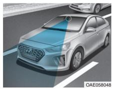
The Lane Following Assist (LFA) system helps detect lane markers on the road with a front view camera at the front windshield, and assists the driver's steering to help keep the vehicle between lanes.
