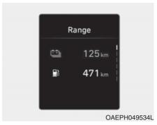
The range is the estimated distance the vehicle can be driven with the remaining fuel in the fuel tank (Gasoline/Petrol) and high-voltage (hybrid) battery (Electric).
