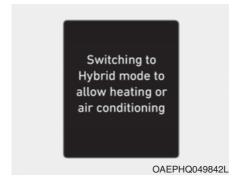
This message is displayed when the vehicle automatically switches to HEV mode to allow heating or air conditioning. It is when the coolant temperature is low (below -14°C) and the driver turns on the heating or cooling system.
