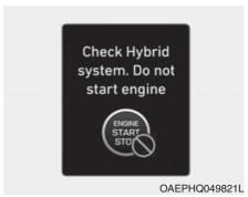
This message is displayed when the hybrid battery power (SOC) level is low. A warning chime will sound until the problem is solved.
