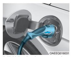
Hold the charging connector handle and connect it to the vehicle AC charging inlet. Push the connector until you hear a "clicking" sound. If the charging connector and charging terminal are not connected properly, this may cause a fire.
