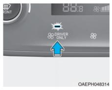
If you press the DRIVER ONLY button(\$\mathbb{G}^{\text{DRIVER}}\_{\text{ONLY}}) and the indicator light illuminates, air mostly blows in the direction of the driver's seat. However, some of the air may come out of other seating position ducts to keep indoor air pleasant.
