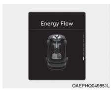
The hybrid system informs the drivers its energy flow in various operating modes. While driving, the current energy flow is specified in 11 modes.
