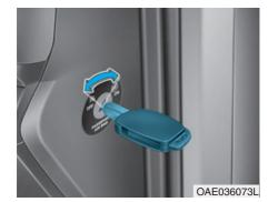
Passenger's front air bag ON/OFF switch (if equipped)
