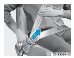
To release your seat belt: Press the release button (1) in the locking buckle.
