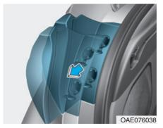
5. Remove the rear combination lamp assembly from the body of the vehicle.
