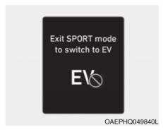
This message is displayed when [HEV] button is pressed but it is impossible to switch from the HEV mode to EV mode because the SPORT mode is engaged.
