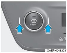
2. Press the temperature control button to set the desired temperature.
