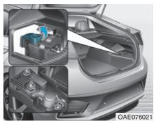
The electronic system may not function correctly even when the fuses located in the engine compartment and instrument panel are not disconnected. In such case, the cause of the problem may be disconnection of the main fuse (BFT type), which is located inside the positive battery terminal (+) cap. Since the main fuse is designed more intricately than other parts, we recommend you visit the nearest HYLINDAI dealer
