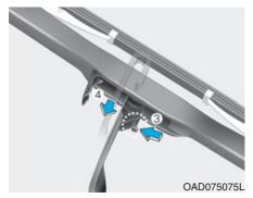
3. While pushing the lock (3), pull down the wiper blade (4).
