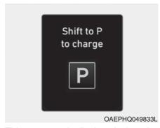
This message is displayed when the charging connector is plugged with the shift lever in R (Reverse), N (Neutral) or D (Drive). Move the shift lever to P (Park) and re-start the charging process.
