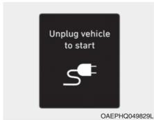
This message is displayed when you start the engine without unplugging the charging cable. Unplug the charging cable, and then start the vehicle.
