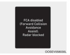
FCA disabled (Forward Collision Avoidance Assist). Radar blocked
