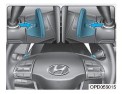
The paddle shifter is used to adjust the regenerative braking level from 0 to 3 when the vehicle is in ECO mode.
