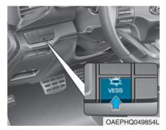
The Virtual Engine Sound System generates engine sound for pedestrians to hear vehicle sound because there is limited sound while motor power is used.
