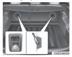
Top-tether anchorages for Child Restraint Systems are located on the rear of the seatbacks.
