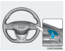
First, switch the mode to Cruise Control by pressing the MDDE button if equipped with the Speed Limit Control System.
