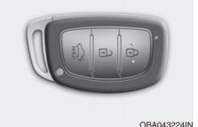
To lock the doors, press the button on the outside door handle while carrying the smart key with you or press the door lock button on the smart key. To unlock the doors, press the button on the outside door handle while carrying the smart key with you or press the door unlock button on the smart key.
