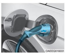
7. Hold the charging connector handle and connect it to the vehicle AC charging inlet. Push the connector until you hear a "clicking" sound. If the charging connector and charging terminal are not connected properly, this may cause a fire.
