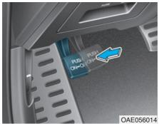
Check whether the stroke is within specification when the parking brake pedal is depressed with 20 kg (44 lb, 196 N) of force. Also, the parking brake alone should securely hold the vehicle on a fairly steep grade. If the stroke is more or less than specified, have the parking brake adjusted by an authorized HYUNDAI dealer.
