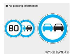
The symbol is displayed on the instrument cluster and the navigation, when the ISLW detects a noovertaking sign.
