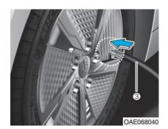
4. Unscrew the valve cap from the valve of the defective and screw the filling hose (3) of the sealant bottle onto the valve.
