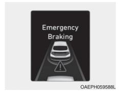
This warning message appears on the LCD display with a warning chime. Additionally, some vehicle system intervention occurs by the engine management system to help decelerate the vehicle.
