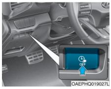
• If you press the scheduled charging deactivation (♣) button to immediately charge the battery, charging must be initiated 3 minutes after the charging cable has been connected. When you press the scheduled charging deactivation (♣) button for immediate charging, the scheduled charge setting is not completely deactivated. If you need to completely deactivate the scheduled charge setting, use the infotainment system to finalize the deactivation.
