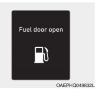
This message is displayed when the fuel filler door opens after the fuel tank is depressurized. If this message is displayed, you can refuel the fuel tank
