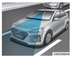
The Intelligent Speed Limit Warning (ISLW) system displays the speed limit information and overtaking restriction of the current road through the instrument cluster and the navigation. The ISLW reads the traffic signs through the camera, which is attached on the upper part of the inner front windshield.
