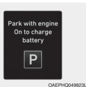
This message is displayed when the hybrid battery power (SOC) level is low.
