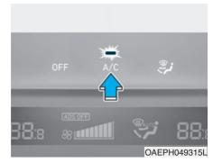
Push the A/C button to turn the air conditioning system on (indicator light will illuminate).
