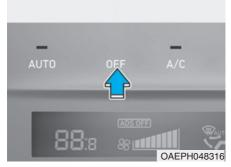
Push the OFF button to turn the climate control system off. However, you can still operate the mode and air intake buttons as long as the ignition switch is in the ON position.
