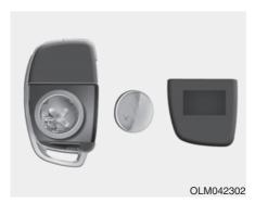
Battery Type: CR2032 To replace the battery:
