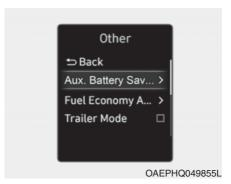
The driver can activate the Aux. Battery Saver+ function by placing the ignition switch to the ON position and by selecting:
