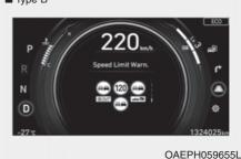
The driver can monitor the information provided from the ISLW system on the LCD display.
