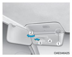
To use a sunvisor, pull it downward. To use a sunvisor for a side window, pull it downward, unsnap it from the bracket (1) and swing it to the side (2). To use the vanity mirror, pull down the sunvisor and slide the mirror cover (3). Use the ticket holder (4) to hold tickets.
