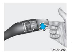
In the OFF (O) position, pull the lever gently toward you to spray washer fluid on the windshield and to run the wipers 1-3 cycles. The spray and wiper operation will continue until you release the lever. If the washer does not work, you may need to add washer fluid to the washer fluid reservoir.
