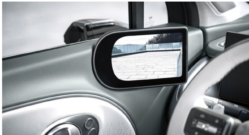
Door-mounted monitor of the Digital Side Mirror (DSM). (optional on Calligraphy trim)
