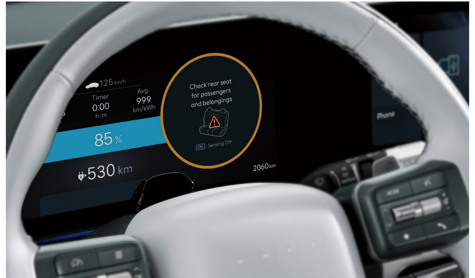
Rear Occupant Alert (ROA) alerts you to check rear seats upon leaving the vehicle.
