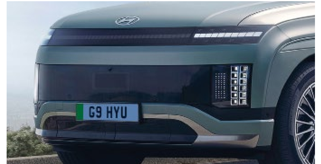
LED Daytime Running Lights with LED Small Cube Projection Headlamps.
