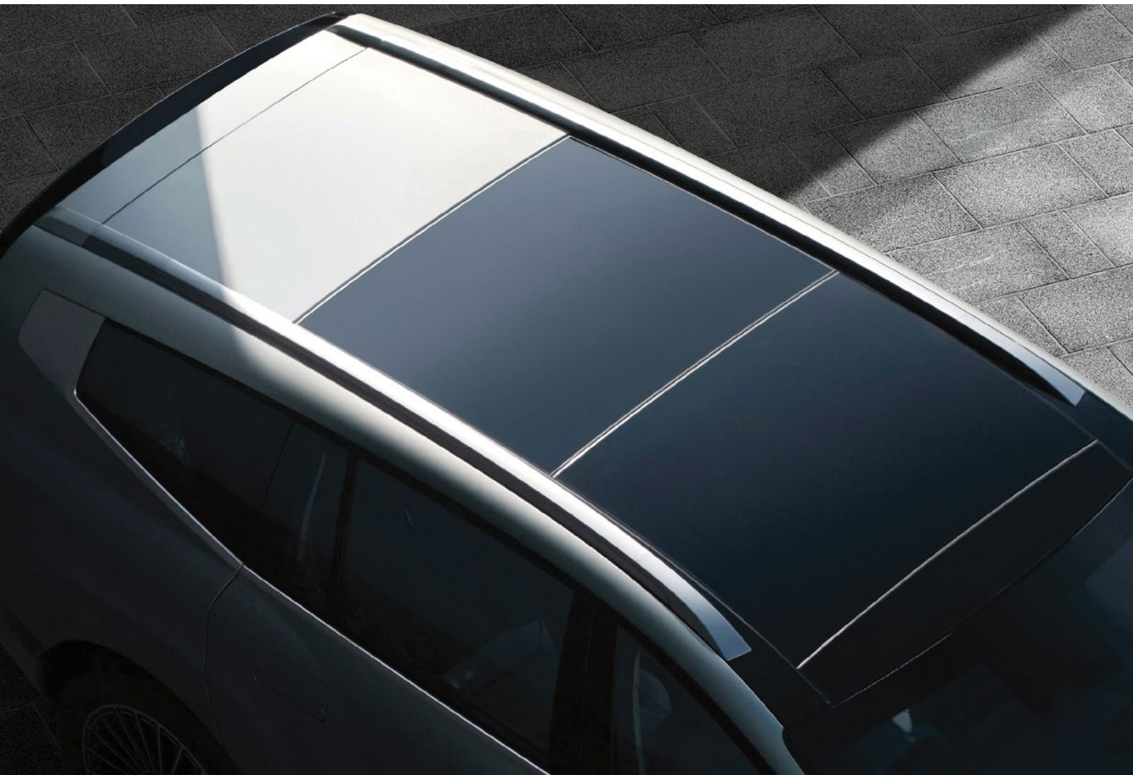
Aerodynamically optimized roof with hidden antennas and openable panoramic sunroof.
