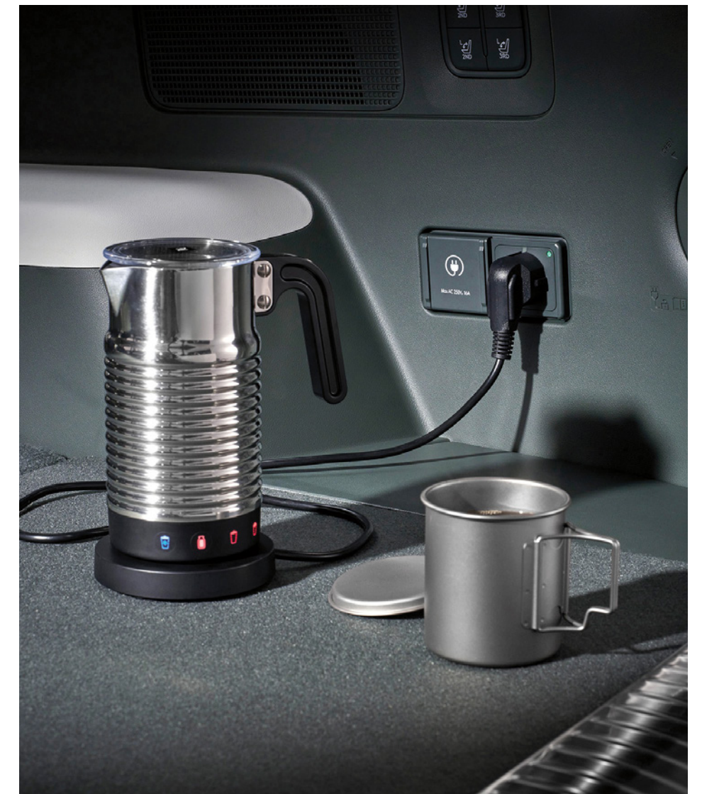
230V Vehicle-to-Load (V2L) socket in the boot.
