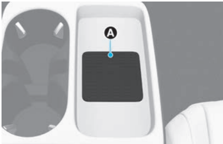
[A] Vehicle authentication pad (wireless charging pad)
