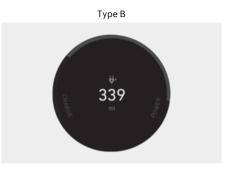
The distance to empty vary depending on many factors such as driving habits, power usage, driving conditions, and high voltage battery. The distance to empty may be increased or decreased than the certified figures as it reflects all the factors comprehensively. Check the distance to empty considering the following:
