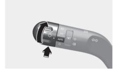
Hight Beam Assist automatically switches between high beam and low beam depending on the detected brightness from the lights of oncoming vehicles or vehicles in front.
