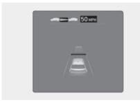
If you want to speed up temporarily without altering the set speed whilst Smart Cruise Control is operating, depress the accelerator pedal. Whilst the accelerator pedal is depressed, the set speed, distance level and target distance will blink on the cluster.
