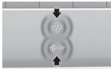
Press the \$\%\text{ button to increase fan speed} and airflow. Press the \$\%\text{or}\text{button to} decrease fan speed and airflow.
