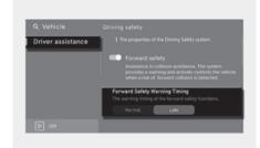
With the vehicle on, select Settings > Vehicle > Driver assistance > Driving safety > Forward Safety Warning Timing in the infotainment system to change the initial warning activation time for Forward Collision-Avoidance Assist. The warning time can be set to either "Normal" or "Late"
