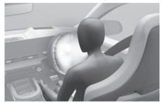
When the SRSCM detects a sufficiently severe impact to the front of the vehicle, it automatically deploys the front airbags.
