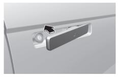
When all doors are closed, touch the touch sensor on the front outside door handle (the engraved part) whilst carrying the Smart Key with you, outside door handle will return and doors will be locked.
