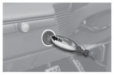
If the smart key battery is weak or the smart key does not work correctly, you can start the vehicle by pressing the Start/Stop button with the smart key in the direction of the picture above.
