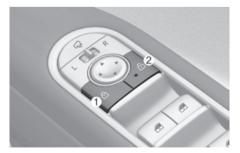
When pressing the  $\Box$  portion (1) on the button, all vehicle doors are locked.
