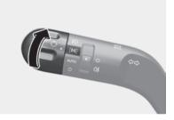
The position light, number plate light, and instrument panel lamp are turned ON.
