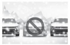
Snow may interfere with the operation of the ultrasonic sensor and wide view camera, or Remote Smart Parking Assist may cancel if the road is slippery whilst parking.
