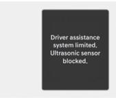
The "Driver assistance system limited. Camera obscured." or "Driver assistance system limited. Ultrasonic sensor blocked." warning message appears on the cluster if the following situations
