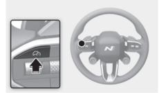
Press the Driving Assist ( ) button to turn Manual Speed Limit Assist off. The Speed Limit ( ) indicator will go off.
