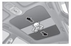
If the power sunshade senses any obstacle whilst it is closing automatically, it will reverse direction then stop at a certain position.
