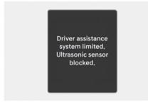
If this occurs the "**Driver assistance** system limited. Ultrasonic sensor blocked." warning message appears on the instrument cluster. Parking Distance Warning operates properly when snow, rain or foreign material is removed.
