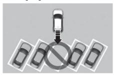
Remote forward function may not operate properly in a diagonal parking space.
