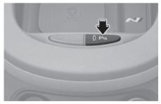
Press and hold the Parking Safety (Pm) button more than 2 seconds, 'Rear Active Assist' or to turn the Parking Collision-Avoidance Assist on or off.
