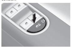
When the electronic child safety lock (a) button is in the LOCK position and an approaching vehicle from the rear area is detected, the electronic child safety lock button will not unlock even if the driver presses the button to prevent the rear doors from opening.
