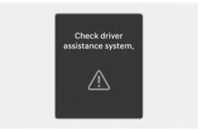
When Smart Cruise Control is not working properly, the "**Check driver assistance system.**" warning message and the master (**(**) warning light will appear on the instrument cluster. We recommend that your vehicle be inspected by a HYUNDAI authorised repairer.
