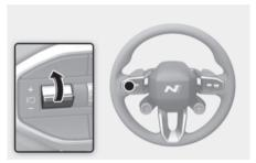
Push the + switch up and release it immediately. The set speed will increase by 1 mph (1 km/h) each time the switch is operated in this manner.  Push the + switch up and hold it whilst monitoring the set speed on the cluster. The set speed will increase by 5 mph (10 km/h) each time the switch is operated in this manner. Release the switch when the desired speed is shown, and the vehicle will accelerate to that speed. You can increase the set speed up to 120 mph (200 km/h).
