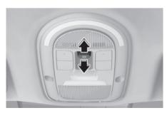
The power sunshade can only be operated when Start/Stop button is in the ON or START position.
