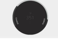
The Power/Charge Gauge shows the energy consumption rate of the vehicle and the charge/discharge status of the regenerative brakes.
