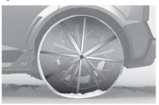
Since the sidewalls of radial tyres are thinner than other types of tyres, they may be damaged by mounting some types of tyre chains on them. Therefore, the use of snow tyres is recommended instead of tyre chains. If tyre chains must be used, use genuine HYUNDAI Parts and install the tyre chains after reviewing the instructions provided with the tyre chains. Damage to your vehicle caused by improper tyre chain use is not covered by your vehicle manufacturer's warranty.
