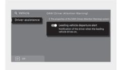
With the vehicle on, select or deselect Settings > Vehicle > Driver assistance > DAW (Driver Attention Warning) and then enable Leading vehicle departure alert in the infotainment system to set whether to use each function.
