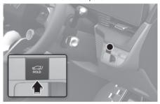
When the tailgate is closed, press the power tailgate open/close button for 1 second. The tailgate opens with a warning sound.
