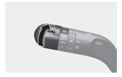
The headlight, position light, number plate light and instrument panel lamp are turned ON.
