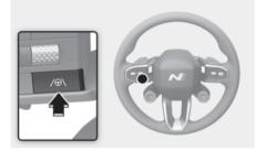
With the vehicle on, shortly press the Lane Driving Assist button located on the steering wheel to turn on Lane Following Assist. The grey or green  $(\Theta)$  indicator light will appear on the cluster.
