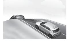
During uphill or downhill driving, the Smart Cruise Control may not detect a moving vehicle in your lane, and cause your vehicle to accelerate to the set speed. Also, vehicle speed will rapidly decrease when the vehicle ahead is detected suddenly.
