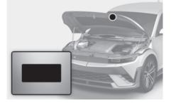
You can find out which air conditioning refrigerant is applied to your vehicle on the label located inside of the bonnet.
