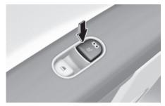
whilst the vehicle is running, press the seat warmer switch to warm the rear seat.
