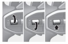
To resume Manual Speed Limit Assist after the function was paused, operate the +, -, || O switch.
