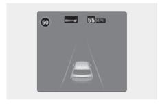
When driving at a speed higher than the displayed speed limit, the red speed limit indicator will blink and warning sounds.
