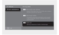
With the vehicle on, select **Settings** > **Driver assistance** > **Driving safety** > **Safe exit** in the infotainment system to turn on Safe Exit Warning and deselect to turn off the function.
