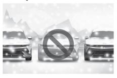
Snow may interfere with the operation of the ultrasonic sensor and wide view camera, or Remote Smart Parking Assist may cancel if the road is slippery whilst parking.
