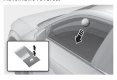
If a window senses any obstacle whilst it is closing automatically, it stops and lowers about 12 in. (30 cm) to allow the object to be cleared.
