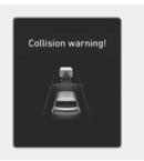
Whilst Smart Cruise Control is operating, when the collision risk with the vehicle ahead is high, the 'Collision Warning!' warning message will appear on the instrument cluster, and an audible warning will sound to warn the driver. Always have your eyes on the road whilst driving, and if necessary, depress the brake pedal to reduce your driving speed in order to maintain a safe distance.
