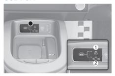
Press the USB port selection button whilst the vehicle is running. Press the upper portion of the button (1) to charge an electronic device. Press the lower portion of the button (2) to charge and listen to music with a media storage device. The USB port can be used after either indicator light turns on.
