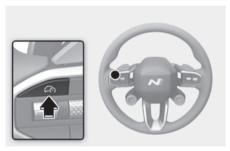
Press the Driving Assist ( ( ) button to turn Cruise Control off. The Cruise ( CRUISE) indicator will go off.
