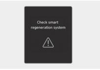
If the smart regeneration system is turned off due to the front radar being covered with foreign substances or due to other causes, the "Check Smart Regeneration System" warning message appears. Also the regenerative braking level is displayed instead of 'AUTO'.
