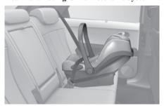
With a rearward-facing Child Restraint System, the collision forces are absorbed
