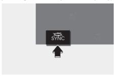
Adjusting the temperature, air flow direction, and fan speed equally
