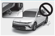
Never start or run the vehicle whilst an AWD vehicle is raised on a jack. The vehicle can slip or roll off of a jack causing serious injury or death to you or those nearby.
