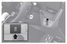
The Electronic Stability Control (ESC) system helps stabilize the vehicle during cornering manoeuvres.
