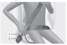
Pull the belt out of the retractor and insert the metal tab (1) into the buckle (2). There An audible "click" sounds when the tab locks into the buckle. Make sure the seat helt is not twisted
