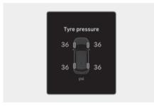
The tyre pressure screen appears to reset the TPMS system.
