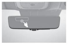
If the symbol shown in the image above is displayed when using the Digital Centre Mirror in digital mirror mode, the system may be malfunctioning. The symbol will disappear after a few seconds. Operate the lever, change to optical mirror mode and we recommend that you have the vehicle inspected by a HYUNDAI authorised repairer.
