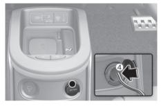
6. With the vehicle ON (READY indicator ON), switch on the compressor and let it run for about 5-7 minutes to fill the sealant up to proper pressure. (refer to the "Tyres and wheels" section in chapter 2). The inflation pressure of the tyre after filling is unimportant and will be checked/corrected later.
