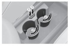
Push the button (1). The cup supporter protrudes from the front console.
