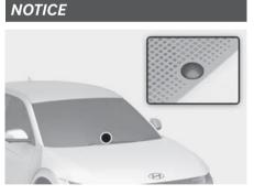
Never place anything near the sensor to ensure better control of the heating and cooling system.
