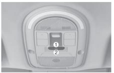
Elements of the Pan-European eCall system, installed in passenger compartment:
