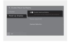
Head-up display can be enabled from the Settings menu in the infotainment system.
