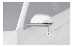
If the side repeater light (1) does not operate, we recommend that the system be inspected by a HYUNDAI authorised repairer.
