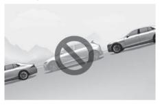
Park or exit manually when the vehicle is on inclines.
