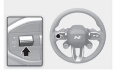
Press the **IID** switch to temporarily pause the set speed limit. The set speed limit will turn off but the Speed Limit (अנאוד) indicator will stay on.
