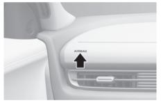
The SRS consists of airbags located in the centre of the steering wheel and the passenger's side front panel pad above the glove box.
