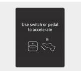
In traffic, your vehicle will stop if the vehicle ahead of you stops. Also, if the vehicle ahead of you starts moving, your vehicle will start as well. In addition, after the vehicle has stopped and a certain time have passed, the **'Use switch or pedal to accelerate**' message will appear on the instrument cluster. Depress the accelerator pedal or operate the **+**, **-** or **II'D** switch to start driving.
