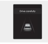
• When the vehicle is stopped due to emergency braking, the "**Drive carefully**" warning message will appear on the cluster.
