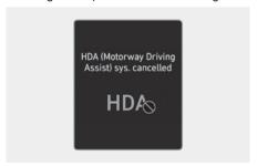
If the driver still does not have their hands on the steering wheel after the hands-off warning, "HDA (Motorway Driving Assist) sys. cancelled" warning message will appear and Highway Driving Assist and Lane Change Assist will be automatically cancelled.
