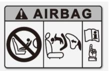
Never install a Child Restraint System in the front passenger seat, unless the airbag is deactived.
