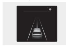
If the vehicle ahead and/or both lane markings are detected and your vehicle speed is below 120 mph (200 km/h), the green (♠) indicator light appears on the cluster, and Lane Following Assist helps centre the vehicle in the lane by assisting the steering wheel.
