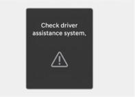
When Safe Exit Warning is not working properly, the "**Check driver assistance system.**" warning message will appear on the cluster for several seconds, and the master ( $\triangle$ ) warning light will appear on the cluster. If this occurs, we recommend that your vehicle be inspected by a HYUNDAI authorised repairer.
