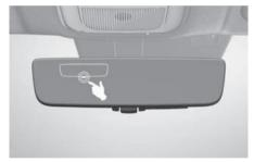
If the symbol shown in the image above is displayed when using the Digital Centre Mirror in digital mirror mode, the system may be malfunctioning. The symbol will disappear after a few seconds. Operate the lever, change to optical mirror mode and we recommend that you have the vehicle inspected by a HYUNDAI authorised repairer.
