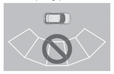
Remote Smart Parking Assist does not work properly when the parking lines are not parallel. Do not park although the parking space is recognised by the sensor.
