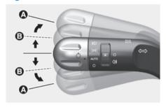
To signal a turn, push down on the lever for a left turn or up for a right turn in position [A].
