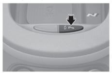
Press the Parking Safety (P<sub>1</sub>) button to turn on Forward/Reverse Parking Distance Warning. Press the button again to turn off the function.
