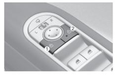
When pressing the 🗗 portion (1) on the button, all vehicle doors are locked.
