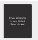
When the rear bumper around the rear-side radar or sensor is covered with foreign material, such as snow or rain, or installing a trailer or carrier, it can reduce the detecting performance and temporarily limit or disable Rear Cross-Traffic Collision-Avoidance Assist.
