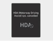
If the driver still does not have their hands on the steering wheel after the hands-off warning, "HDA (Motorway Driving Assist) sys. cancelled" warning message will appear and Highway Driving Assist and Lane Change Assist will be automatically cancelled.
