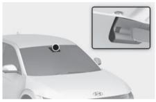
The Auto defogging reduces the likelihood of fogging up the inside of the windscreen by automatically sensing moisture on inside of the windscreen.
