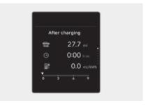
Trip distance, total driving time, average energy consumption, and instant energy consumption after the vehicle has been recharged are displayed. To reset manually, press the **OK** button on the steering wheel for more than 1 second when "**After charging**" appears.
