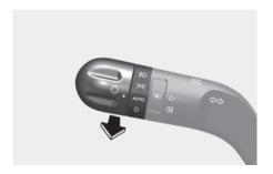
To flash the high beam headlight, pull the lever towards you, then release the lever. The high beams remain ON as long as you hold the lever.
