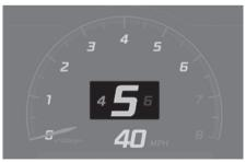
In the manual shift mode, this indicator informs which gear is desired whilst driving to save energy.
