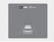
When Based on driving style is operating, the vehicle distance level and target distance will be displayed white based on the driving style.
