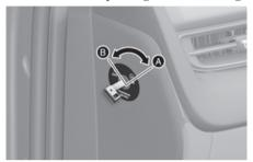
[A] Passenger airbag ON[B] Passenger airbag OFF
