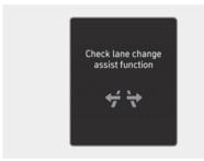
When Highway Driving Assist is not working properly, the "Check driver assistance system" and "Check lane change assist function" warning message and the master (△) warning light appears on the instrument cluster. If this occurs, we recommend that your vehicle be inspected by a HYUNDAI authorised repairer.
