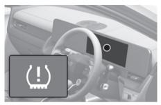
The TPMS Malfunction ((L)) Indicator illuminates after it blinks for about one minute when there is a problem with the Tyre Pressure Monitoring System.
