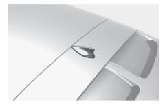
The shark fin antenna receives transmitted data (for example, AM/FM, SXM).
