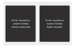
When the front windscreen where the front view camera is located, front radar cover, bumper (if equipped) or sensor is covered with foreign material, such as snow or rain, it can reduce the detecting performance and temporarily limit or disable Forward Collision-Avoidance Assist.
