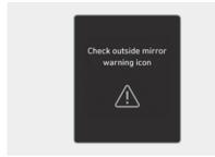
When the outside rearview warning light is not working properly, the "**Check outside mirror warning icon**" warning message will appear on the instrument cluster for several seconds, and the master (A) warning light will illuminate on the instrument cluster. If this occurs, we recommend that your vehicle be inspected by a HYUNDAI authorised repairer.
