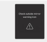
When the outside rearview mirror warning light is not working properly, the "Check outside mirror warning icon" warning message will appear on the cluster for several seconds, and the master (A) warning light will appear on the cluster. If this occurs, we recommend that your vehicle be inspected by a HYUNDAI authorised repairer.
