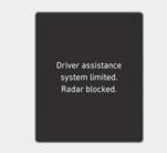
When the rear bumper around the rear corner radar or sensor is covered with foreign material, such as snow or rain, or installing a trailer or carrier, it can reduce the detecting performance and temporarily limit or disable Blind-Spot Collision-Avoidance Assist.
