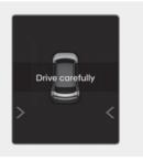
Brake control will end after the vehicle is stopped by emergency braking for about 2 seconds.
