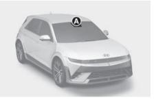
[A] Front view camera See the illustration above for the detailed location of the detecting sensor.
