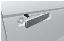
When all doors are closed, touch the touch sensor on the front outside door handle (the engraved part) whilst carrying the Smart Key with you, outside door
