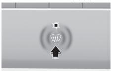
Press the front windscreen defroster button (indicator light ON) to turn on the front windscreen defroster. If the windscreen defogging is set, outside (fresh) mode is automatically selected and the air conditioning turns on according to the detected ambient temperature.
