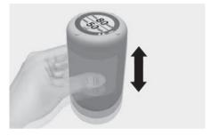
Remove the sealant bottle (2) cap and sealant bottle holder (5) cap and screw the bottle onto the sealant bottle holder.
