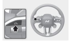
To turn Smart Cruise Control off, press the Driving Assist (द्रि) button.
