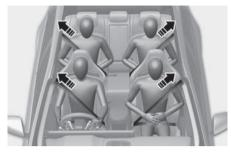
Your vehicle is equipped with driver's and front passenger's and rear passengers' (except rear centre seat) pretensioner seat belts (retractor pretensioner). The pretensioner makes sure the seat belts fit tightly against your body in certain frontal or side collision(s). The pretensioner seat belts may be activated in some crashes where the frontal or side collision(s) is severe enough, together with the airbags.
