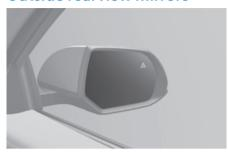
Your vehicle is equipped with both left-hand and right-hand rearview mirrors. The mirrors can be adjusted with the mirror adjustment control switch. Adjust the rearview mirrors to your desired position before driving. The rearview mirrors can be folded to help prevent damage when going through an automatic car wash or when passing through a narrow street.
