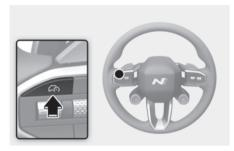
Press the Driving Assist (A) button to turn Manual Speed Limit Assist off. The Speed Limit (S) LIMIT) indicator will go off.
