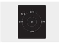
This mode displays the force delivered to the vehicle laterally whilst the vehicle is in motion.
