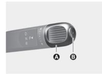
[A] Rotary gear shift dial[B] P button
