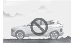
Remote Smart Parking Assist may cancel when the vehicle slips, or the vehicle cannot move due to road conditions such as pebbles or fragmented stones. • Parking behind a truck
