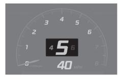
In the manual shift mode, this indicator informs which gear is desired whilst driving to save energy.
