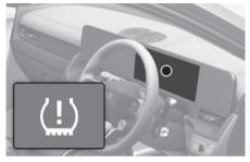
The TPMS Malfunction ((!)) Indicator illuminates after it blinks for about one minute when there is a problem with the Tyre Pressure Monitoring System.
