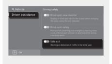
With the vehicle on, select **Settings** > **Driver assistance** > **Driving safety** > **Safe exit** in the infotainment system to turn on Safe Exit Warning and deselect to turn off the function.
