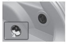
If the charging connector does not disconnect after pulling the emergency cable, we recommend that your vehicle be inspected by a HYUNDAI authorised repairer.
