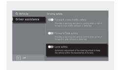
With the vehicle on, select **Settings** > **Vehicle** > **Driver assistance** > **Driving safety** > **Lane safety** in the infotainment system to set whether to use each function.
