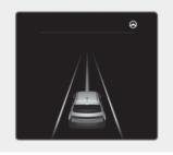
If the vehicle ahead and/or both lane markings are detected and your vehicle speed is below 120 mph (200 km/h), the green  $(\Theta)$  indicator light appears on the cluster, and Lane Following Assist helps centre the vehicle in the lane by assisting the steering wheel.
