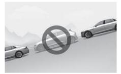
Park or exit manually when the vehicle is on inclines.
