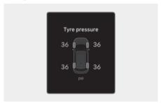
The tyre pressure screen appears to reset the TPMS system.
