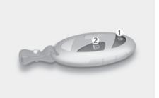
You can start the vehicle using the Remote Start button of the smart key.
