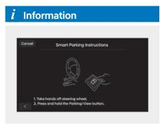
If Remote Smart Parking Assist cannot activate Remote Parking function, only the Smart Parking guide will be displayed on the infotainment system.
