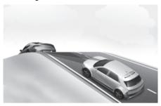
During uphill or downhill driving, the Smart Cruise Control may not detect a moving vehicle in your lane, and cause your vehicle to accelerate to the set speed. Also, vehicle speed will rapidly decrease when the vehicle ahead is detected suddenly.
