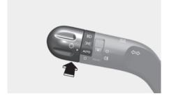
To turn on the high beam headlight, push the lever away from you. The lever returns to its original position.
