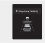
To warn the driver that emergency braking will be assisted, Forward Safety (♣) warning light blinking, the 'Emergency braking' warning message will appear on the instrument cluster, an audible warning will sound.
