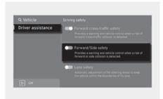
With the vehicle on, select **Settings** > **Vehicle** > **Driver assistance** > **Driving safety** > **Forward/Side safety** in the infotainment system to set whether to use each function.
