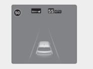
When driving at a speed higher than the displayed speed limit, the red speed limit indicator will blink and warning sounds.
