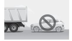
Do not use Remote Smart Parking Assist around vehicles with higher ground clearance, such as a bus, truck, etc. It may lead to an accident.
