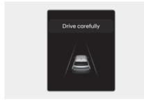
• When the vehicle is stopped due to emergency braking, the "**Drive carefully**" warning message will appear on the cluster.
