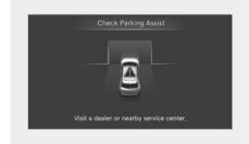
When Remote Smart Parking Assist is not working properly, the '**Check Parking Assist**' warning message will appear on the infotainment system. If the message appears, stop using Remote Smart Parking Assist, and we recommend that you have the vehicle inspected by a HYUNDAI authorised repairer.
