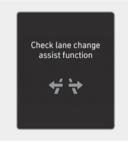
When Highway Driving Assist is not working properly, the "Check driver assistance system" and "Check lane change assist function" warning message and the master (A) warning light appears on the instrument cluster. If this occurs, we recommend that your vehicle be inspected by a HYUNDAI authorised repairer.
