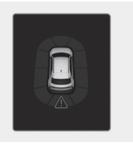
A master (A) warning light appears in the relative directions in case of a malfunction or blinding of the ultrasonic sensors while the Reverse Parking Collision-Avoidance Assist (PCA) is active. You can check the message in the utility information view of the instrument cluster.
