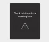
When the outside rearview mirror warning light is not working properly, the "Check outside mirror warning icon" warning message will appear on the instrument cluster for several seconds, and the master (A) warning light will appear on the instrument cluster. If this occurs, we recommend that your vehicle be inspected by a HYUNDAI authorised repairer.
