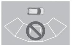
Remote Smart Parking Assist does not work properly when the parking lines are not parallel. Do not park although the parking space is recognised by the sensor. Inclined parking space
