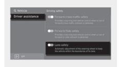
With the vehicle on, select **Settings** > **Vehicle** > **Driver assistance** > **Driving safety** > **Lane safety** in the infotainment system to set whether to use each function.
