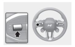
Press the IIO switch to temporarily pause the set speed limit. The set speed limit will turn off but the Speed Limit (©LIMIT) indicator will stay on.
