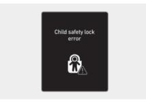
When electronic child safety lock does not work even though the button is pressed, the message will be displayed and an alarm will sound. If this occurs, we recommend that the vehicle be inspected by a HYUNDAI authorised repairer.
