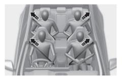
Your vehicle is equipped with driver's and front passenger's and rear passengers' (except rear centre seat) pretensioner seat belts (retractor pretensioner). The pretensioner makes sure the seat belts fit tightly against your body in certain frontal or side collision(s). The pretensioner seat belts may be activated in some crashes where the frontal or side collision(s) is severe enough, together with the airbags.
