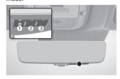
Press the menu button (1). You can adjust the brightness and the vertical angle of the display.
