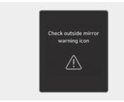
When the outside rearview mirror warning light is not working properly, the "Check outside mirror warning icon" warning message appears on the instrument cluster for several seconds, and the master ( $\triangle$ ) warning light illuminates on the cluster. If this occur, we recommend that your vehicle be inspected by a HYUNDAI authorised repairer.
