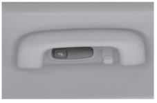
$\overline{X}, \overline{S}$ : Press the button to turn on and off the rear room lamp.
