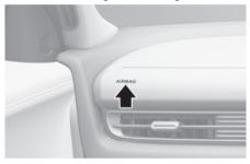
The SRS consists of airbags located in the centre of the steering wheel and the passenger's side front panel pad above the glove box.
