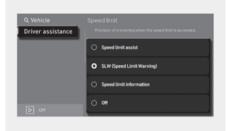
With the vehicle on, select or deselect Settings > Vehicle > Driver assistance > Speed limit from the infotainment system to set whether to use each function.
