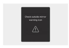
When the outside rearview mirror warning light is not working properly, the "Check outside mirror warning icon" warning message appears on the instrument cluster for several seconds, and the master (A) warning light illuminates on the cluster. If this occur, we recommend that your vehicle be inspected by a HYUNDAI authorised repairer.
