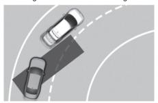
Blind-Spot Collision-Avoidance Assist may not operate properly when driving on a curved road. The function may recognise a vehicle in the same lane.
