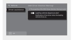
With the vehicle on, select or deselect Settings > Vehicle > Driver assistance > DAW (Driver Attention Warning) and then enable Leading vehicle departure alert in the infotainment system to set whether to use each function.
