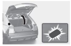
The cargo area lamp turns on when the tailgate is opened and off when the tailgate is closed.
