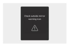
When the outside rearview warning light is not working properly, the "Check outside mirror warning icon" warning message will appear on the instrument cluster for several seconds, and the master (△) warning light will illuminate on the instrument cluster. If this occurs, we recommend that your vehicle be inspected by a HYUNDAI authorised repairer.
