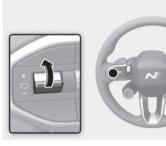
Push the + switch up and release it immediately. The set speed will increase by 1 mph (1 km/h) each time the switch is operated in this manner.  Push the + switch up and hold it whilst monitoring the set speed on the cluster. The set speed will increase by 5 mph (10 km/h) each time the switch is operated in this manner. Release the switch when the desired speed is shown, and the vehicle will accelerate to that speed. You can increase the set speed up to 120 mph (200 km/h).
