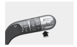
Push the lever away from you to spray rear washer fluid and to run the rear wipers 1-3 cycles. The spray and wiper operation continues until you release the lever
