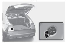
The power outlet is designed to provide power for mobile phones or other devices designed to operate with vehicle electrical systems.
