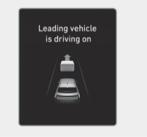
When a detected vehicle in front departs from a stop, Leading Vehicle Departure Alert will inform the driver by displaying the "**Leading vehicle is driving on**" message on the instrument cluster and an audible warning will sound.
