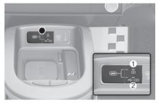
Press the USB port selection button whilst the vehicle is running. Press the upper portion of the button (1) to charge an electronic device. Press the lower portion of the button (2) to charge and listen to music with a media storage device. The USB port can be used after either indicator light turns on.
