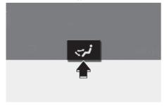
The mode selection switch controls the direction of the air flow through the ventilation system.
