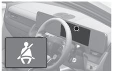
As a reminder to the driver, the driver's seat belt warning lights illuminates for about 6 seconds each time the Start/Stop button is in the ON position regardless of seat belt fastening.
