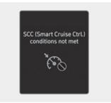
If the Driving Assist button, +, - or IIO switch is operated when Smart Cruise Control operating conditions are not satisfied, the "SCC (Smart Cruise Ctrl.) conditions not met" will appear on the cluster, and an audible warning will sound.
