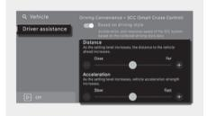
With the vehicle on, select **Settings** > **Vehicle** > **Driver assistance** > **Driving Convenience** > **SCC (Smart Cruise Control)** is selected in the infotainment system, you can change the vehicle distance, the acceleration, and the reaction speed manually.
