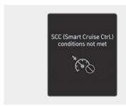
If the Driving Assist button, +, — or II D switch is operated when Smart Cruise Control operating conditions are not satisfied, the "SCC (Smart Cruise Ctrl.) conditions not met" will appear on the cluster, and an audible warning will sound.
