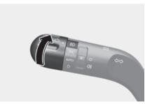
The headlight, position light, number plate light and instrument panel lamp are turned ON.
