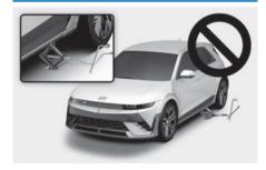
Never start or run the vehicle whilst an AWD vehicle is raised on a jack. The vehicle can slip or roll off of a jack causing serious injury or death to you or those nearby.
