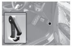
3. Go to the front of the vehicle, raise the bonnet slightly, push to the left the secondary bonnet release lever (1) inside of the bonnet centre and lift the bonnet (2).
