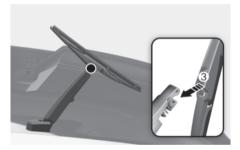
4. If the replacement is complete, put down the wiper arm onto the rear windscreen, and turn the vehicle ON and operate the wipers to check the blade is installed correctly.
