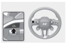
To turn Smart Cruise Control off, press the Driving Assist (යිබ) button.
