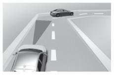
• The front sensors may be unable to recognise the foregoing vehicle if you are coasting on a curve. The regenerative braking intensity may automatically be lowered, which may accelerate the vehicle.
