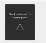
When the outside rearview mirror warning light is not working properly, the "Check outside mirror warning icon" warning message will appear on the cluster for several seconds, and the master ( $\triangle$ ) warning light will appear on the cluster. If this occurs, we recommend that your vehicle be inspected by a HYUNDAI authorised repairer.
