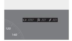
The main settings of CUSTOM mode is displayed at the top of the cluster. The CUSTOM mode can be set on the infotainment system.
