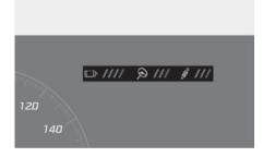
The main settings of CUSTOM mode is displayed at the top of the cluster. The CUSTOM mode can be set on the infotainment system.
