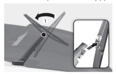
Install the new blade assembly by inserting the centre part into the slot in the wiper arm until it clicks into place (3).
