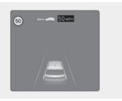
Manual Speed Limit Assist or Smart Cruise Control assists the vehicle to adjust its speed according to the speed limit. When the cruising speed is set as same as the speed limit, the vehicle automatically adjusts its speed if the speed limit changes. The function operates on the road which has a speed limit of 45 mph (70 km/h) or higher. When the function is active, the cruising speed on the instrument cluster appears in green.
