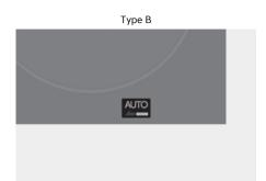
The smart regeneration system is ON and the regenerative braking level is displayed as 'AUTO'.
