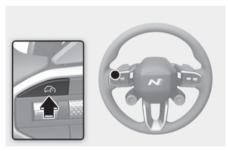
Press the Driving Assist ((20)) button to turn Cruise Control off. The Cruise ((NCRUISE) indicator will go off.
