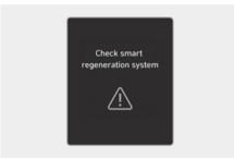
If the smart regeneration system is turned off due to the front radar being covered with foreign substances or due to other causes, the "Check Smart Regeneration System" warning message appears. Also the regenerative braking level is displayed instead of 'AUTO'.
