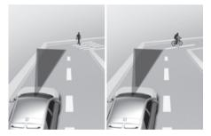
Forward Collision-Avoidance Assist may not detect other vehicles, powered two-wheelers, pedestrians or cyclists in front of you when driving on curved roads adversely affecting the performance of the sensors. This may result in no warning, braking assist when necessary.
