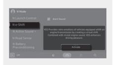
• When N e-Shift is activated, the sound of N Active Sound+ will automatically turn to ignition mode.
