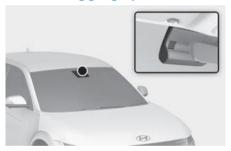
The Auto defogging reduces the likelihood of fogging up the inside of the windscreen by automatically sensing moisture on inside of the windscreen.
