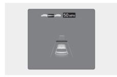
If you want to speed up temporarily without altering the set speed whilst Smart Cruise Control is operating, depress the accelerator pedal. Whilst the accelerator pedal is depressed, the set speed, distance level and target distance will blink on the cluster.
