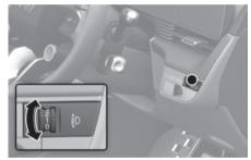
To adjust the headlight beam level according to the number of the passengers and loading weight in the luggage area, turn the beam levelling switch.
