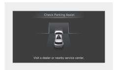
When Remote Smart Parking Assist is not working properly, the 'Check Parking Assist' warning message will appear on the infotainment system. If the message appears, stop using Remote Smart Parking Assist, and we recommend that you have the vehicle inspected by a HYUNDAI authorised repairer.
