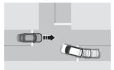
Junction Turning function can help avoid a collision with an oncoming vehicle or powered two-wheeler in an adjacent lane when turning left (left-hand drive) or right (right-hand drive) at a crossroad with the turn signal on by applying emergency braking.
