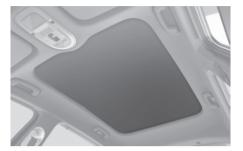
If your vehicle is equipped with a vision roof, you can slide open the power sunshade and an all-glass roof appears.
