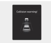
Whilst Smart Cruise Control is operating, when the collision risk with the vehicle ahead is high, the '**Collision Warning!**' warning message will appear on the instrument cluster, and an audible warning will sound to warn the driver. Always have your eyes on the road whilst driving, and if necessary, depress the brake pedal to reduce your driving speed in order to maintain a safe distance.
