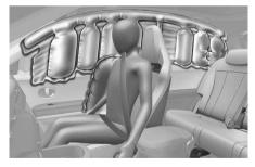
Side and curtain airbags are designed to inflate when an impact is detected by side collision sensors depending on the severity of impact resulting from a side impact collision. Although the driver's and front passenger's airbags are designed to inflate in frontal collisions and side and curtain airbags are designed to inflate in side impact collisions, airbags may inflate in other types of collisions if the sensors detect a sufficient impact.
