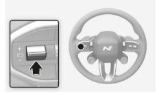
Press the **IIO** switch or depress the brake pedal to temporarily cancel Smart Cruise Control.
