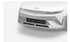
Active air flap system controls the air flap below the front bumper to cool the vehicle parts and improve energy efficiency.
