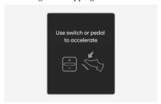
When Highway Driving Assist is operating, your vehicle will stop if the vehicle ahead of you stops. Also, if the vehicle ahead of you starts moving within 30 seconds after the stop, your vehicle
