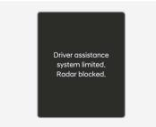
When the rear bumper around the rear corner radar or sensor is covered with foreign material, such as snow or rain, or installing a trailer or carrier, it can reduce the detecting performance and temporarily limit or disable Blind-Spot Collision-Avoidance Assist. If this occurs, the "**Driver assistance** system limited. Radar blocked." warning message will appear on the cluster.
