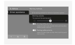
With the vehicle on, go to Settings > Vehicle > Driver assistance > Warning methods from the Settings in the infotainment system to select the following:
