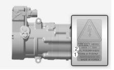
A compressor label informs you the type of compressor your vehicle is equipped with such as model, supplier part number, production number, refrigerant (1) and refrigerant oil (2).
