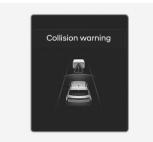
While Smart Cruise Control is operating, when the collision risk with the vehicle ahead is high, the "**Collision Warning**" warning message will appear on the instrument cluster, and an audible warning will sound to warn the driver. Always have your eyes on the road while driving, and if necessary, depress the brake pedal to reduce your driving speed in order to maintain a safe distance.
