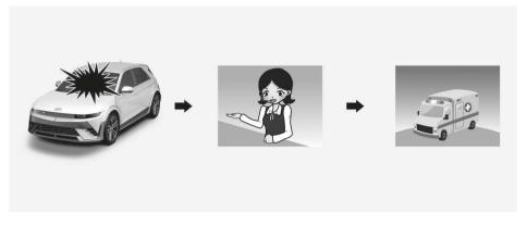
The Pan-European eCall device automatically makes an emergency call to the Public Safety Answering Point (PSAP) for proper rescuing operations in event of vehicle accident.
