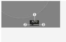
The instrument cluster displays 'AUTO' (1) when the smart regeneration system is ON. Depending on the conditions, the system adjusts the regenerative braking level (2). The sky blue indicator light (3) illuminates when the vehicle recognizes a vehicle.
