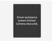
When the front windshield where the front view camera is located, or sensor is covered with foreign material, such as snow or rain, it can reduce the detecting performance and temporarily limit or disable Lane Keeping Assist. If this occurs, the "Driver assistance system limited. Camera obscured." warning message and the master ( $\triangle$ ) warning light or Lane Keeping Assist (/ $\equiv$ )
