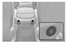
The USB charger is designed to recharge batteries of small size electronic devices using a USB cable.
