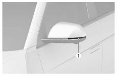
If the side repeater light (1) does not operate, we recommend that the system be inspected by an authorized HYUNDAI dealer.
