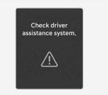
When Safe Exit Warning is not working properly, the "**Check driver assistance system.**" warning message will appear on the cluster for several seconds, and the master warning light ( $\triangle$ ) will appear on the cluster. If this occurs, we recommend that your vehicle be inspected by an authorized HYUNDAI dealer.
