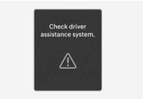
When Rear Cross-Traffic Collision-Avoidance Assist is not working properly, the "**Check driver assistance system.**" warning message appears on the instrument cluster for several seconds, and the master (A) warning light illuminates on the instrument cluster. If this occur, we recommend that your vehicle be inspected by an authorized HYUNDAI dealer.
