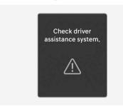
When Lane Following Assist is not working properly, the "Check driver assistance system." warning message will appear on the instrument cluster for several seconds, and the master (A) warning light appears on the instrument cluster. If this occur, we recommend that your vehicle be inspected by an authorized HYUNDAI dealer.
