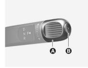
[A] Rotary gear shift dial[B] P button
