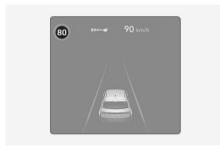
When driving at a speed higher than the displayed speed limit, the red speed limit indicator will blink and warning sounds.
