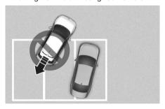
If Remote Smart Parking Assist is used when parking in a space next to misaligned vehicles, your vehicle may not be parked side by side.
