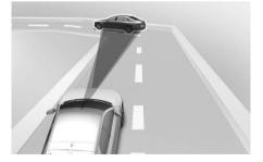
Your vehicle speed can be reduced due to a vehicle in the adjacent lane.
