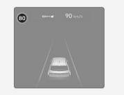
When driving at a speed higher than the displayed speed limit, the red speed limit indicator will blink and warning sounds.
