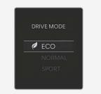
The mode changes, whenever the N1 or N2 button on the steering wheel or the Drive mode button is pressed.
