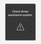
When Intelligent Speed Limit Assist is not working properly, the "**Check driver assistance system.**" warning message will appear on the instrument cluster for several seconds, and the master (A) warning light and speed limit ( $\bigcirc$ ) warning light will appear on the instrument cluster. If this occurs, we recommend that your vehicle be inspected by an authorized HYUNDAI dealer.
