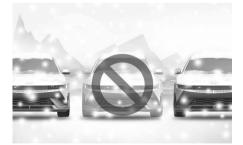
Snow may interfere with the operation of the ultrasonic sensor and wide view camera, or Remote Smart Parking Assist may cancel if the road is slippery while parking. Abnormal parking space
