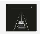
If the vehicle ahead and/or both lane markings are detected and your vehicle speed is below 200 km/h (120 mph), the green (②) indicator light appears on the cluster, and Lane Following Assist helps center the vehicle in the lane by assisting the steering wheel.
