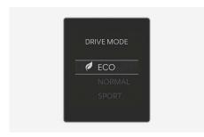
The mode changes, whenever the N1 or N2 button on the steering wheel or the Drive mode button is pressed.
