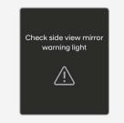
When the outside rearview warning light is not working properly, the "Check side view mirror warning light" (or "Check outside mirror warning icon") warning message will appear on the instrument cluster for several seconds, and the master ( $\triangle$ ) warning light will illuminate on the instrument cluster. If this occurs, we recommend that your vehicle be inspected by an authorized HYUNDAI dealer.
