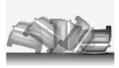
Front airbags may not inflate in rollover accidents because front airbag deployment would not provide additional occupant protection.
