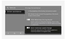
With the vehicle on, select Settings > Vehicle > Driver assistance > Driving Convenience > Auto motorway speed change from the infotainment system to turn on Navigation based Smart Cruise Control and deselect to turn off the function.
