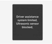
If this occurs the "**Driver assistance** system limited. Ultrasonic sensor blocked." warning message appears on the instrument cluster. Parking Distance Warning operates properly when snow, rain or foreign material is removed. If Parking Distance Warning does not operate properly after obstruction (snow, rain, or foreign material) is removed (including trailer, carrier, etc., from the rear bumper), we recommend to have your vehicle inspected by an authorized HYUNDAI dealer.
