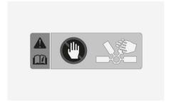
Do not put your hand near the cooling fan in the motor compartment while charging. It may operate automatically to control the battery temperature, even if the vehicle is turned off.
