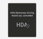
If the driver still does not have their hands on the steering wheel after the hands-off warning, "HDA (Motorway Driving Assist) sys. cancelled" (or "Highway Driving Assist deactivated") warning message will appear and Highway Driving Assist and Lane Change Assist will be automatically cancelled.
