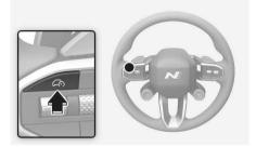
To turn Smart Cruise Control off, press the Driving Assist (ন্কে) button.
