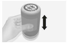
2. Remove the sealant bottle (2) cap and open the sealant bottle holder (5) cap and screw the bottle onto the sealant bottle holder.
