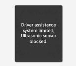
If this occurs the "**Driver assistance** system limited. Ultrasonic sensor blocked." warning message appears on the instrument cluster. Parking Distance Warning operates properly when snow, rain or foreign material is removed.
