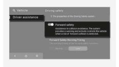
With the vehicle on, select **Settings** > **Vehicle** > **Driver assistance** > **Driving safety** in the infotainment system to set whether to use each function.
