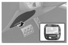
Inside the fuse panel cover, you can find the panel label describing fuse names and ratings.
