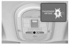
Insert the key or a similar rigid device into the passenger's front airbag ON/OFF switch and turn it to the ON position [A]. The passenger airbag ON indicator (<sup>®</sup>) illuminates.
