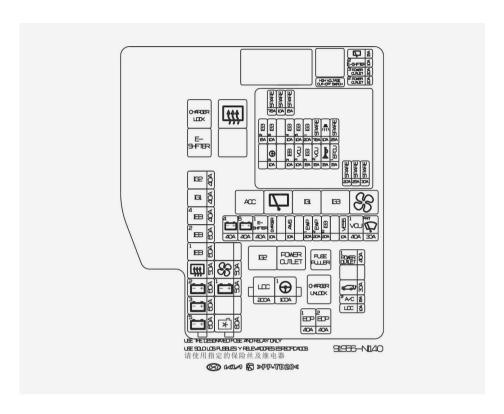
Motor compartment fuse panel (Motor compartment junction block)
