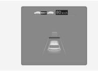
If you want to speed up temporarily without altering the set speed while Smart Cruise Control is operating, depress the accelerator pedal. While the accelerator pedal is depressed, the set speed, distance level and target distance will blink on the cluster.
