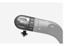
To flash the high beam headlight, pull the lever towards you, then release the lever. The high beams remain ON as long as you hold the lever.
