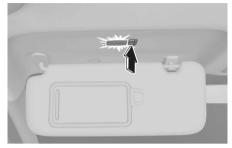
Push the switch to turn the lamp on or off.
