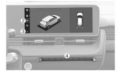
The 3D view shows the image around the vehicle from various angles.
