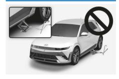
Never start or run the vehicle while an AWD vehicle is raised on a jack. The vehicle can slip or roll off of a jack causing serious injury or death to you or those nearby.
