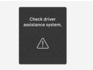
When Forward Collision-Avoidance Assist is not working properly, the "Check driver assistance system." warning message will appear, and the swarning lights will illuminate on the instrument cluster. We recommend that your vehicle be inspected by an authorized HYUNDAI dealer.
