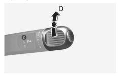
To shift the gear to D (Drive), rotate the rotary gear shift dial to D (Drive) while depressing the brake pedal.
