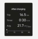
Trip distance, total driving time, average energy consumption, and instant energy consumption after the vehicle has been recharged are displayed. To reset manually, press the **OK** button on the steering wheel for more than 1 second when "After charging" appears.
