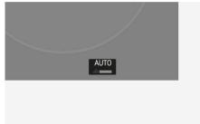
The smart regeneration system is ON and the regenerative braking level is displayed as 'AUTO'.
