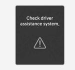
When Parking Collision-Avoidance Assist or other related functions are not working properly, the "**Check driver assistance system.**" warning message will appear on the instrument cluster, and Parking Collision-Avoidance Assist will turn off automatically. We recommend that you have the vehicle inspected by an authorized HYUNDAI dealer.
