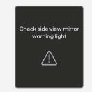
When the side view mirror warning light is not working properly, the "**Check side view mirror warning light**" (or "**Check outside mirror warning icon**") warning message will appear on the instrument cluster for several seconds, and the master (**A**) warning light will appear on the instrument cluster. If this occurs, we recommend that your vehicle be inspected by an authorized HYUNDAI dealer.
