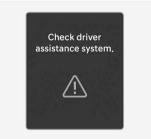
When Lane Keeping Assist is not working properly, the "**Check driver assistance system**" warning message and yellow Lane Keeping Assist (/=\) warning light appears on the cluster. If this occurs, we recommend that your vehicle be inspected by an authorized HYUNDAI dealer.
