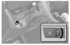
To adjust the headlight beam level according to the number of the passengers and loading weight in the luggage area, turn the beam leveling switch.
