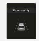
• When the vehicle is stopped due to emergency braking, the "**Drive carefully**" warning message will appear on the cluster.
