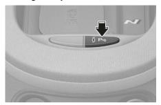
Press the Parking Safety (P<sup>n</sup>) button to turn on Forward/Reverse Parking Distance Warning. Press the button again to turn off the function.
