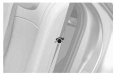
4. Pull up the seatback folding lever (1), then fold the seat toward the front of the vehicle (2).
