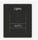
This indicator displays which exterior light is selected using the lighting control.
