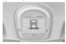
Elements of the UAE eCall System, installed in passenger compartment:
