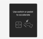
In traffic, your vehicle will stop if the vehicle ahead of you stops. Also, if the vehicle ahead of you starts moving, your vehicle will start as well. In addition, after the vehicle has stopped and a certain time have passed, the "**Use switch or pedal to accelerate**" message will appear on the instrument cluster. Depress the accelerator pedal or operate the + switch, - switch or **IIO** switch to start driving.
