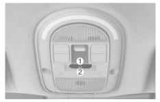
Elements of the UAE eCall System, installed in passenger compartment: (1) SOS button (2) LED SOS button: the driver/passenger makes an emergency call to the single duty dispatch service by pressing the button.
