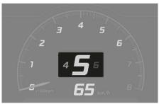
In the manual shift mode, this indicator informs which gear is desired while driving to save energy.
