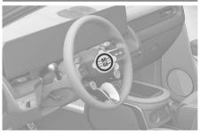
Detach the speed restriction label (1) from the sealant bottle (2), and place it in a highly visible place inside the vehicle such as on the steering wheel to remind the driver not to drive too fast.
