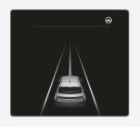
If the vehicle ahead and/or both lane markings are detected and your vehicle speed is below 200 km/h (120 mph), the green  $(\Theta)$  indicator light appears on the cluster, and Lane Following Assist helps center the vehicle in the lane by assisting the steering wheel.
