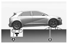
[A] Roll tester (Speedometer)[B] Temporary free roller
