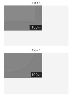
The odometer indicates the total distance that the vehicle has been driven and is used to determine when periodic maintenance is required.
