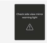
When the side view mirror warning light is not working properly, the "Check side view mirror warning light" (or "Check outside mirror warning icon") warning message will appear on the cluster for several seconds, and the master warning light (A) will appear on the cluster. If this occurs, we recommend that your vehicle be inspected by an authorized HYUNDAI dealer.
