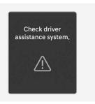
When Intelligent Speed Limit Assist is not working properly, the "Check driver assistance system." warning message will appear on the instrument cluster for several seconds, and the master (⚠) warning light and speed limit (⊖) warning light will appear on the instrument cluster. If this occurs, we recommend that your vehicle be inspected by an authorized HYUNDAI dealer.
