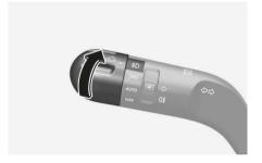
The headlight, position light, license plate light and instrument panel lamp are turned ON.
