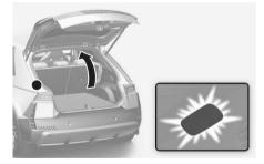
The cargo area lamp turns on when the tailgate is opened and off when the tailgate is closed.
