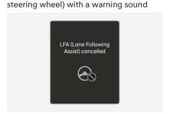
If the driver still does not have their hands on the steering wheel after the hands-off warning, the "LFA (Lane Following Assist) cancelled" (or "Lane Following Assist deactivated") warning message will appear and Lane Following Assist will be automatically cancelled.
