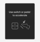
When Highway Driving Assist is operating, your vehicle will stop if the vehicle ahead of you stops. Also, if the vehicle ahead of you starts moving within 30 seconds after the stop, your vehicle will start as well. In addition, after the vehicle has stopped and 30 seconds have passed, the "**Use switch or pedal to accelerate**" message will appear on the instrument cluster. Depress the accelerator pedal or operate the **+** switch, - switch or **IIO** switch to start driving.
