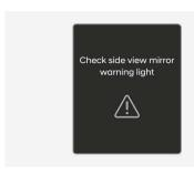
When the outside rearview warning light is not working properly, the "Check side view mirror warning light" (or "Check outside mirror warning icon") warning message will appear on the instrument cluster for several seconds, and the master (A) warning light will illuminate on the instrument cluster. If this occurs, we recommend that your vehicle be inspected by an authorized HYUNDAI dealer.
