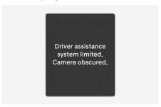
When the front windshield where the front view camera is located, or sensor is covered with foreign material, such as snow or rain, it can reduce the detecting performance and temporarily limit or disable Lane Keeping Assist.
