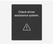
When Smart Cruise Control is not working properly, the "**Check driver assistance system.**" warning message and the master (A) warning light will appear on the instrument cluster. We recommend that your vehicle be inspected by an authorized HYUNDAI dealer.
