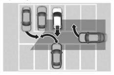
Rear Cross-Traffic Collision-Avoidance Assist may detect vehicles which are parking or pulling out near your vehicle (for example, a vehicle leaving beside your vehicle, a vehicle parking or pulling out in the rear area, a vehicle approaching your vehicle making a turn, etc.). If this occurs, the function may unnecessarily warn the driver and control the brake.
