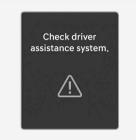
When Lane Following Assist is not working properly, the "**Check driver assistance system."** warning message will appear on the instrument cluster for several seconds, and the master (A) warning light appears on the instrument cluster. If this occur, we recommend that your vehicle be inspected by an authorized HYUNDAI dealer.
