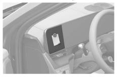
The cluster fascia side panel is a pad to attach light items such as parking tickets, receipts, etc., using its magnetic surface.
