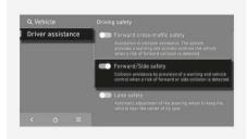
With the vehicle on, select **Settings** > **Vehicle** > **Driver assistance** > **Driving safety** > **Forward/Side safety** in the infotainment system to set whether to use each function.
