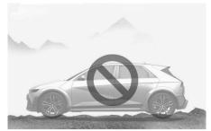
Remote Smart Parking Assist may cancel when the vehicle slips, or the vehicle cannot move due to road conditions such as pebbles or fragmented stones.
