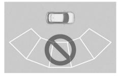
Remote Smart Parking Assist does not work properly when the parking lines are not parallel. Do not park although the parking space is recognized by the sensor.
