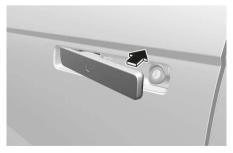
When all doors are closed, touch the touch sensor on the front outside door handle (the engraved part) while carrying the Smart Key with you, outside door handle will return and doors will be locked.
