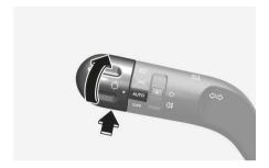
Hight Beam Assist automatically switches between high beam and low beam depending on the detected brightness from the lights of oncoming vehicles or vehicles in front.
