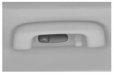
$\overline{\hookrightarrow}$ ,  $\overline{\hookrightarrow}$ : Press the button to turn on and off the rear room lamp.
