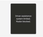
When the rear bumper around the rear corner radar or sensor is covered with foreign material, such as snow or rain, or installing a trailer or carrier, it can reduce the detecting performance and temporarily limit or disable Safe Exit Assist.
