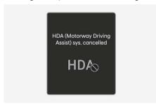
If the driver still does not have their hands on the steering wheel after the hands-off warning, "HDA (Motorway Driving Assist) sys. cancelled" (or "Highway Driving Assist deactivated") warning message will appear and Highway Driving Assist and Lane Change Assist will be automatically cancelled.
