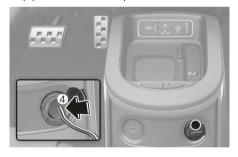
6. With the vehicle ON (READY indicator ON), switch on the compressor and let it run for about 5-7 minutes to fill the sealant up to proper pressure. (refer to the "Tires and wheels" section in chapter 2). The inflation pressure of the tire after filling is unimportant and will be checked/corrected later.
