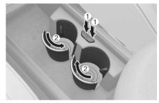
Push the button (1). The cup supporter protrudes from the front console.
