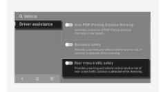
With the vehicle on, select **Settings** > **Vehicle** > **Driver assistance** > **Parking safety** > **Rear cross-traffic safety** in the infotainment system to turn on Rear Cross-Traffic Collision-Avoidance Assist and deselect to turn off the function.
