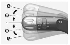
Highway Lane Change Assist function will operate, when you push the turn signal lever up or down to the A or B position while the function is in the ready state (indicator is green), and all of the following conditions are satisfied:
