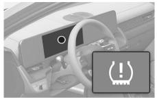
The TPMS Malfunction Indicator ((!)) illuminates after it blinks for about one minute when there is a problem with the Tire Pressure Monitoring System.
