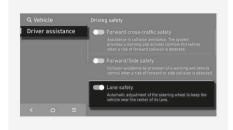
With the vehicle on, select **Settings** > **Vehicle** > **Driver assistance** > **Driving safety** > **Lane safety** in the infotainment system to set whether to use each function.
