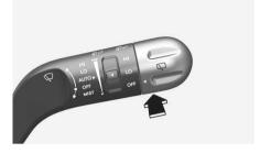
Push the lever away from you to spray rear washer fluid and to run the rear wipers 1-3 cycles. The spray and wiper operation continues until you release the lever.
