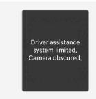
When the front windshield where the front view camera is located is covered with foreign material, such as snow or rain, it can reduce the detecting performance and temporarily limit or disable Intelligent Speed Limit Assist. If this occurs, the "Driver assistance"
