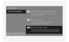
With the vehicle on, select **Settings** > **Vehicle** > **Driver assistance** > **Parking safety** > **Rear cross-traffic safety** in the infotainment system to turn on Rear Cross-Traffic Collision-Avoidance Assist and deselect to turn off the function.
