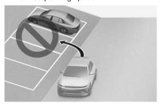
Remote Smart Parking Assist does not work properly on a inclined or curved road surface. Do not park although the parking space is recognized by the sensor.
