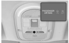
Insert the key or a similar rigid device into the passenger's front airbag ON/ OFF switch and turn it to the OFF position [B]. The passenger airbag OFF indicator (\*) illuminates and stays on until the passenger's front airbag is reactivated. To reactivate the passenger's front airbag:
