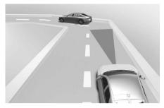
• The front sensors may be unable to recognize the foregoing vehicle if you are coasting on a curve. The regenerative braking intensity may automatically be lowered, which may accelerate the vehicle.
