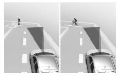
Forward Collision-Avoidance Assist may not detect other vehicles, powered two-wheelers, pedestrians or cyclists in front of you when driving on curved roads adversely affecting the performance of the sensors. This may result in no warning, braking or steering (if equipped) assist when necessary.
