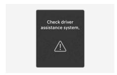
When Blind-Spot Collision Warning is not working properly, the "Check driver assistance system." warning message will appear on the instrument cluster for several seconds, and the master (1/2)
