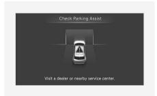
When Remote Smart Parking Assist is not working properly, the 'Check Parking Assist' warning message will appear on the infotainment system. If the message appears, stop using Remote Smart Parking Assist, and we recommend that you have the vehicle inspected by an authorized HYUNDAI dealer.
