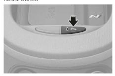
Press and hold the Parking Safety (P<sub>m</sub>) button more than 2 seconds, 'Rear Active Assist' or to turn the Parking Collision-Avoidance Assist on or off.
