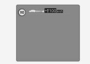
If the speed limit of the road changes during the operation of Manual Speed Limit Assist or Smart Cruise Control, an arrow in the direction of up or down is displayed to inform the driver that the set speed needs to be changed. At this time, the driver can change the set speed according to the speed limit by using the + or - switch on the steering wheel.
