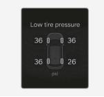
This warning message appears if the tire pressure is low. The corresponding tire on the vehicle is illuminated.
