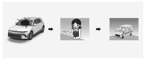
The UAE eCall device automatically makes an emergency call to the Public Safety Answering Point (PSAP) for proper rescuing operations in event of vehicle accident.
