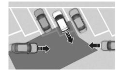
Rear Cross-Traffic Collision-Avoidance Assist may be limited when backing up diagonally, and may not detect the vehicle approaching from the left or right. If this occurs, the function may not warn the driver or control the brakes when necessary.
