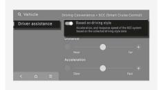
With the vehicle on, select **Settings** > **Vehicle** > **Driver assistance** > **Driving convenience** > **SCC (Smart Cruise Control)** > **Based on driving style** is selected in the infotainment system, Smart Cruise Control will operate based on the driver's driving style, such as vehicle distance, acceleration, reaction speed.
