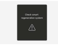
If the smart regeneration system is turned off due to the front radar being covered with foreign substances or due to other causes, the "Check smart regeneration system" warning message appears. Also the regenerative braking level is displayed instead of 'AUTO'.
