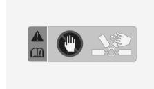
When using the V2L, the cooling fan in the vehicle motor compartment can operate automatically even if the vehicle is turned off. Do not put your hand near the cooling fan in the V2L operating state.
