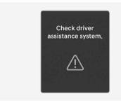
When Lane Keeping Assist is not working properly, the "Check driver assistance system" warning message and yellow Lane Keeping Assist (A) warning light appears on the cluster. If this occurs, we recommend that your vehicle be inspected by an authorized HYUNDAI dealer.
