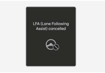
If the driver still does not have their hands on the steering wheel after the hands-off warning, the "LFA (Lane Following Assist) cancelled" (or "Lane Following Assist deactivated")warning message will appear and Lane Following Assist will be automatically cancelled.
