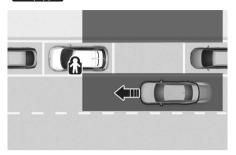
While your vehicle is stopped, and if Safe Exit Assist detects a vehicle approaching the rear corner of your vehicle and a passenger opens a door, Safe Exit Assist may warn you with a warning message and a warning sound to help avoid a collision.
