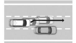
When vehicle speed is above 60 km/h (40 mph), if a detected vehicle around you is driving at a close distance, your vehicle will control steering in the opposite direction of the vehicle to assist in safe driving. If there a detected vehicle in both sides of the lane that are driving close to you, the function will not veer to the opposite side of the lane.
