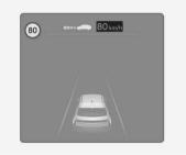
Manual Speed Limit Assist or Smart Cruise Control assists the vehicle to adjust its speed according to the speed limit. When the cruising speed is set as same as the speed limit, the vehicle automatically adjusts its speed if the speed limit changes. The function operates on the road which has a speed limit of 70 km/h (45 mph) or higher. When the function is active, the cruising speed on the instrument cluster appears in green.
