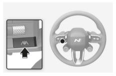
With the vehicle on, shortly press the Lane Driving Assist button located on the steering wheel to turn on Lane Following Assist. The gray or green (⋈) indicator light will appear on the cluster.
