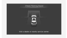
When Remote Smart Parking Assist is not working properly, the '**Check Parking Assist**' warning message will appear on the infotainment system. If the message appears, stop using Remote Smart Parking Assist, and we recommend that you have the vehicle inspected by an authorized HYUNDAI dealer. **Remote Smart Parking Assist canceled**
