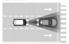
Forward Collision-Avoidance Assist detects a vehicle, a powered two-wheeler, a pedestrian, or a cyclist ahead on the road and may warn you of a possible collision with a warning message on the instrument cluster and a warning sound. Also, Forward Collision-Avoidance Assist may assist with braking your vehicle to help reduce collision speed or avoid a collision.
