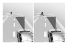
Forward Collision-Avoidance Assist may not detect other vehicles, powered two-wheelers, pedestrians or cyclists in front of you when driving on curved roads adversely affecting the performance of the sensors. This may result in no warning, braking or steering (if equipped) assist when necessary.
