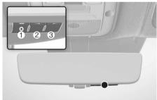
1. Press the menu button (1). You can adjust the brightness and the vertical angle of the display.
