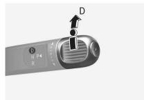
To shift the gear to D (Drive), rotate the rotary gear shift dial to D (Drive) while depressing the brake pedal.
