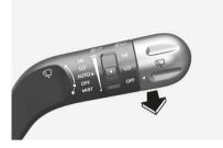
In the **OFF(O)** position, pull the lever gently toward you to spray washer fluid on the windshield and to run the wipers 1-3 cycles. The spray and wiper operation continues until you release the lever. If the washer does not work, you may need to add washer fluid to the washer fluid reservoir.
