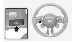
With the vehicle on, shortly press the Lane Driving Assist button located on the steering wheel to turn on Lane Following Assist. The gray or green  $(\Theta)$  indicator light will appear on the cluster.
