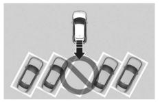
Remote forward function may not operate properly in a diagonal parking space.
