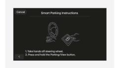
If Remote Smart Parking Assist cannot activate Remote Parking function, only the Smart Parking guide will be displayed on the infotainment system.
