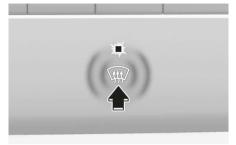
Press the front windshield defroster button (indicator light ON) to turn on the front windshield defroster. If the windshield defogging is set, outside (fresh) mode is automatically selected and the air conditioning turns on according to the detected ambient temperature.
