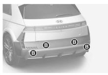
[A] Front ultrasonic sensors[B] Rear ultrasonic sensors
