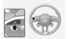
Press the Driving Assist ( ( ) button to turn Cruise Control off. The Cruise ( CRUISE) indicator will go off.
