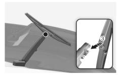
4. If the replacement is complete, put down the wiper arm onto the rear windshield, and turn the vehicle ON and operate the wipers to check the blade is installed correctly.
