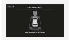
When the vehicle is stopped by depressing the brake pedal, the vehicle sensors will detect the distance from nearby objects and check for space to exit.
