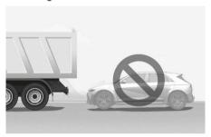
Do not use Remote Smart Parking Assist around vehicles with higher ground clearance, such as a bus, truck, etc. It may lead to an accident. · Parking near a pillar
