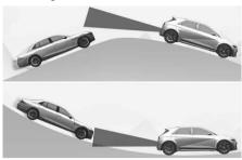
Blind-Spot Collision-Avoidance Assist may not operate properly when driving on a slope. The function may not detect the vehicle in the next lane or may incorrectly detect the ground or structure. Always pay attention to road and driving conditions while driving.
