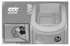
6. With the vehicle ON (READY indicator ON), switch on the compressor and let it run for about 5-7 minutes to fill the sealant up to proper pressure. (refer to the "Tires and wheels" section in chapter 2). The inflation pressure of the tire after filling is unimportant and will be checked/corrected later.
