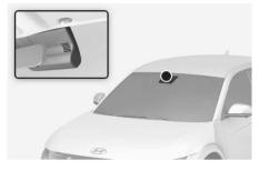
The Auto defogging reduces the likelihood of fogging up the inside of the windshield by automatically sensing the moisture on inside of the windshield.
