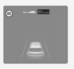
Manual Speed Limit Assist or Smart Cruise Control assists the vehicle to adjust its speed according to the speed limit. When the cruising speed is set as same as the speed limit, the vehicle automatically adjusts its speed if the speed limit changes. The function operates on the road which has a speed limit of 70 km/h (45 mph) or higher. When the function is active, the cruising speed on the instrument cluster appears in green.
