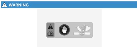
Do not put your hand near the cooling fan in the motor compartment while charging. It may operate automatically to control the battery temperature, even if the vehicle is turned off.
