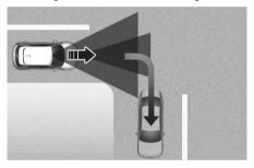
When a vehicle in front of you merges out of the lane, Smart Cruise Control may not immediately detect the new vehicle that is now in front of you.
