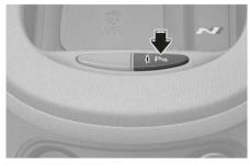
Press and hold the Parking Safety (Pm) button more than 2 seconds, 'Rear Active Assist' or to turn the Parking Collision-Avoidance Assist on or off.
