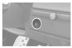
Whenever the front door is opened, the Start/Stop button illuminates and goes off for a few seconds after the door is closed.
