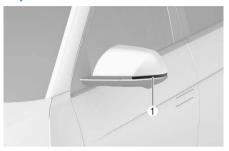
If the side repeater light (1) does not operate, we recommend that the system be inspected by an authorized HYUNDAI dealer.
