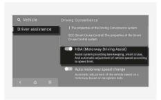
With the vehicle on, select or deselect Settings > Vehicle > Driver assistance > Driving Convenience > HDA (Motorway Driving Assist) from the infotainment system to set whether to use each function.
