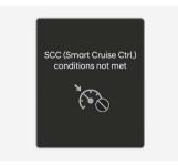
If the Driving Assist button, + switch, switch or II'O switch is operated when Smart Cruise Control operating conditions are not satisfied, the "SCC (Smart Cruise Ctrl.) conditions not met" (or "Smart Cruise Control conditions not met") will appear on the cluster, and an audible warning will sound.
