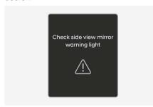
When the side view mirror warning light is not working properly, the "Check side view mirror warning light" (or "Check outside mirror warning icon") warning message will appear on the instrument cluster for several seconds, and the master (A) warning light will appear on the instrument cluster. If this occurs, we recommend that your vehicle be inspected by an authorized HYUNDAI dealer
