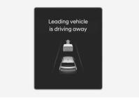
When a detected vehicle in front departs from a stop, Leading Vehicle Departure Alert will inform the driver by displaying the "Leading vehicle is driving away" (or "Leading vehicle is driving on") message on the instrument cluster and an audible warning will sound.
