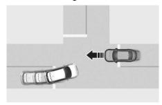
Junction Turning function can help avoid a collision with an oncoming vehicle or powered two-wheeler in an adjacent lane when turning left (left-hand drive) or right (right-hand drive) at a crossroad with the turn signal on by applying emergency braking.
