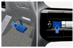
Press the II switch or depress the brake pedal to temporarily cancel SCC.
