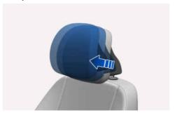
The head restraint may be adjusted forward to 3 different positions by pulling the head restraint forward to the desired detent. To adjust the head restraint to it's furthest rearwards position, pull it fully forward to the farthest position and release it.
