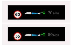
If the speed limit of the road changes during the operation of Manual Speed Limit Assist (MSLA) or Smart Cruise Control (SCC), an arrow in the direction of up or down appears to inform the driver that the set speed needs to be changed. At this time, the driver can change the set speed according to the speed limit by using the + or - switch on the steering wheel.
