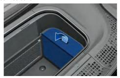
7 Connect the cables to the + jumper terminal in the motor compartment fuse panel and the - jumper terminal in numerical order.
