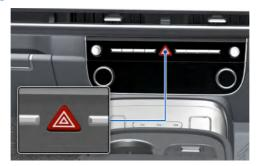
The hazard warning flasher warns other drivers to exercise extreme caution when approaching, overtaking, or passing your vehicle. It should be used whenever making emergency repairs or when stopped near the edge of a roadway.
