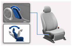
Push the control switch forward or rearward to adjust the seatback angle.
