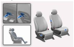
Press and hold the front portion of the Relaxation mode switch to return the seat to the original position.
