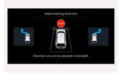
With the vehicle stopped by depressing the brake pedal, touch the infotainment system to select the desired exit direction.
