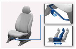
Slide the seat whilst pulling up and holding the seat slide adjustment lever. Release the lever at the position you desire.
