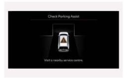
When RSPA is not working properly, the 'Check Parking Assist' warning message appears on the infotainment system. If the message appears, stop using RSPA, and we recommend that your vehicle be inspected by a HYUNDAI authorised repairer.
