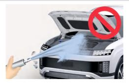
Water washing in the motor compartment including high pressure water washing may cause the failure of electrical circuits located in the motor compartment.
