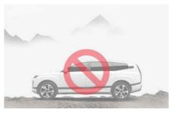
RSPA may cancel when the vehicle slips, or the vehicle cannot move due to road conditions such as pebbles or fragmented stones.
