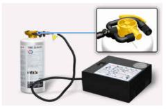
3 Unscrew the valve cap from the valve of the defective wheel and screw the filling hose of the sealant bottle onto the tyre valve.
