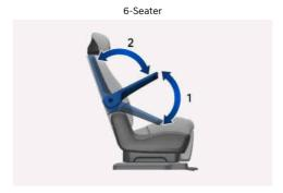
When the armrest is within Range 2, lower the armrest to the lowest position, then lift the armrest within Range 1 of the armrest adjustment angle, and then use it at the angle you desire.
