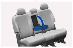
You can open or close the armrest by pulling the top of the armrest forward or pushing it toward the seatback.
