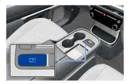
Press and hold the Parking/View P button to turn on RSPA. Also, Parking Distance Warning (PDW) and Surround View Monitor (SVM) automatically turns on.
