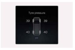
You can check the tyre pressure in the Utility view mode on the cluster display.
