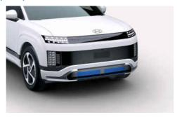
AAF system controls the air flap below the front bumper to cool the vehicle parts and improve energy efficiency.
