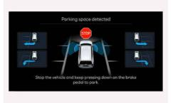
Parking type: Perpendicular reverse (Left/Right), Parallel reverse (Left/Right), Diagonal reverse (Left/Right) With the vehicle stopped by depressing the brake pedal, touch the infotainment system to select the desired parking type.
