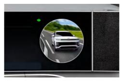
When the left or right side turn signal turns on, the image in that direction appears on the instrument cluster.
