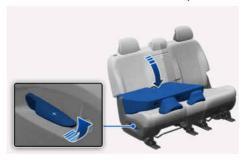
· When using it as a seat, pull the seatback folding lever (2nd row seat) to fully raise the seatback. Adjust the seatback to the desired angle and release the lever to lock in place.
