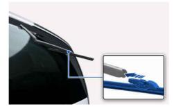
5 If the replacement is complete, put down the wiper arm onto the rear windscreen, and turn the Start/Stop button to POWER ON and operate the wipers to check the blade is installed correctly.
