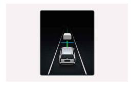
HDA operates on main roads of highways (or motorways), and does not operate on interchanges or junctions.
