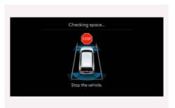
When the vehicle is stopped by depressing the brake pedal, the vehicle sensors detects the distance from nearby objects and check for space to exit.
