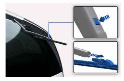
4 Insert a new wiper blade into the wiper arm until an audible "click" sounds.
