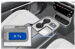
Press the Parking Safety  $P_{N}$  button to turn on PDW. Press the button again to turn off the function.
