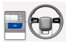
With the vehicle on, shortly press the Lane Driving Assist /⊕\ button located on the steering wheel to turn on LFA. Press the button again to turn off the function.
