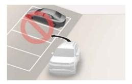
RSPA does not work properly on a inclined or curved road surface. Do not park even though the parking space is recognised by the sensor.
