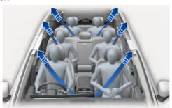
Your vehicle is equipped with driver's, front passenger's and rear passenger's (if equipped) pretensioner seat belts (retractor pretensioner). The pretensioner makes sure the seat belts fit tightly against your body in certain frontal or side collision(s). The pretensioner seat belts may be activated in some crashes where the frontal or side collision(s) is severe enough, together with the airbags.
