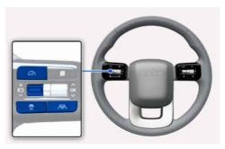
Press the Driving Assist 🚓 button to turn on or off SCC.
