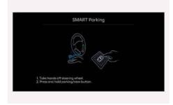
If RSPA cannot activate Remote Parking function, only the Smart Parking guide appears on the infotainment system.
