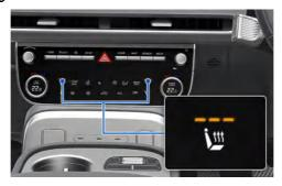
Whilst the vehicle is running, touch the icon to warm the driver's seat or front passenger's seat.
