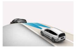
During uphill or downhill driving, the SCC may not detect a moving vehicle in your lane, and cause your vehicle to accelerate to the set speed. Also, vehicle speed rapidly decreases when the vehicle ahead is detected suddenly. Select the appropriate set
