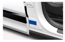
The vehicle certification label attached on the left or right front seat side centre pillar gives the VIN.
