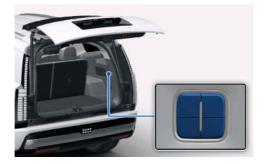
This feature can make it easier for you to fold or unfold the 2nd row, 3rd row seatback when the tailgate is open.
