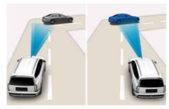
On curves, SCC may not detect a vehicle in the same lane, and may accelerate to the set speed. Also, vehicle speed may rapidly decrease when the vehicle ahead is detected suddenly.
