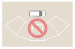
RSPA does not work properly when the parking lines are not parallel. Do not park even though the parking space is recognised by the sensor.
