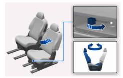
4 Release the swivel lever and turn it fully to the position where the seat orientation is locked.
