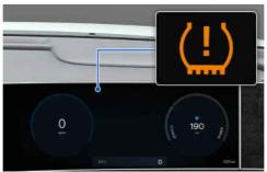
The TPMS Malfunction (1) Indicator illuminates after it blinks for about one minute when there is a problem with the TPMS. We recommend that the system be inspected by a HYUNDAI authorised repairer as soon as possible.
