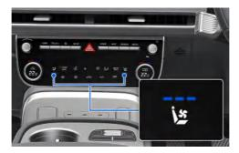
Whilst the vehicle is running, touch the icon to cool the driver's seat or front passenger's seat.
