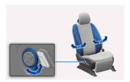
Push the adjustment lever clockwise, the seatback bolster is adjusted inward. Push the lever counterclockwise, the seatback bolster is adjusted outward.
