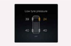
TPMS is not a substitute for manually checking the tyre pressure with a tyre gauge. Changes in temperature affect tyre pressure. For proper tyre inflation and tyre pressure measurement procedure, refer to the 'Check tyre inflation pressure' section in the chapter
