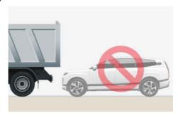
Do not use RSPA around vehicles with higher ground clearance, such as a bus, truck, etc. It may lead to an accident. Park or exit your vehicle manually.
