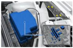
4 Check the removed fuse and replace it if it is blown. Spare fuses are provided in the instrument panel fuse panels (or in the motor compartment fuse panel).
