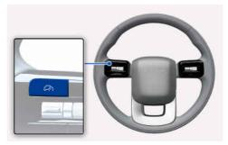
Press the Driving Assist button to turn off Cruise Control. The Cruise (MCRUISE) indicator light goes off.
