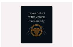
If the driver is still unresponsive despite the prior warning, Emergency Stop controls the steering wheel and brake pedal to stop the vehicle within the driving lane. It is also notified to the driver that Emergency Stop is operating with a warning message, a warning sound, the hazard warning flasher blinking, and vibration on the steering wheel.
