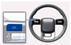
HDA operates when driving on the main road of highways, and turning on/off HDA by pressing the Driving Assist ← button.
