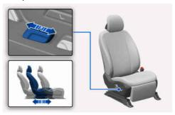
Push the control switch forward or rearward to adjust the seat to the desired position.
