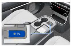
Press and hold the Parking safety Pn button to turn the PCA on or off.
