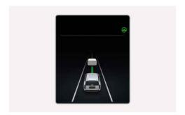
You can see the status of the LFA operation in the Driving Assist view on the instrument cluster. For more information, refer to the 'Cluster settings' section in chapter 4.
