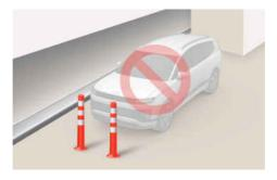
RSPA performance may be reduced or collision with an obstacle may occur when there is a narrow object, circular pillar, square pillar, or a pillar surrounded by objects such as a fire extinguisher, etc., near the parking space. Park or exit your vehicle manually.
