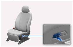
To set the desired position for the front passenger seat, adjust the seat to your preferred position and then quickly press the front portion of the relaxation switch three times consecutively.
