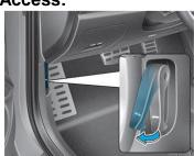
Pull the release lever to unlatch the hood. The hood should pop open slightly.
