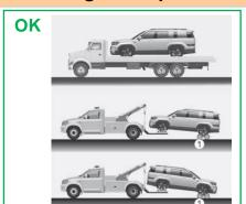
Notice: The use of wheel dollies (1) or flatbed is recommended. Use a wheel lift or flatbed equipment.
