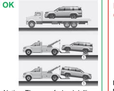
Notice: The use of wheel dollies (1) or flatbed is recommended. Use a wheel lift or flatbed equipment.
