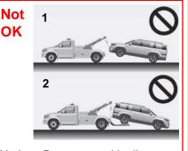
Notice : Do not tow with slingtype equipment (1). Do not tow the vehicle with the front wheels on the ground as this may cause damage to the vehicle (2).
