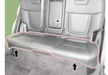
Remove the rear seat cushion assembly (A).
