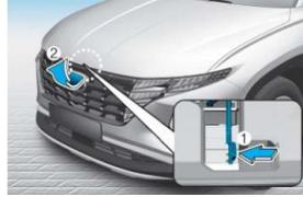
Raise the hood slightly, push the secondary latch up (①) inside of the hood center and lift the hood (②)
