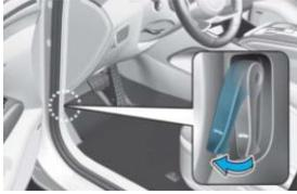
Pull the release lever to unlatch the hood. The hood should pop open slightly.
