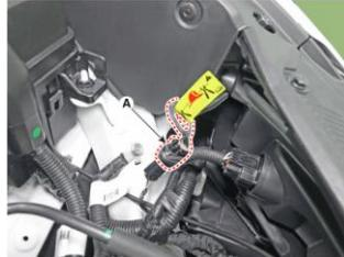
Disconnect the service interlock connector (A).
