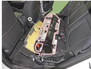
There is inlet/outlet duct and HEV battery system.
