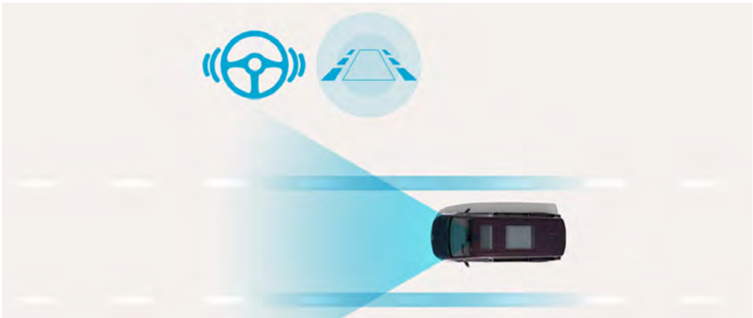
Lane Following Assist 2 (LFA 2). When activated, LFA2 provides slight steering inputs to keep the vehicle centred in its lane at speeds between 0 and 140 km per hour on highways and city streets. The front view camera recognizes lanes to help with steering. ♦
