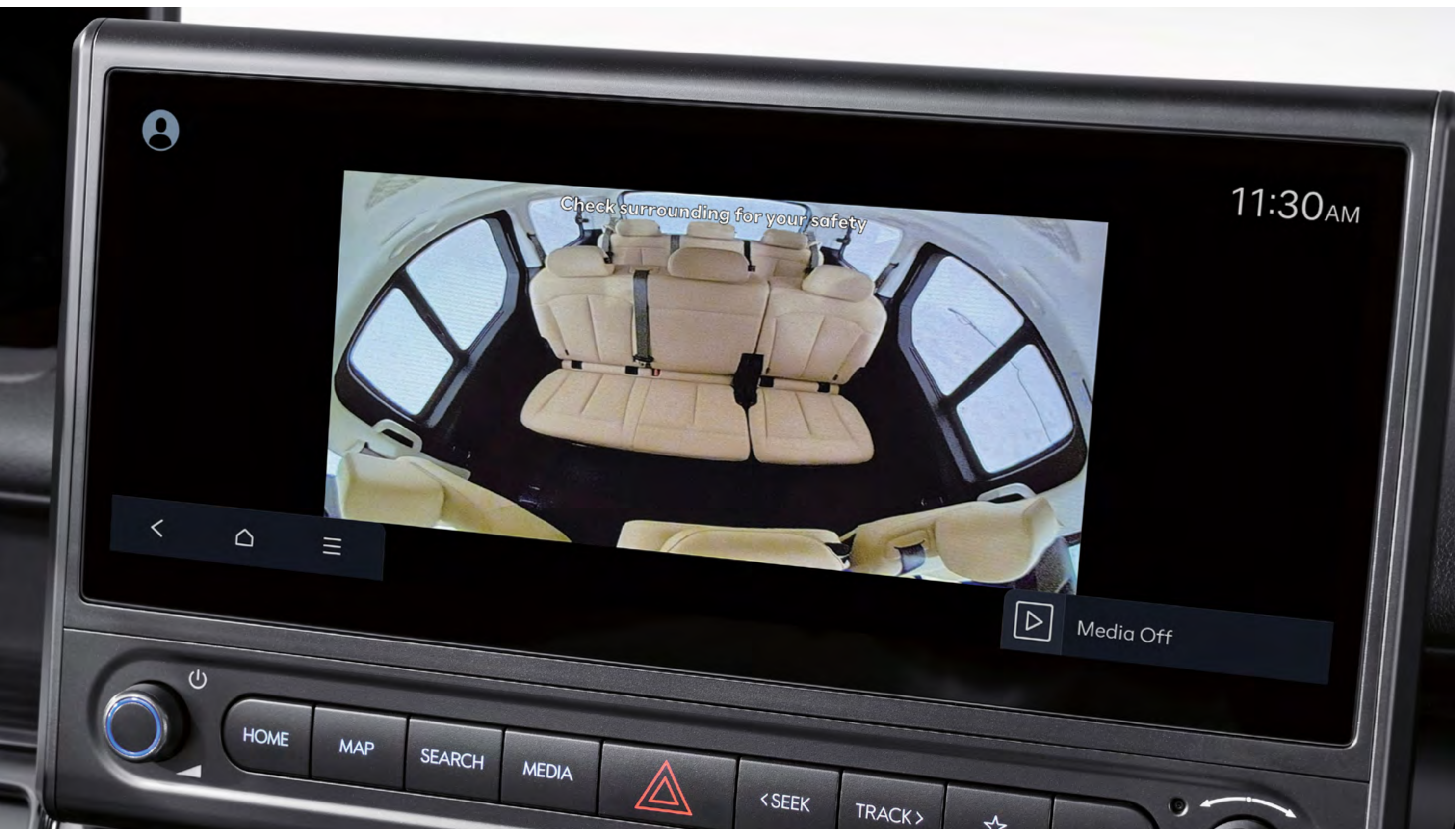
Passenger watch and talk, A camera brings rear passengers onto the centre screen while microphones and speakers support easy conversation.
