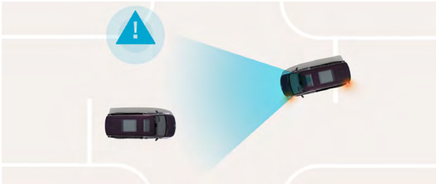
Forward Collision-avoidance Assist 1.5 with Junction Turning (FCA-JT). Automatically brakes when it detects sudden braking by the car ahead or detects pedestrians or cyclists in your path. During cross intersection turning, it brakes if there is a risk of collision with an oncoming vehicle. ♦
