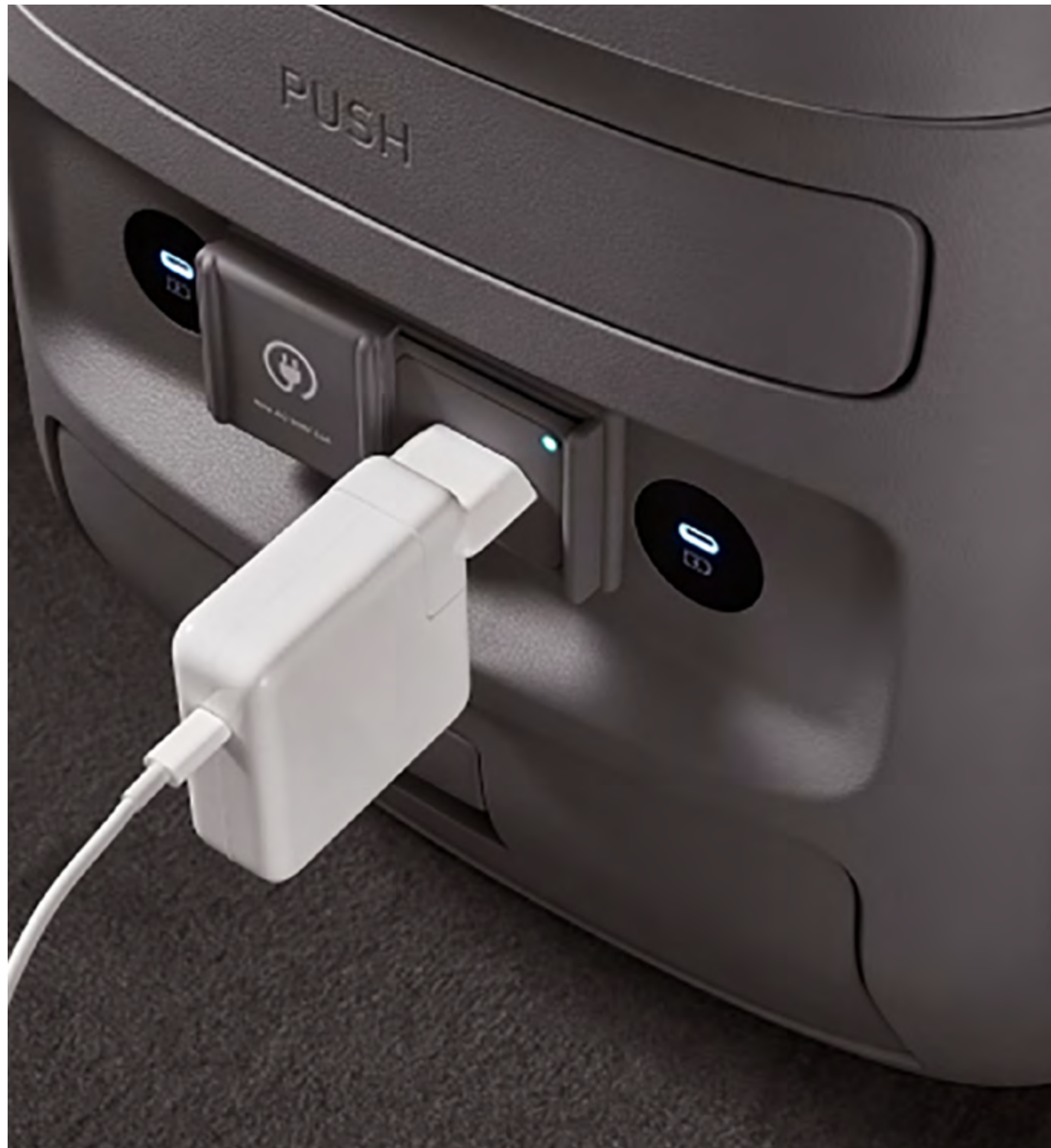
230V Vehicle-to-Load (V2L) socket in the centre console.
