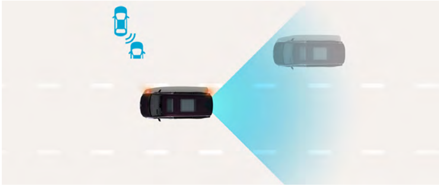
Blind Spot Collision-avoidance Assist (BCA). Using two radar sensors in the lower rear bumper, the system warns you of traffic in the blind spot area. Should you set the turn indicator in such a situation, it will sound an acoustic and visual alert. ♦
