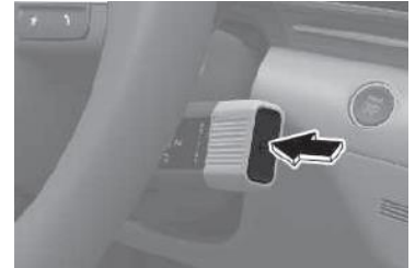
Put the vehicle in P (Park) position by pressing the 'P' button on the rotary shifter
