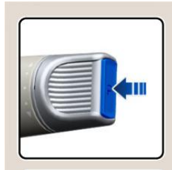
Put the vehicle in P (Park) position by pressing the 'P' button on the rotary shifter
