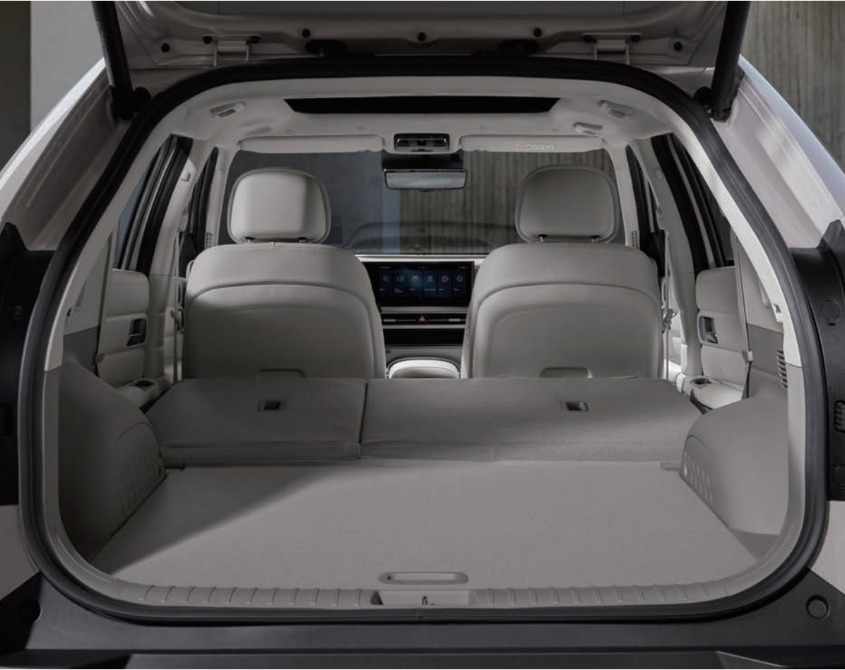
Cargo space: 510 L / max 1630 L with second-row seats folded flat. (VDA standard)
