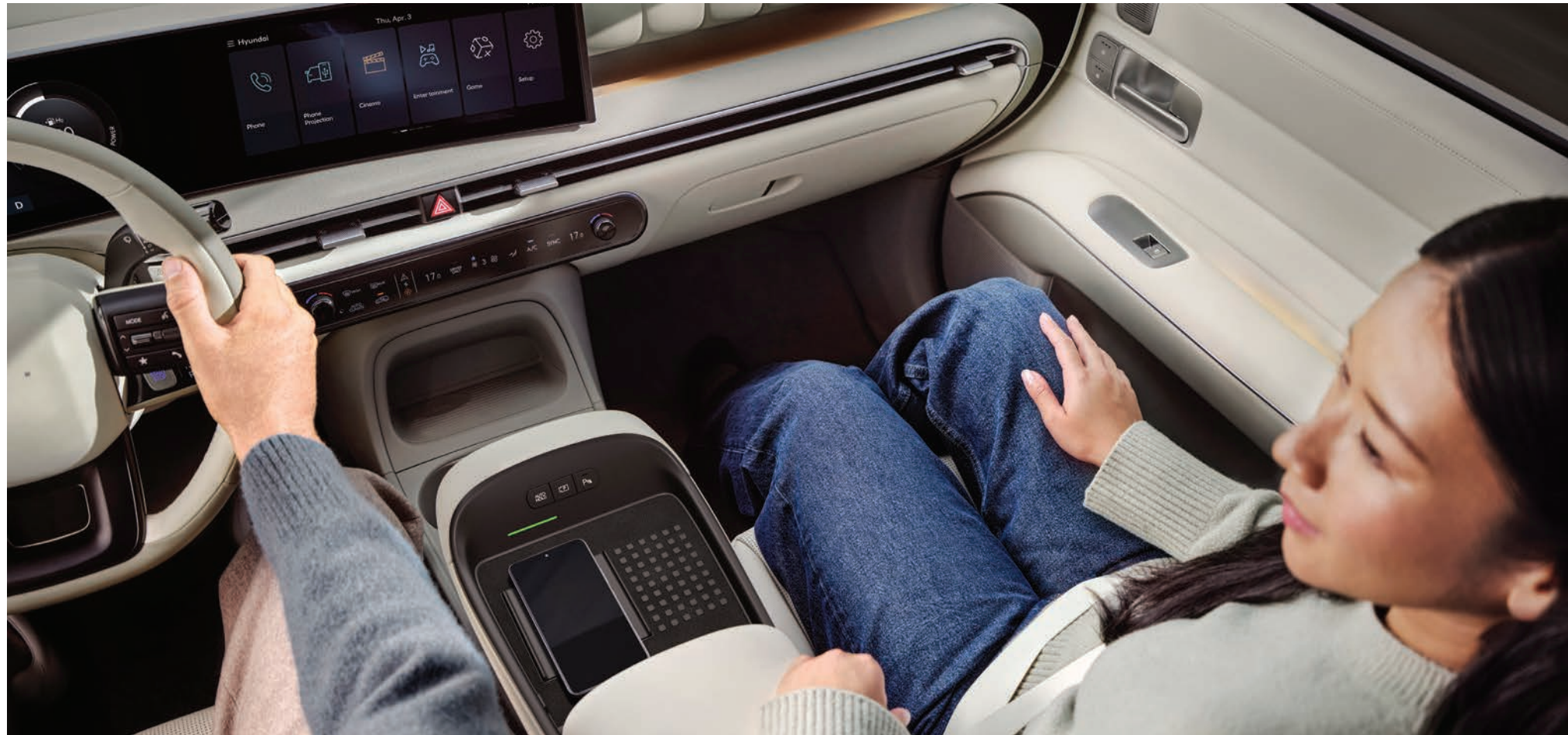
Located in the centre console, the wireless charging pad makes high-speed smartphone charging easy. The 15W system includes a cooling fan to prevent overheating. USB-C ports are also on board.
