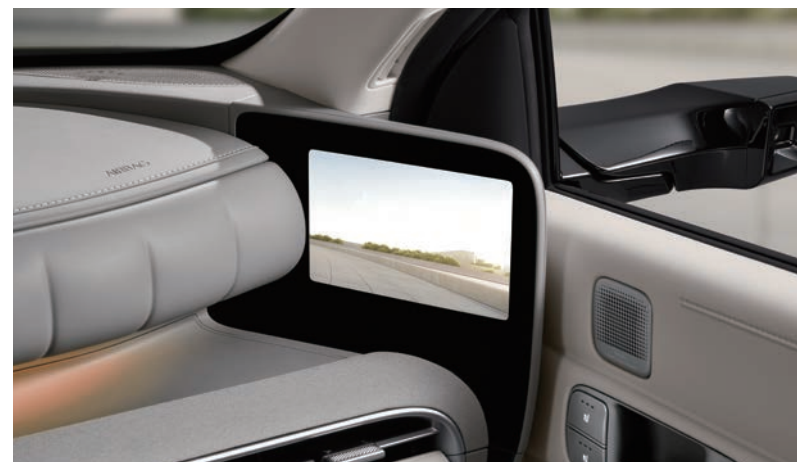
Digital Center Mirror (DCM). Digital Side Mirror (DSM).
