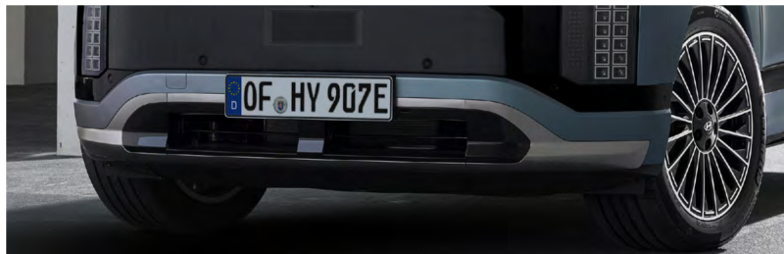
Dual-motion active air flap system for improved aerodynamics and a sleeker appearance.
