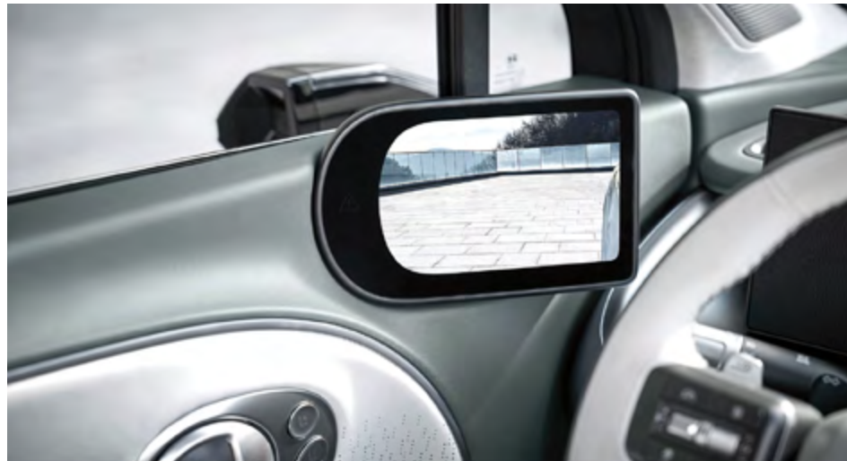
Door-mounted monitor of the Digital Side Mirror (DSM).
