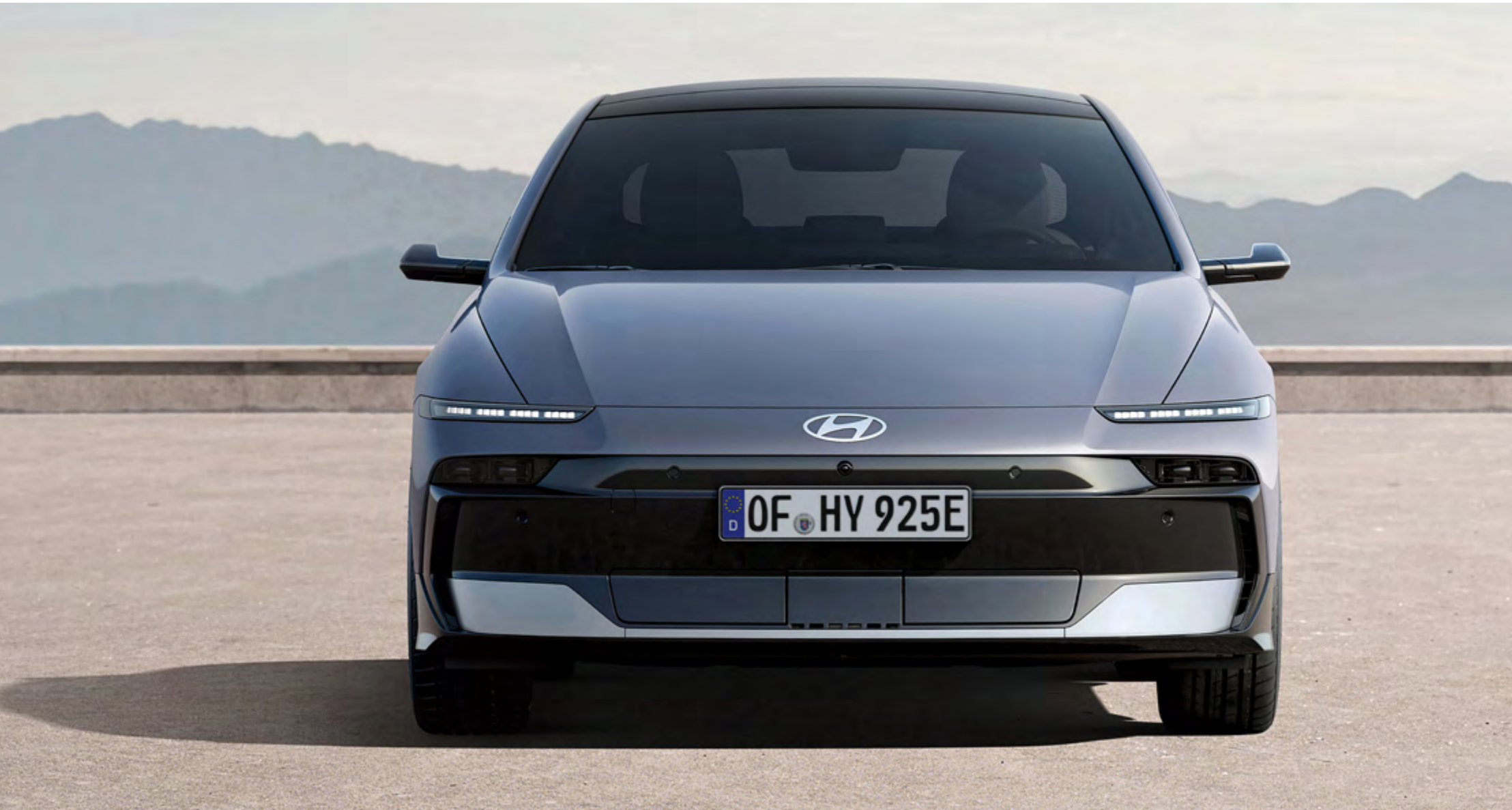
The new front bumper has been reshaped with sharp muscular lines and now holds the main Matrix LED headlamps.
