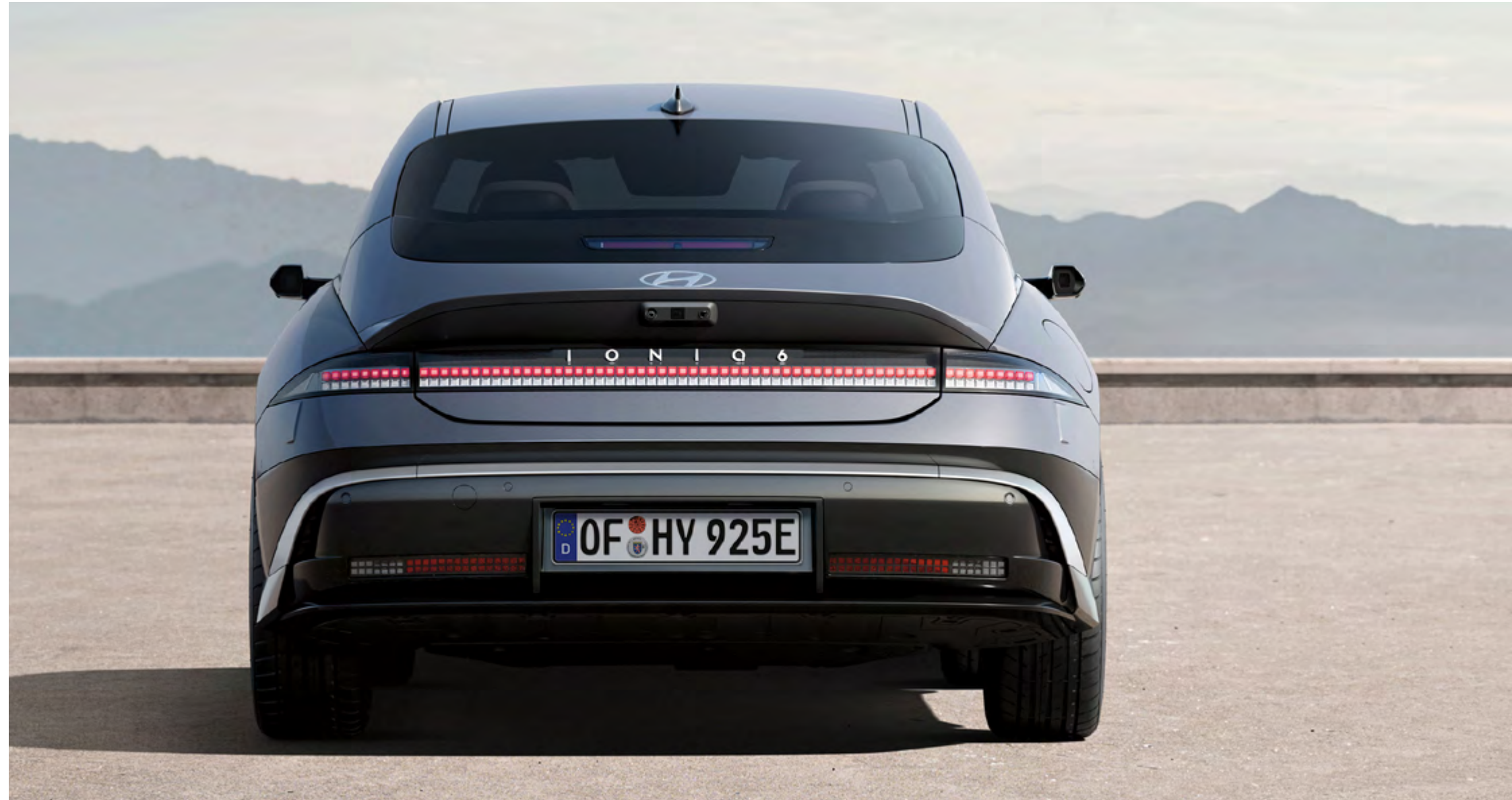
The rear bumper features bold horizontal design elements and signature IONIQ Parametric Pixels lighting connecting the combination LED lamps.
