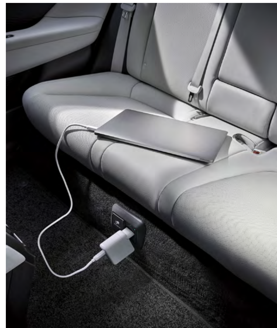
Interior 230V Vehicle-to-Load socket (V2L).
