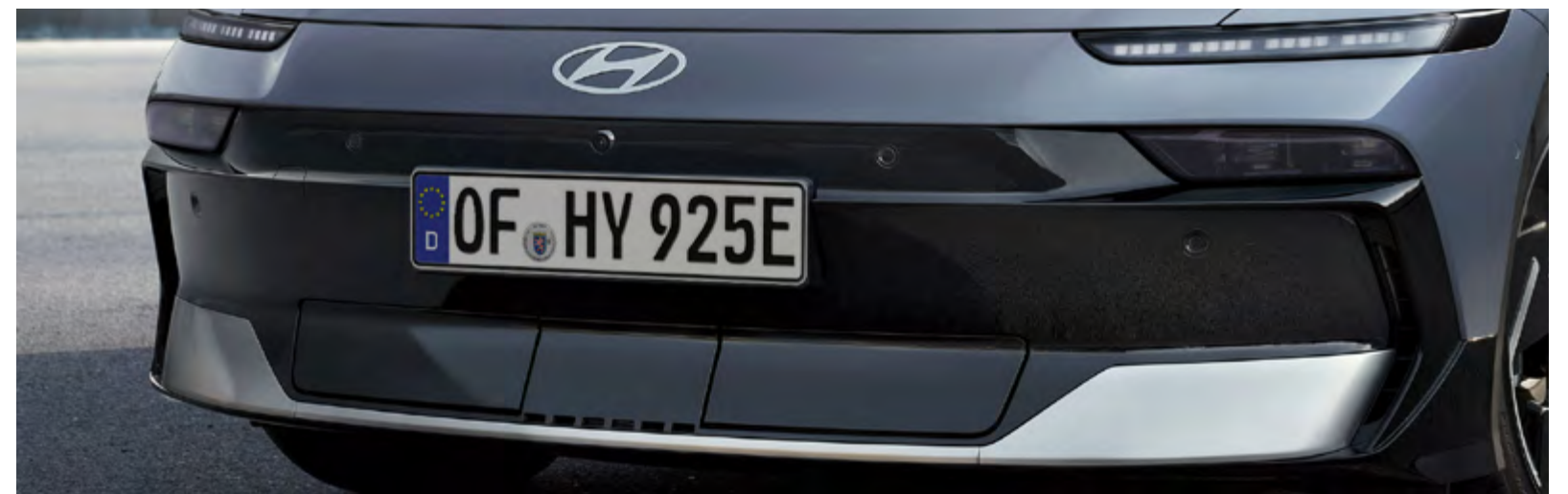
Active air flaps automatically open and close for maximum aerodynamic efficiency and battery cooling.
