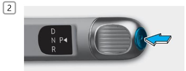
2. For automatic transmission vehicles, shift into park(P) gear.
