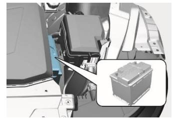
3. Battery in the engine compartment
