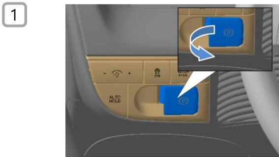
1. Chock the wheels and pull the switch to set the parking brake.
