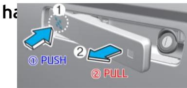
When the door outer handle doesn't pop-out, push the front side inwards.
