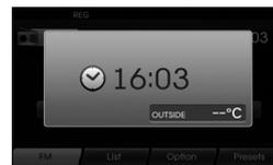
Press the time (🕒) on the control panel when the system is off.
